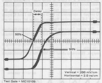
FIGURE 4 – MECL 10,000 Propagation Delay
