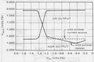
FIGURE 3 – Typical MECL 10,000 Transfer Characteristics
