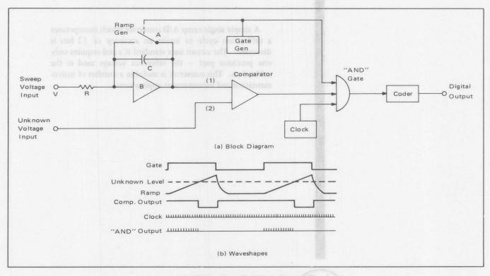
FIGURE 1 - Simplified Single Ramp A/D
