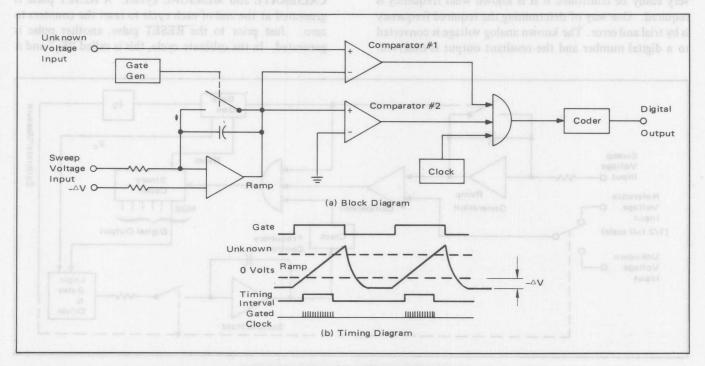
FIGURE 2 - Single Ramp Starting Below Zero
