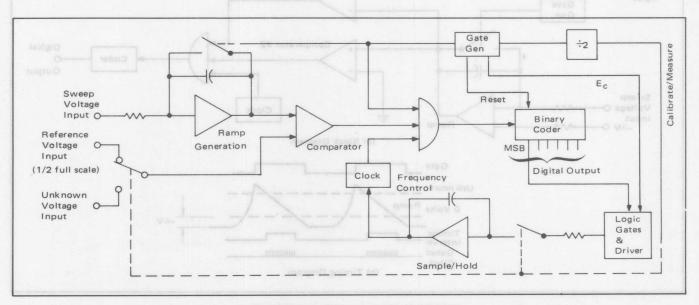
FIGURE 3 – Calibration Block Diagram
