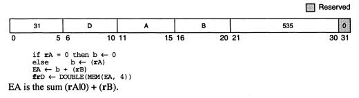
The word in memory addressed by EA is interpreted as a floating-point single-precision operand. This word is converted to floating-point double-precision (see Section D.6, "Floating-Point Load Instructions") and placed into **fr**D.
