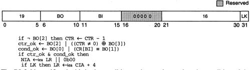
The BI field specifies the bit in the condition register to be used as the condition of the branch. The BO field is encoded as described in Table 8-8. Additional information about BO field encoding is provided in Section 4.2.4.2, "Conditional Branch Control."
