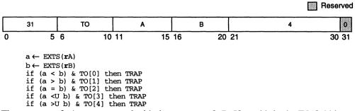
The contents of  $\mathbf{r}\mathbf{A}$  are compared with the contents of  $\mathbf{r}\mathbf{B}$ . If any bit in the TO field is set and its corresponding condition is met by the result of the comparison, then the system trap handler is invoked.
