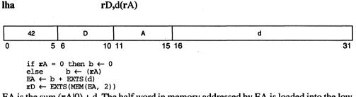
EA is the sum (rA|0) + d. The half word in memory addressed by EA is loaded into the loworder 16 bits of rD. The remaining bits in rD are filled with a copy of the most-significant bit of the loaded half word.
