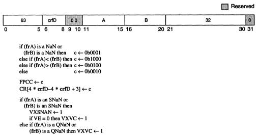
The floating-point operand in **fr**A is compared to the floating-point operand in **fr**B. The result of the compare is placed into CR field **crfD** and the FPCC.
