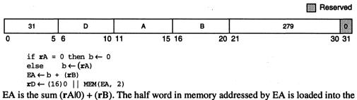
EA is the sum (rA|0) + (rB). The half word in memory addressed by EA is loaded into the low-order 16 bits of rD. The remaining bits in rD are cleared.
