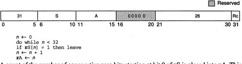
A count of the number of consecutive zero bits starting at bit 0 of rS is placed into rA. This number ranges from 0 to 32, inclusive.
