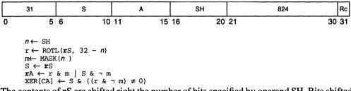
The contents of rS are shifted right the number of bits specified by operand SH. Bits shifted out of position 31 are lost. The shifted value is sign-extended before being placed in rA. The 32-bit result is placed into rA. XER[CA] is set if rS contains a negative number and any 1 bits are shifted out of position 31; otherwise XER[CA] is cleared. A shift amount of zero causes XER[CA] to be cleared.
