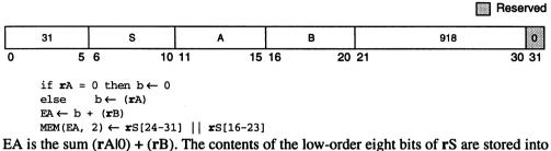
EA is the sum (rAl0) + (rB). The contents of the low-order eight bits of rS are stored into bits 0–7 of the half word in memory addressed by EA. The contents of the subsequent loworder eight bits of rS are stored into bits 8–15 of the half word in memory addressed by EA.
