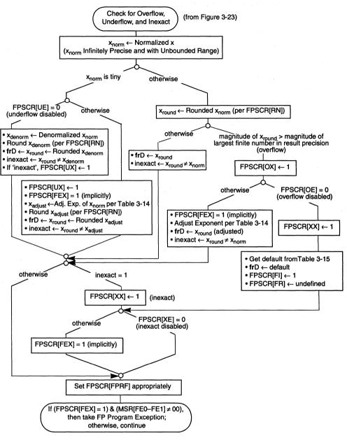
Figure 3-24. Checking of Remaining Floating-Point Exception Conditions
