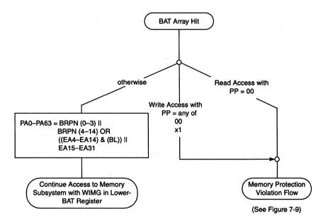
Figure 7-11. Block Address Translation Flow
