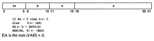
The contents of register frS are stored into the double word in memory addressed by EA.
