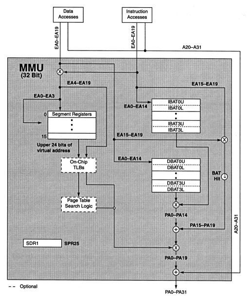
Figure 7-1. MMU Conceptual Block Diagram
