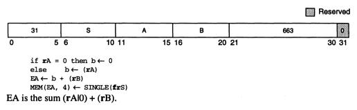
The contents of register **frS** are converted to single-precision and stored into the word in memory addressed by EA. For a discussion on floating-point store conversions, see Section D.7, "Floating-Point Store Instructions."
