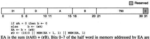
EA is the sum  $(\mathbf{r}A|0) + (\mathbf{r}B)$ . Bits 0–7 of the half word in memory addressed by EA are loaded into the low-order eight bits of  $\mathbf{r}D$ . Bits 8–15 of the half word in memory addressed by EA are loaded into the subsequent low-order eight bits of  $\mathbf{r}D$ . The remaining bits in  $\mathbf{r}D$ are cleared.
