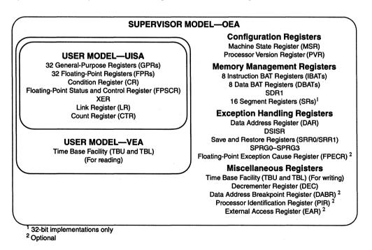
Figure 1-1. Programming Model—PowerPC Registers
