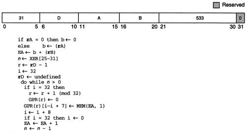
EA is the sum (rAl0) + (rB). Let n = XER[25-31]; *n* is the number of bytes to load. Let nr = CEIL(n + 4); *nr* is the number of registers to receive data. If n > 0, *n* consecutive bytes starting at EA are loaded into GPRs rD through rD + nr - 1.
