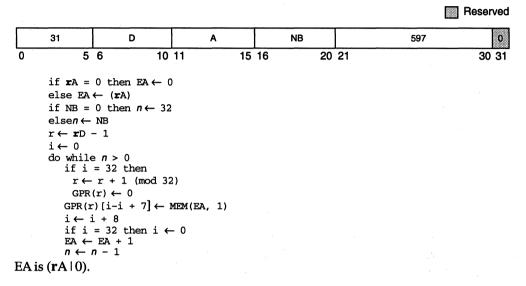
Let n = NB if  $\text{NB} \neq 0$ , n = 32 if NB = 0; *n* is the number of bytes to load. Let  $nr = \text{CEIL}(n \neq 4)$ ; *nr* is the number of registers to be loaded with data.
