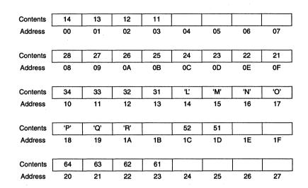
Figure 3-6. Munged Little-Endian Structure S as Seen by Processor
