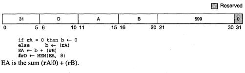
The double word in memory addressed by EA is placed into frD.
