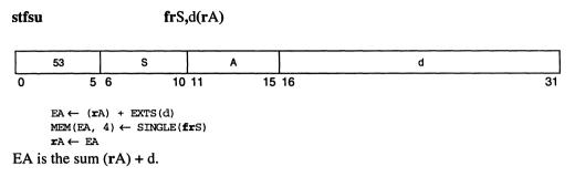
The contents of **fr**S are converted to single-precision and stored into the word in memory addressed by EA. Note that the value to be stored should be in single-precision format prior to the execution of the **stfsu** instruction. For a discussion on floating-point store conversions, see Section D.7, "Floating-Point Store Instructions."
