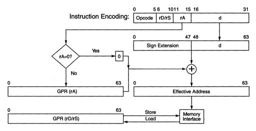
Figure 4-1. Register Indirect with Immediate Index Addressing for Integer Loads/Stores
