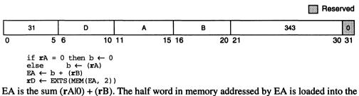
EA is the sum (rA|0) + (rB). The half word in memory addressed by EA is loaded into the low-order 16 bits of rD. The remaining bits in rD are filled with a copy of the most-significant bit of the loaded half word.
