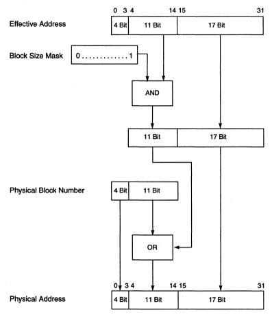
Figure 7-10. Block Physical Address Generation
