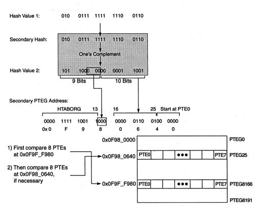
Figure 7-24. Example Secondary PTEG Address Generation
