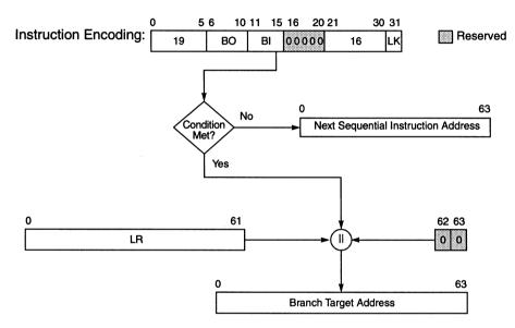
Figure 4-10. Branch Conditional to Link Register Addressing
