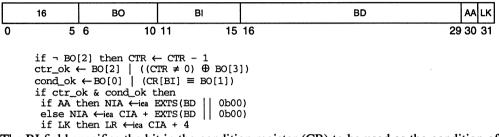
The BI field specifies the bit in the condition register (CR) to be used as the condition of the branch. The BO field is encoded as described in Table 8-6. Additional information about BO field encoding is provided in Section 4.2.4.2, "Conditional Branch Control."
