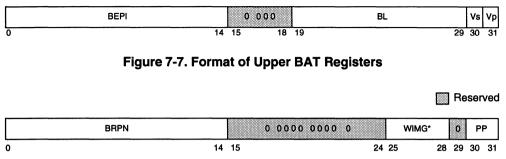
\*W and G bits are not defined for IBAT registers. Attempting to write to these bits causes boundedly-undefined results.
