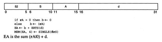
The contents of register frS are converted to single-precision and stored into the word in memory addressed by EA. Note that the value to be stored should be in single-precision format prior to the execution of the stfs instruction. For a discussion on floating-point store conversions, see Section D.7, "Floating-Point Store Instructions."
