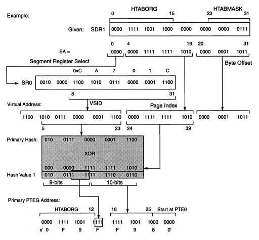
Figure 7-23. Example Primary PTEG Address Generation
