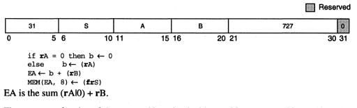
The contents of register frS are stored into the double word in memory addressed by EA.
