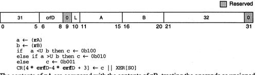
The contents of  $\mathbf{r}A$  are compared with the contents of  $\mathbf{r}B$ , treating the operands as unsigned integers. The result of the comparison is placed into CR field **crf**D.
