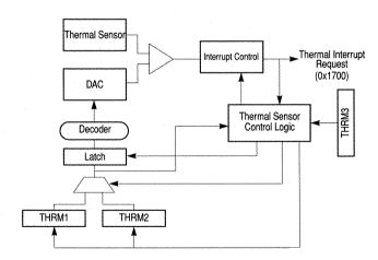
Figure 10-1. Thermal Assist Unit Block Diagram
