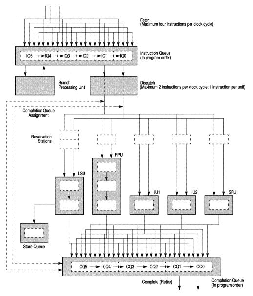
Figure 6-4. Instruction Flow Diagram
