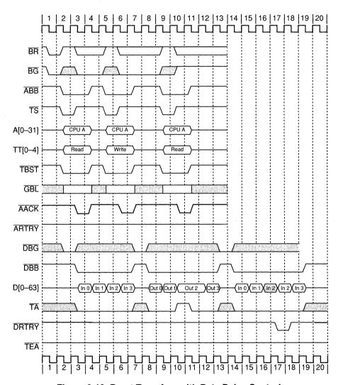
Figure 8-19. Burst Transfers with Data Delay Controls
