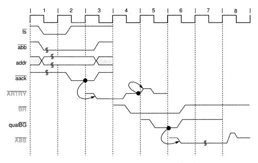
Figure 8-7. Snooped Address Cycle with ARTRY
