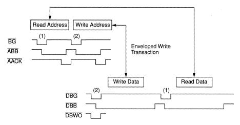
Figure 8-22. Data Bus Write Only Transaction
