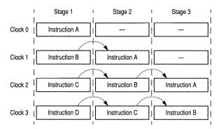
Figure 6-1. Pipelined Execution Unit
