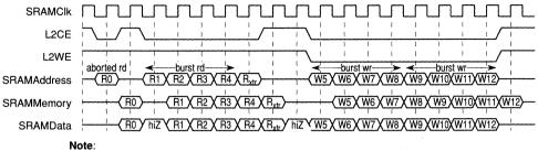
R<sub>xtr</sub> indicates where an extra read cycle is signaled to keep the burst RAM driving the data bus for the last read.
