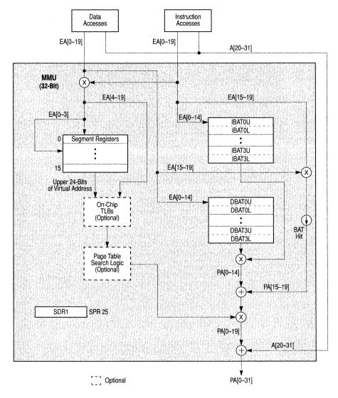
Figure 5-1. MMU Conceptual Block Diagram—32-Bit Implementations
