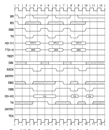
Figure 8-18. Single-Beat Writes Showing Data Delay Controls
