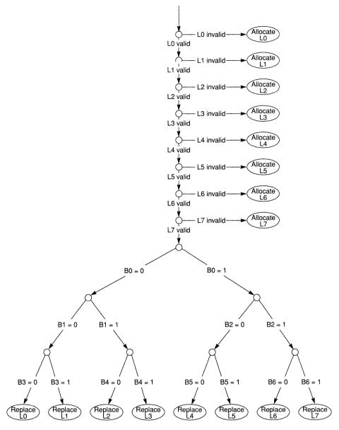
Figure 3-5. PLRU Replacement Algorithm
