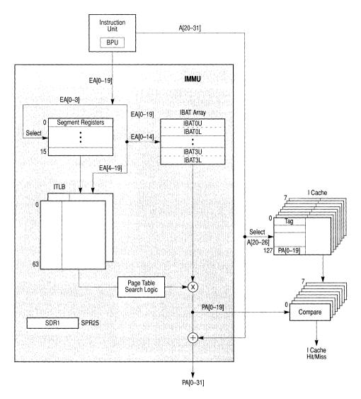
Figure 5-2. MPC750 Microprocessor IMMU Block Diagram
