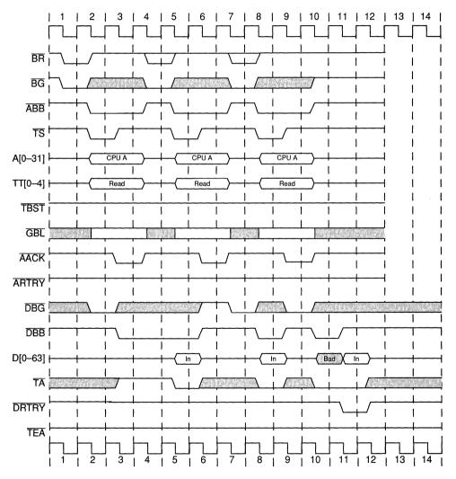
Figure 8-17. Single-Beat Reads Showing Data-Delay Controls
