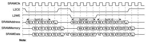
$R_{\text{xtr}}$  indicates where an extra read cycle is signaled to keep the burst RAM driving the data bus for the last read.
