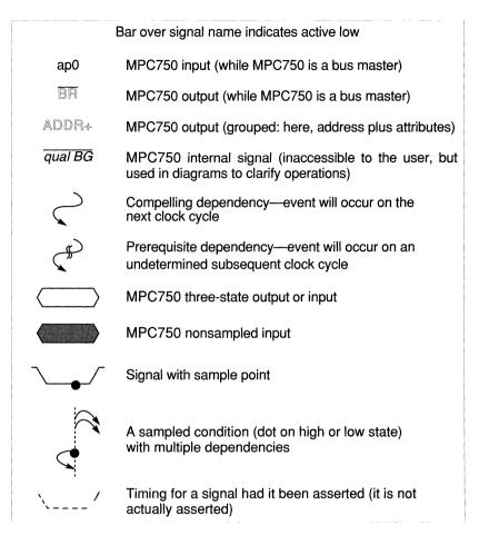
Figure 8-2. Timing Diagram Legend
