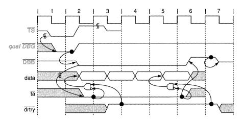
Figure 8-11. Normal Burst Transaction
