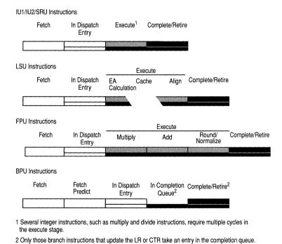
Figure 6-3. MPC750 Microprocessor Pipeline Stages
