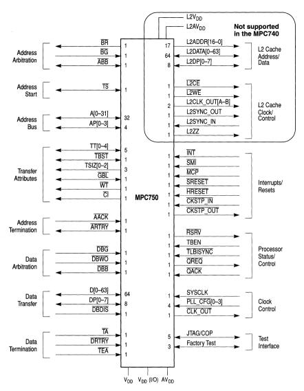
Figure 1-4. MPC750 Microprocessor Signal Groups
