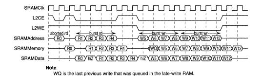
Figure 9-10. Burst Read-Write-Write L2 Cache Access (Late-Write SRAM)
