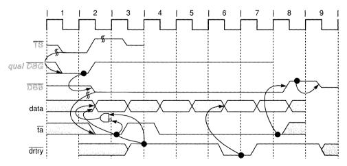
Figure 8-13. Read Burst with TA Wait States and DRTRY
