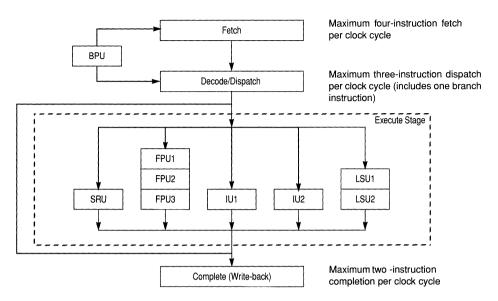
Figure 6-2. Superscalar/Pipeline Diagram
