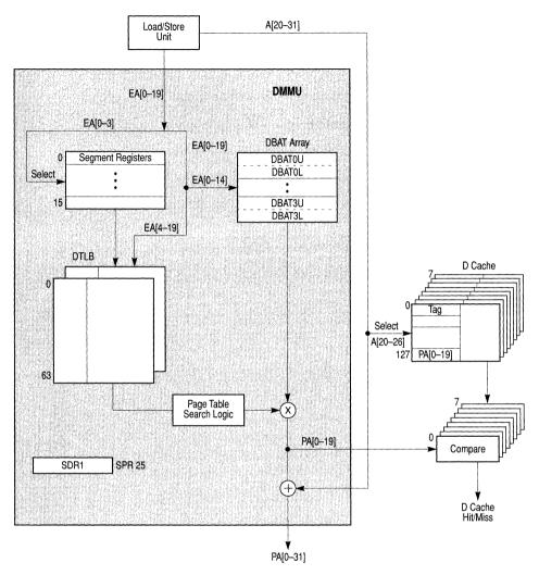
Figure 5-3. MPC750 Microprocessor DMMU Block Diagram
