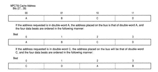
Figure 3-6. Double-Word Address Ordering—Critical Double Word First
