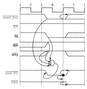
Figure 8-5. Address Bus Arbitration Showing Bus Parking
