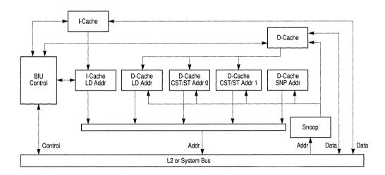
Figure 3-7. Bus Interface Address Buffers
