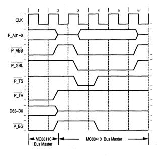
Figure 4-13. Primary Cache Invalidate Timing
