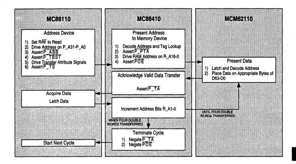
Figure 4-15. Burst Read Transaction Flow
