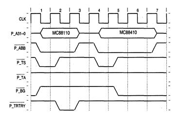
Figure 4-21. Retry of a Processor Transaction
