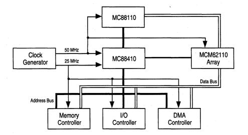
Figure 5-1. Half-Speed System Interface
