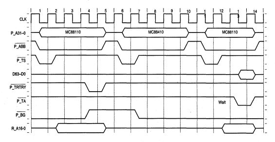
Figure 4-22. Retry Caused By Replacement Copyback
