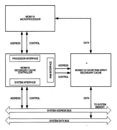
Figure 1-1. MC88110/MC88410 System Configuration
