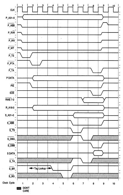
Figure 5-11. Full-Speed Single-Beat Write-Through Timing
