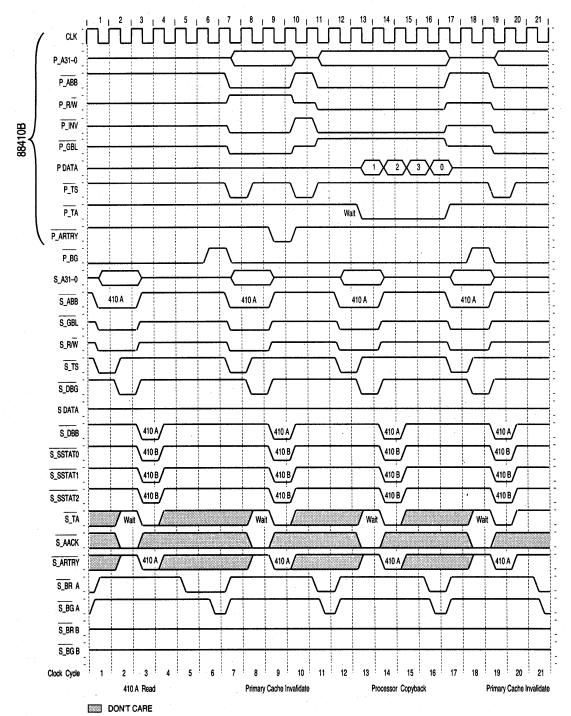
Figure 5-41a. Full-Speed Snoop Hit with Processor Copyback (Split Bus)
