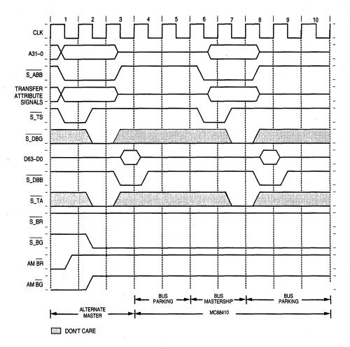
Figure 5-5. Bus Parking: Full-Speed Mode
