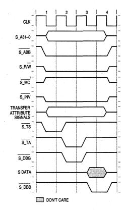
Figure 5-12. Full-Speed System Invalidate Transaction
