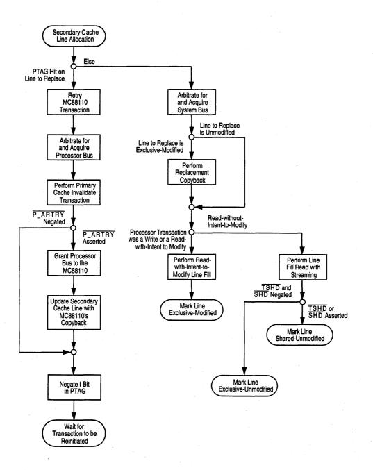
Figure 2-15. Secondary Cache Line Allocation Flow
