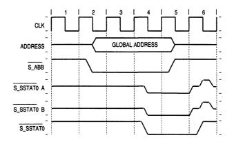
Figure 5-32. Snoop Status Negation Timing
