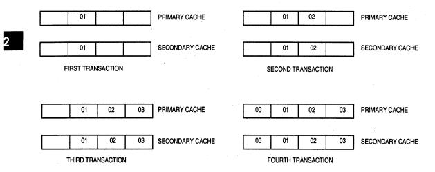
Figure 2-11. Streaming with 32-Byte Secondary Cache Line and Critical-Word-First
