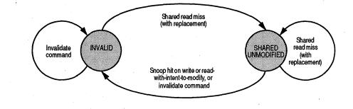
Figure 2-9. Secondary Cache States in Write-Through Mode
