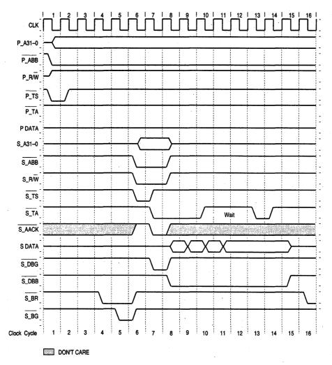
Figure 5-19. Full-Speed Burst Write with Wait Cycles
