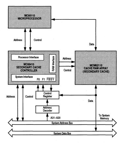
Figure 2-19. Flush Control Hardware
