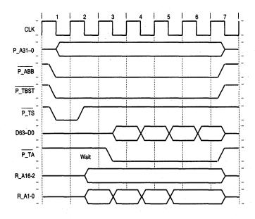
Figure 4-14. Burst Transaction - Fastest Case
