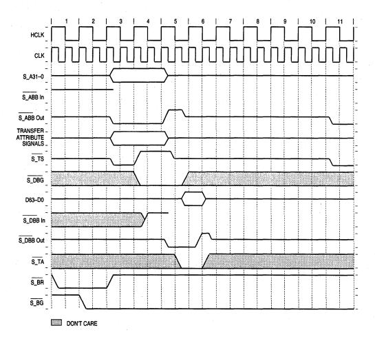
Figure 5-3. Half-Speed System Bus Arbitration Timing Example
