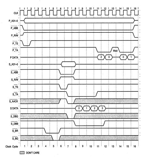
Figure 5-20. Streaming — 32 Byte Cache Line Size with Zero-Word-First
