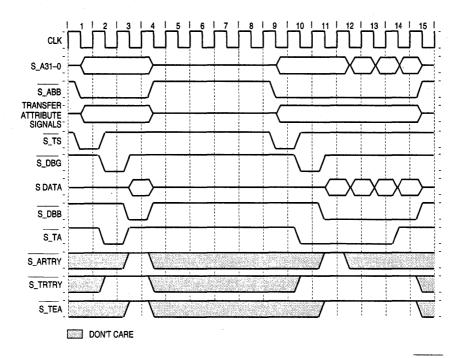
Figure 5-24. Full-Speed Normal Transaction Terminations with S\_TA
