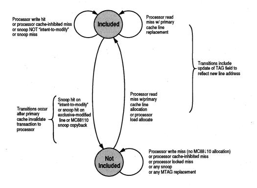
Included state —Corresponding secondary and primary cache lines are valid. Not Included state —Corresponding primary cache line is invalid. Corresponding secondary cache line may or may not be valid.
