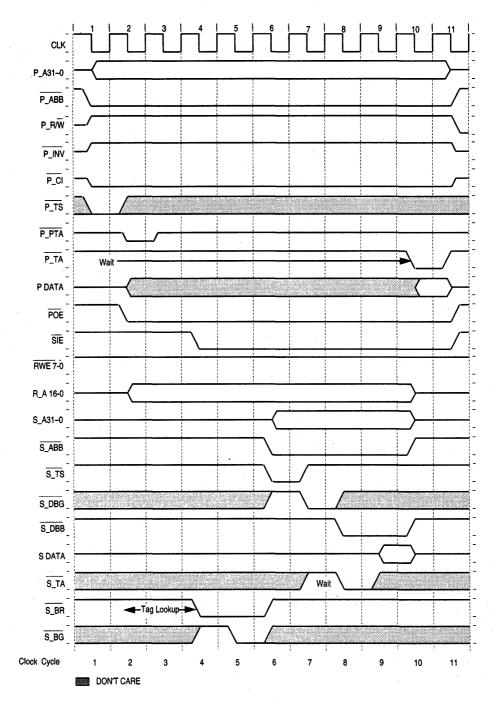
Figure 5-9. Full-Speed Single-Beat Cache-Inhibited Read
