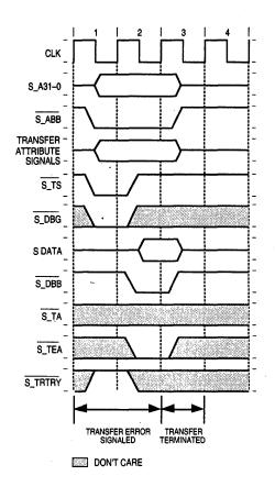
Figure 5-28. Transfer Error Termination
