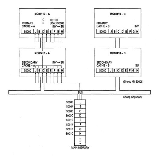
Figure 2-29. Completion of MC88110 – A Load, Cache Miss
