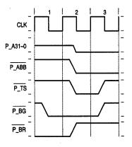
Figure 4-7. External Arbitration Timing
