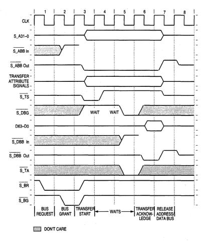
Figure 5-4. Full-Speed Data Bus Arbitration Timing Example
