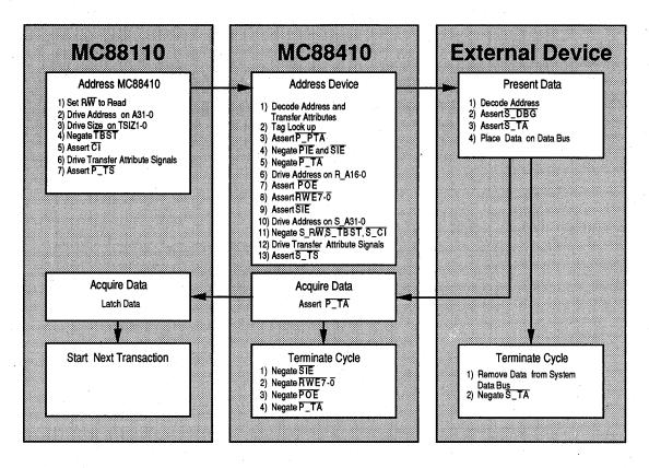
Figure 5-8. Full-Speed Single Beat Read Transaction Flow
