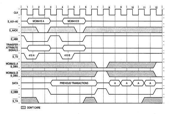
Figure 5-7. Full-Speed Multi-Level System Bus Arbitration
