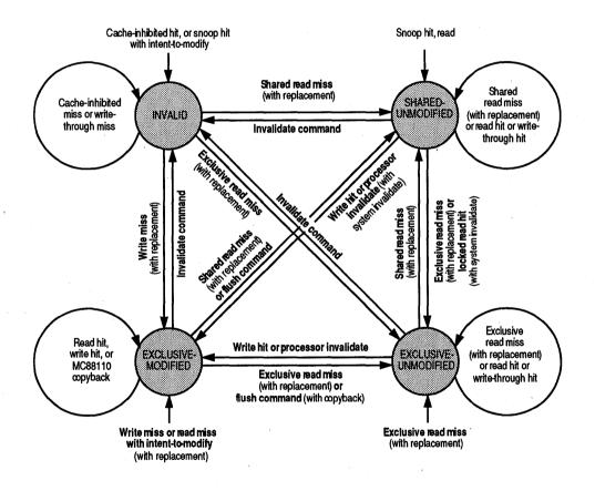
Figure 2-8. Secondary Cache States in Write-Back Mode
