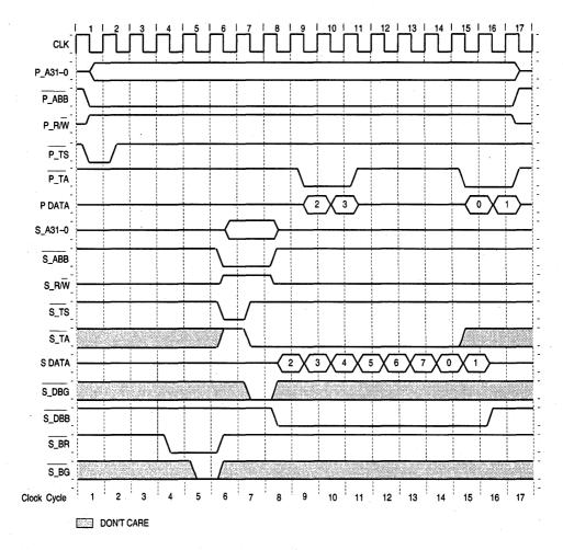
Figure 5-21. Streaming — 64 Byte Cache Line Size with Critical-Word-First
