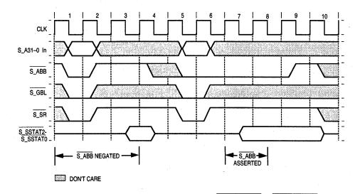
Figure 5-31. Snoop Hit/Miss Indication (S\_SSTAT2 - S\_SSTAT0)
