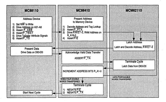
Figure 4-17. Burst Write Transaction Flow
