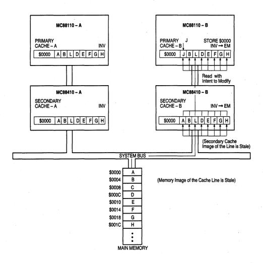
Figure 2-41. Completion of MC88110–A Load, Cache Miss
