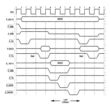
Figure 5-43. Lock Collision
