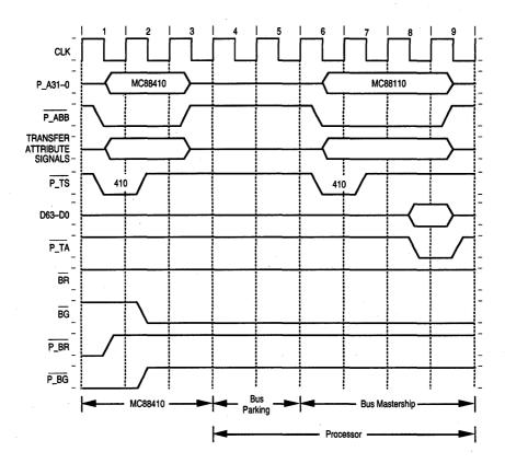
Figure 4-4. Bus Parking by External Arbiter
