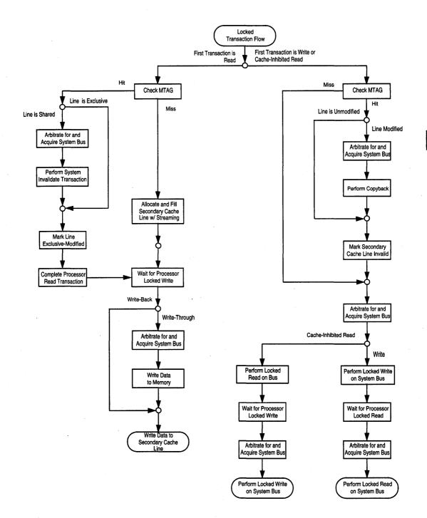
Figure 2-18. Locked Transaction Flow
