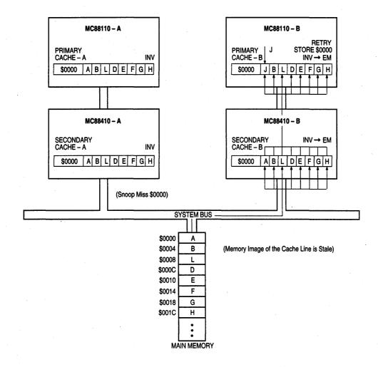
Figure 2-47. Completion of MC88110–A Load, Cache Miss
