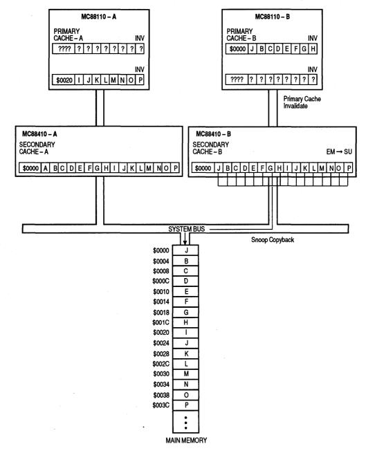
Figure 2-35. MC88110–A Snoop Copyback
