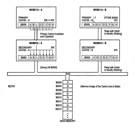
Figure 2-45. MC88410-B Read-with-Intent-to-Modify, Retried
