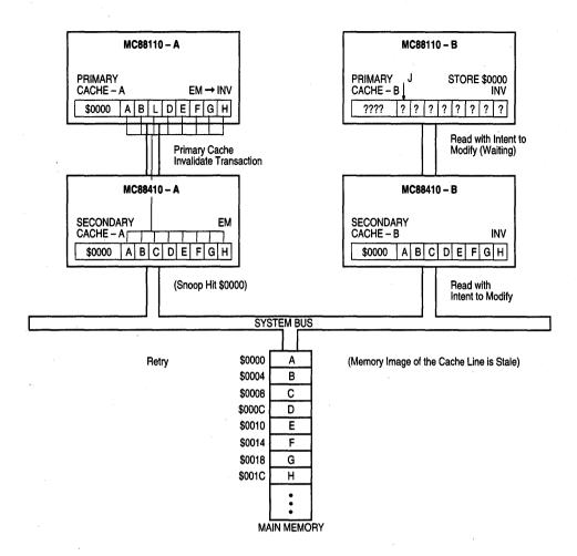
Figure 2-39. MC88410-B Read-with-Intent-to-Modify, Retried
