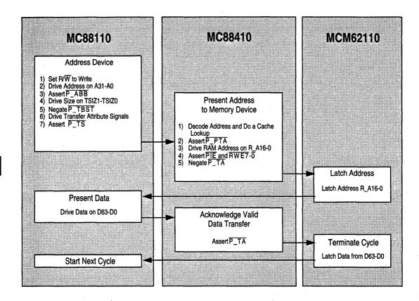
Figure 4-11. Single-Beat Write Transaction Flow
