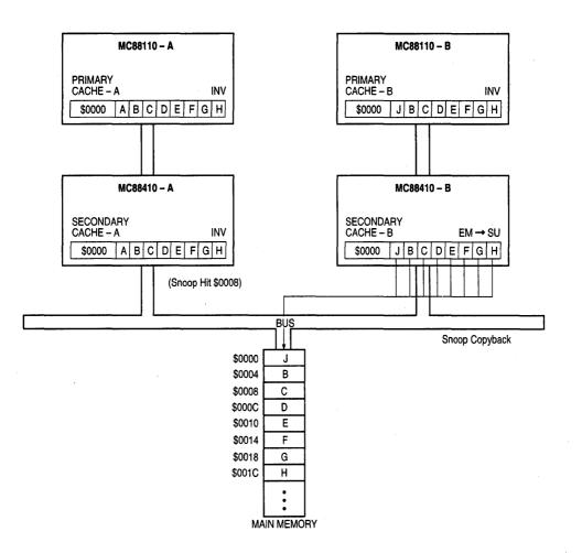
Figure 2-28. MC88110 – B Snoop Copyback
