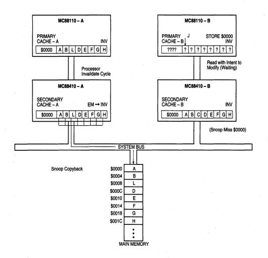
Figure 2-40. MC88410–A Snoop Copyback
