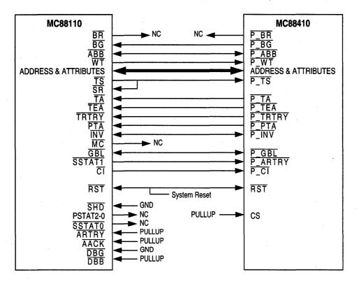
Figure 4-2. Single-MC88410 Configuration
