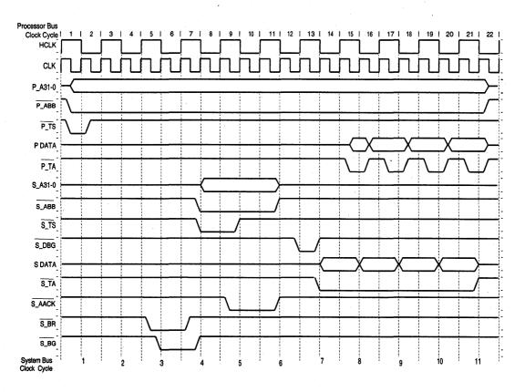
Figure 5-17. Half-Speed Streaming Line Fill
