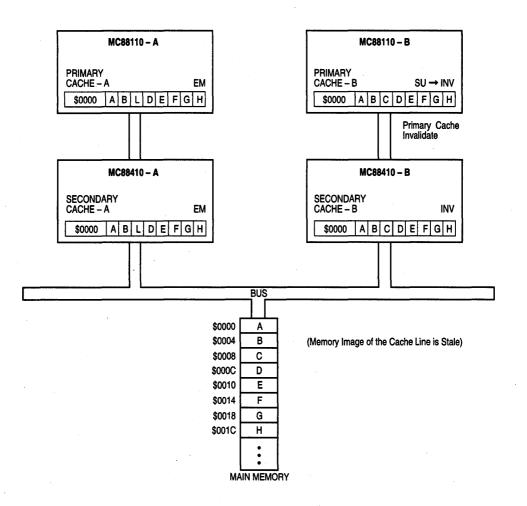
Figure 2-44. MC88410–B Processor Invalidate Transaction
