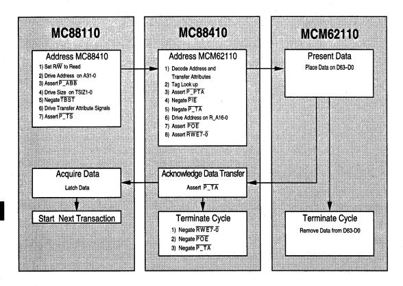
Figure 4-9. Single Beat Read Transaction Flow – Secondary Cache Hit
