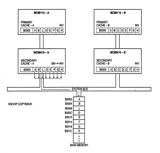
Figure 2-46. MC88410-A Snoop Copyback
