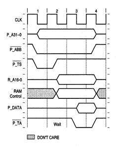
Figure 4-8. Single-Beat Transaction – Fastest Case
