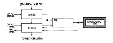
Figure 6-7. Bidirectional Cell Arrangement
