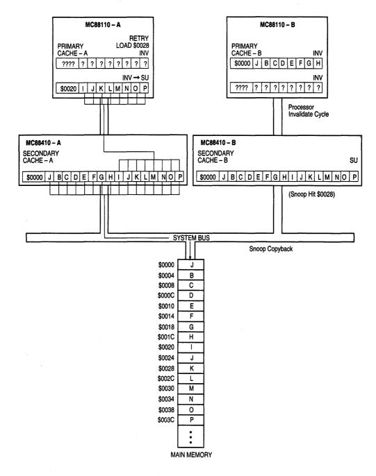
Figure 2-36. Completion of MC88110-A Load, Cache Miss
