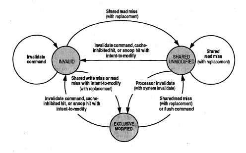
Figure 2-10. Secondary Cache States with Three-State Model
