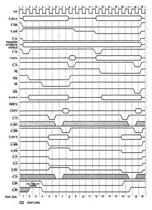
Figure 5-13. Cache-Inhibited Load-Store Locked Transaction
