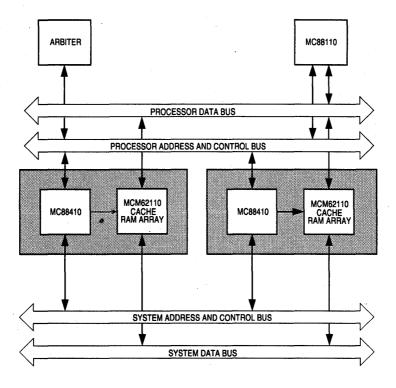
Figure 1-2. System with Two MC88410s
