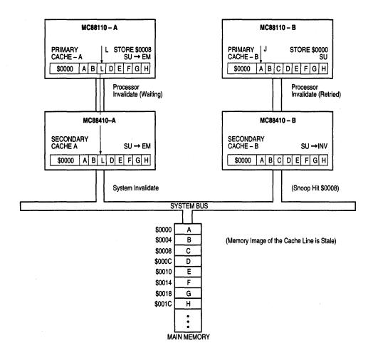
Figure 2-43. Simultaneous MC88110 Stores, Data Cache Miss, MC88410–A System Invalidate
