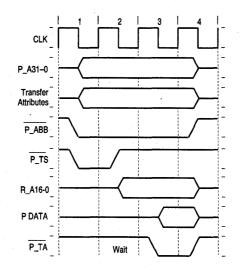
Figure 4-19. Normal Termination with P\_TA
