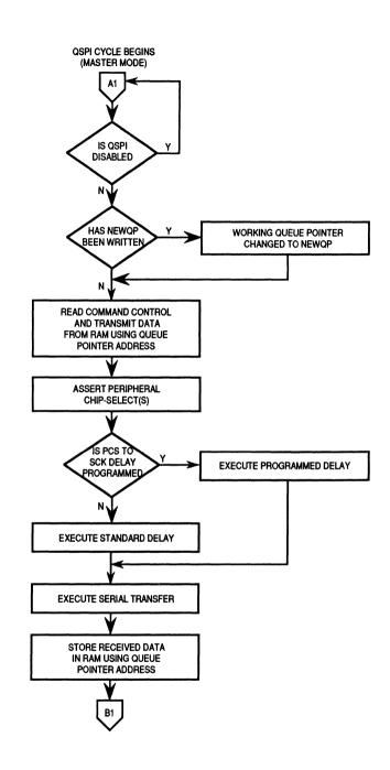
Figure 7-5. Flowchart of QSPI Master Operation (Part 1)
