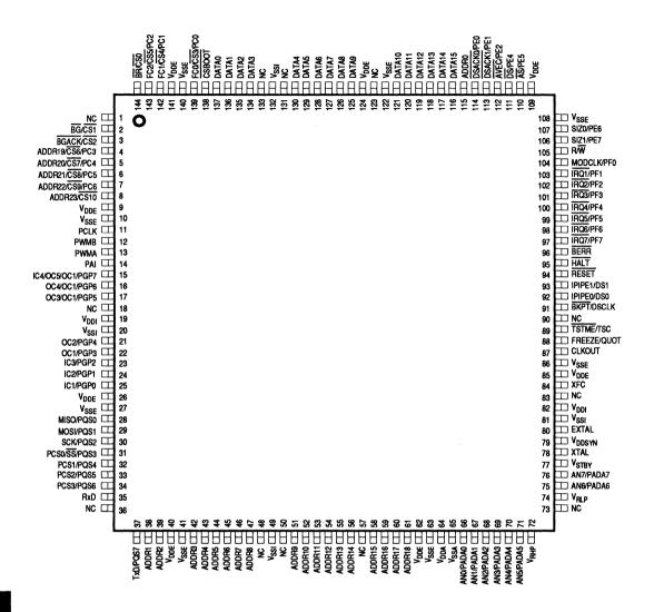
Figure B-4. 144-Pin Plastic Surface Mount Package Pin Assignments
