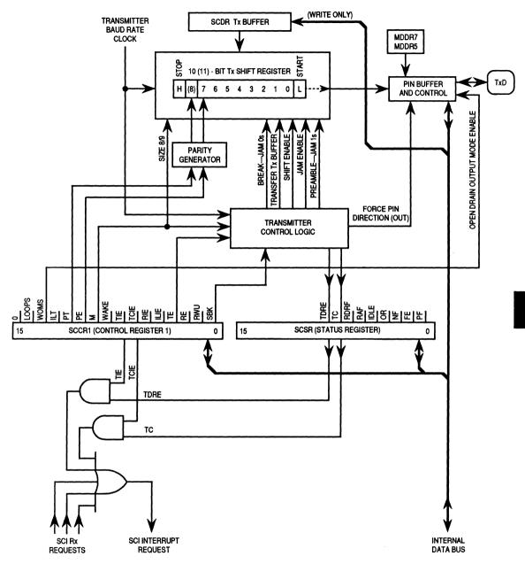
Figure 7-7. SCI Transmitter Block Diagram
