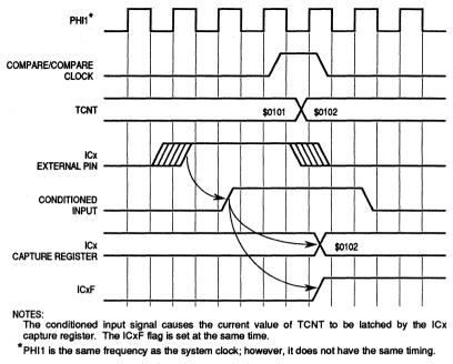
Figure 8–4. Input Capture Timing Example
