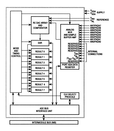
Figure 6-1. ADC Block Diagram
