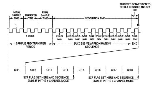
Figure 6-3. 10-Bit Conversion Timing
