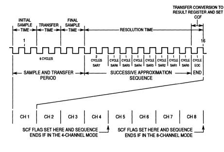
Figure 6-2. 8-Bit Conversion Timing
