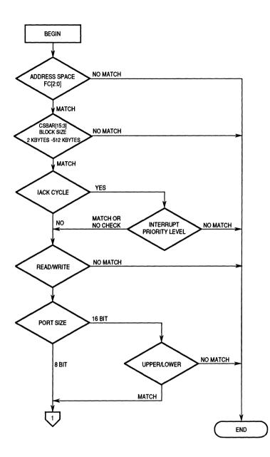
Figure 4-35. Flow Diagram for Chip Select (Sheet 1 of 3)
