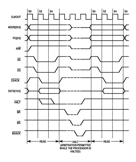
Figure 4–25. HALT Timing
