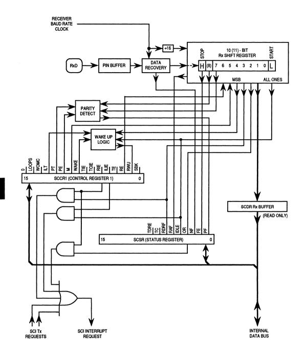
Figure 7-8. SCI Receiver Block Diagram
