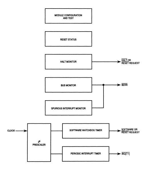
Figure 4-2. System Configuration and Protection
