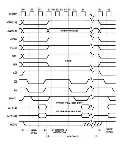
Figure 4-31. Interrupt Acknowledge Cycle Timing
