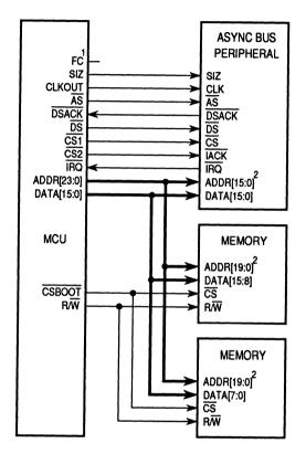
1. CAN BE DECODED TO PROVIDE ADDITIONAL ADDRESS SPACE. 2. VARIES DEPENDING UPON PERIPHERAL MEMORY SIZE.
