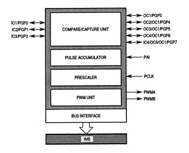
Figure 8–1. GPT Block Diagram
