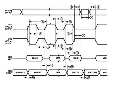
Figure A-17. QSPI Timing Master, CPHA = 1 APPENDIX A ELECTRICAL CHARACTERISTICS
