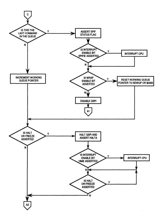
Figure 7-6. Flowchart of QSPI Slave Operation (Part 2)
