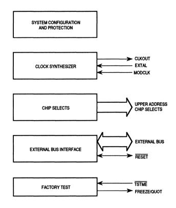
Figure 4–1. System Integration Module Block Diagram
