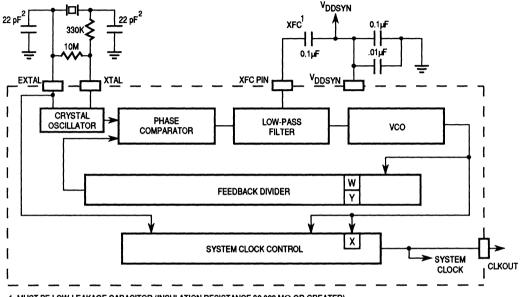
1. MUST BE LOW-LEAKAGE CAPACITOR (INSULATION RESISTANCE 30,000 M $\Omega$  OR GREATER). 2. CAPACITANCE BASED ON A TEST CIRCUIT CONSTRUCTED WITH A DAISHINKU DMX-38 32,768 kHz CRYSTAL.
