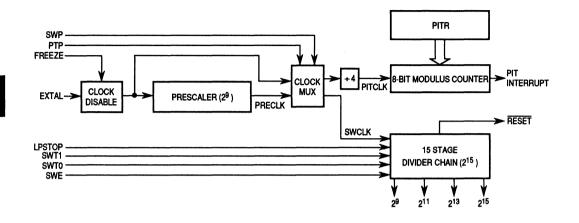
Figure 4–3. Periodic Interrupt Timer and Software Watchdog Timer
