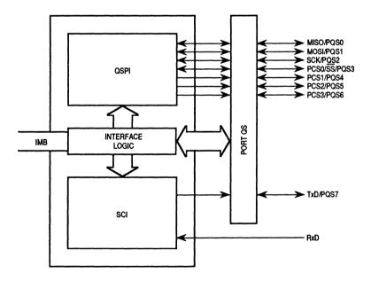
Figure 7-1. QSM Block Diagram
