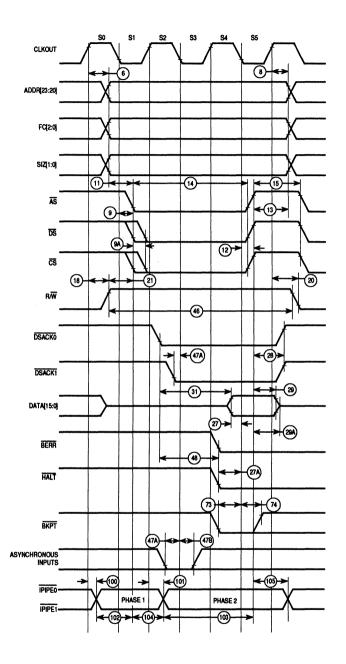
Figure A-4. Read Cycle Timing Diagram
