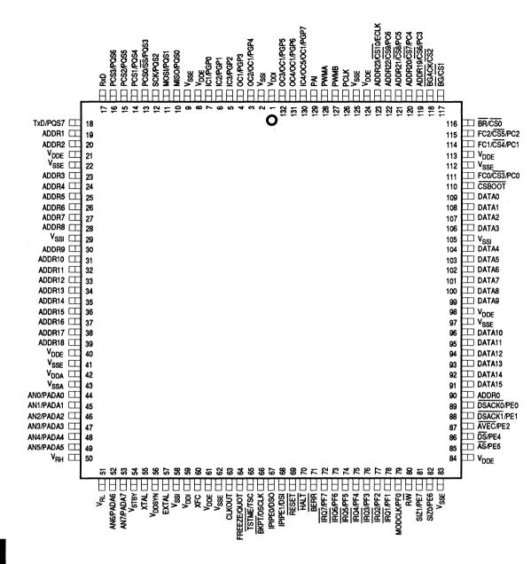
Figure B–1. 132-Pin Plastic Surface Mount Package Pin Assignments
