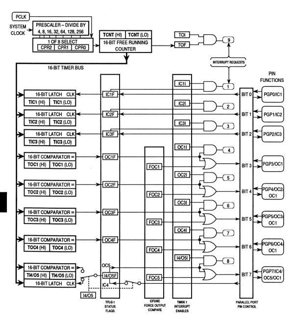
Figure 8–3. Capture/Compare Block Unit Diagram
