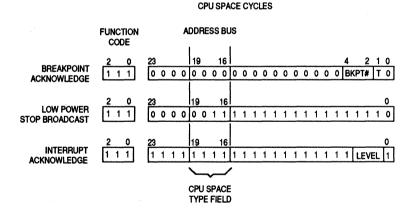
Figure 4-21. CPU Space Address Encoding
