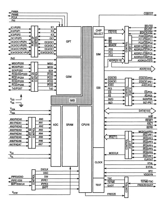
Figure 3-1. MC68HC16Z1 Block Diagram
