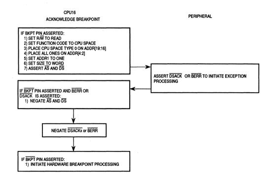
Figure 4-22. Breakpoint Operation Flow
