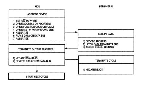
Figure 4–19. Write Cycle Flowchart
