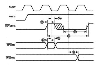
Figure A-14. Background Debugging Mode Timing Diagram — Serial Communication
