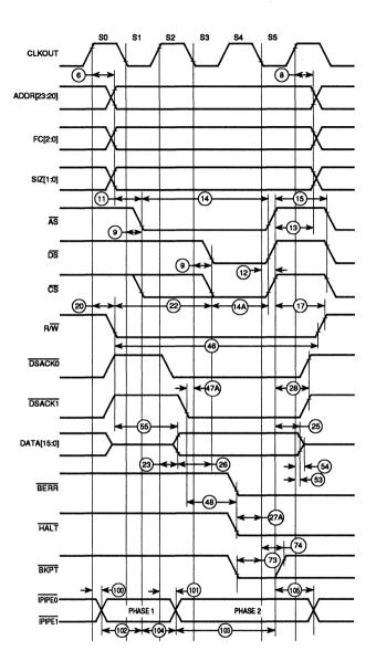
Figure A-5. Write Cycle Timing Diagram
