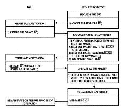
Figure 4-26. Bus Arbitration Flowchart for Single Request
