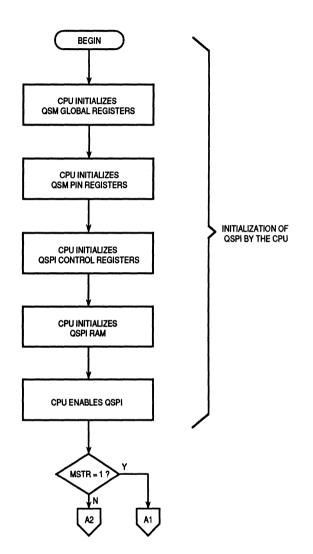
Figure 7-4. Flowchart of QSPI Initialization Operation
