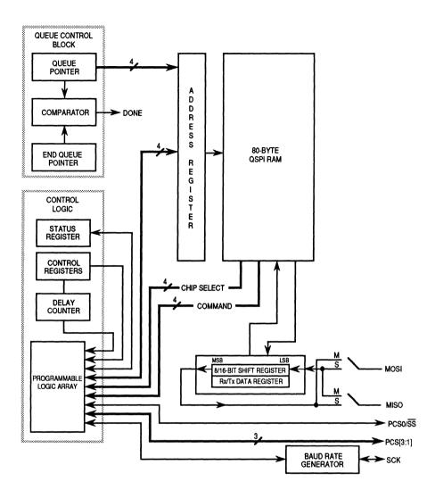
Figure 7-2. QSPI Block Diagram
