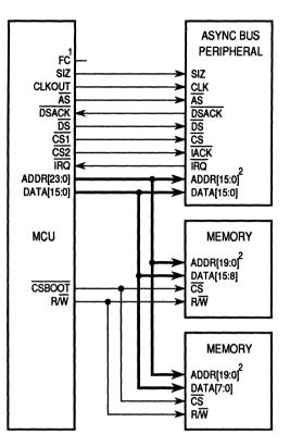
1. CAN BE DECODED TO PROVIDE ADDITIONAL ADDRESS SPACE. 2. VARIES DEPENDING UPON PERIPHERAL MEMORY SIZE.
