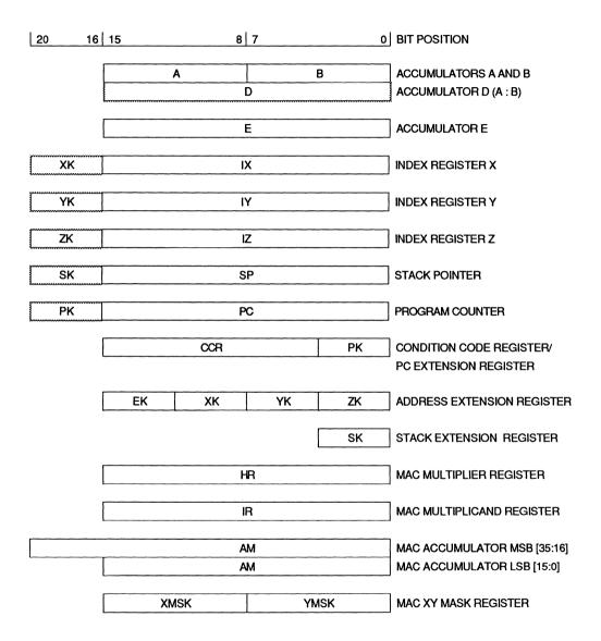
Figure 5-1. CPU16 Register Model
