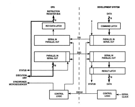
Figure 5-6. BDM Serial I/O Block Diagram
