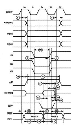
Figure A-10. Fast Termination Read Cycle Timing Diagram
