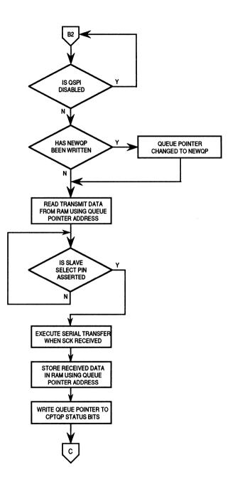
Figure 7-6. Flowchart of QSPI Slave Operation (Part 1)
