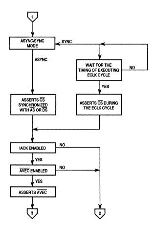
Figure 4-35. Flow Diagram for Chip Select (Sheet 2 of 3)
