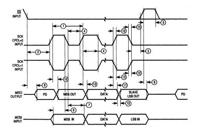
Figure A-19. QSPI Timing Slave, CPHA = 1 APPENDIX A ELECTRICAL CHARACTERISTICS
