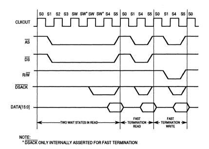
Figure 4-20. Fast-Termination Timing
