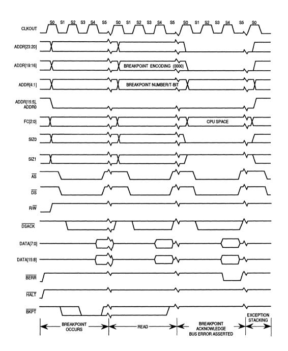
Figure 4–23. Breakpoint Acknowledge Cycle Timing (Exception Signaled)
