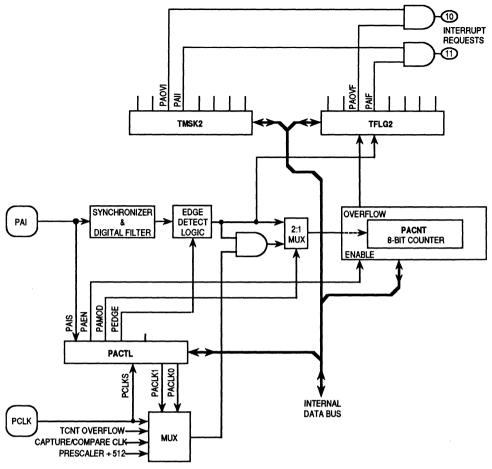
Figure 8–5. Pulse Accumulator Block Diagram
