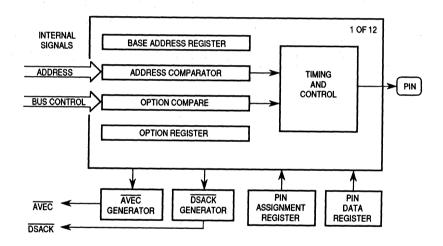
Figure 4-34. Chip-Select Circuit Block Diagram
