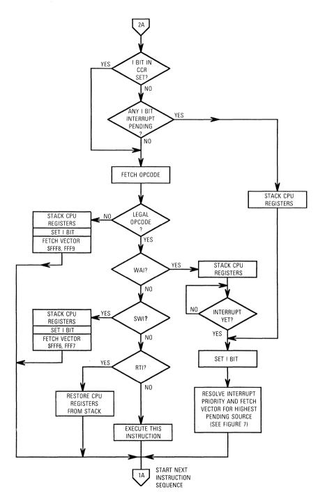
Figure 6-3. Processing Flow Out of Resets (Sheet 2 of 2)
