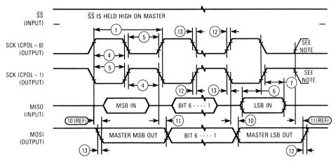
NOTE: The last clock edge is generated internally but is not seen at the SCK pin.
