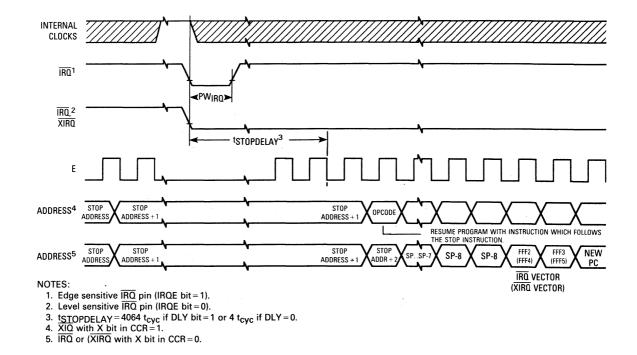
Figure 13-4. STOP Recovery Timing Diagram
