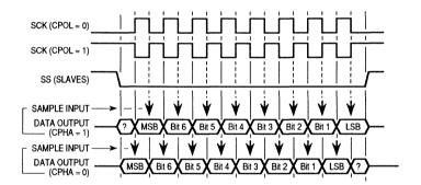
Figure 10-3. SPI Data Clock Timing Diagram
