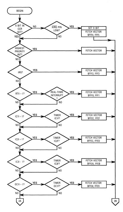
Figure 6-4. Interrupt Priority Resolution (Sheet 1 of 2)
