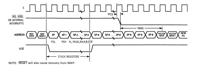
Figure 13-5. WAIT Recovery from Interrupt Timing Diagram
