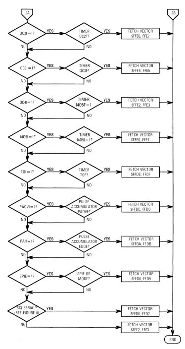
Figure 6-4. Interrupt Priority Resolution (Sheet 2 of 2)
