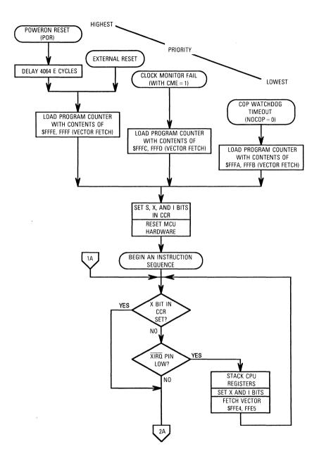
Figure 6-3. Processing Flow Out of Resets (Sheet 1 of 2)
