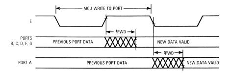
Figure 13-7. Port Write Timing Diagram
