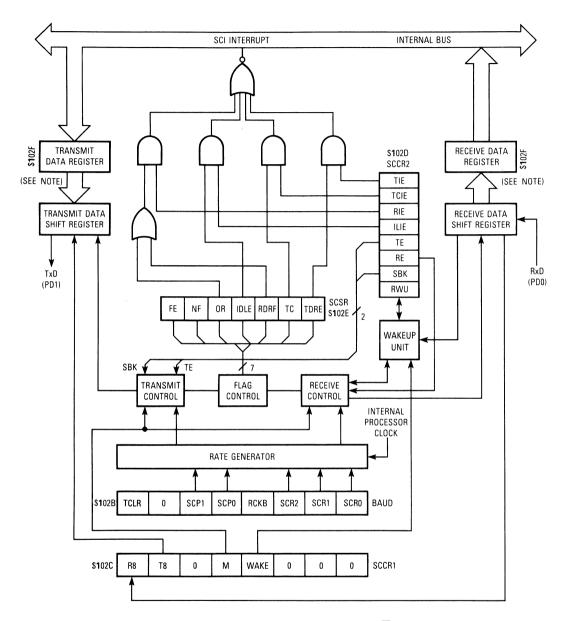
NOTE: The serial communications data register (SCDR) is controlled by the internal R/W signal. It is the transmit data register when written and received data register when read.
