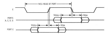
Figure 13-8. Port Read Timing Diagram
