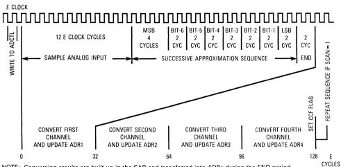
NOTE: Conversion results are built up in the SAR and transferred into ADRx during the END period. The CCF status flag is set during the END period of the fourth conversion after a write to ADCTL. This figure assumes CSEL in the OPTION register is 0 so that the E clock is acting as the conversion clock. IF MULT = 0 all four conversions in the sequence are performed on the same analog channel.
