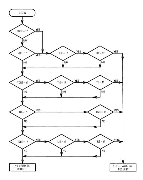
Figure 6-5. Interrupt Source Resolution within SCI
