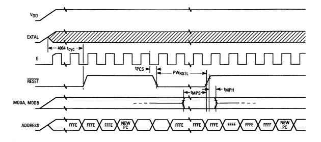
Figure 13-3. POR External Reset Timing Diagram
