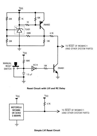
Figure 6-1. Typical LVI Reset Circuits
