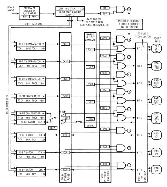
\*Port A pin actions controlled by DDRA, OC1M, OC1D, TCTL1, and TCTL2 registers.
