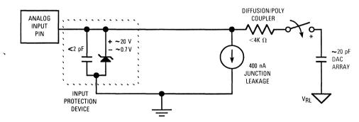
\*This analog switch is closed only during the 12-cycle sample time.
