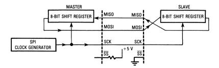
Figure 10-2. SPI Master-Slave Interconnections
