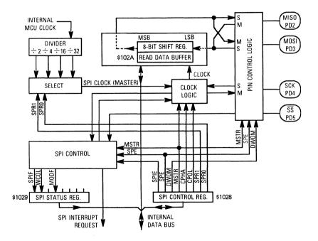
Figure 10-1. SPI Block Diagram
