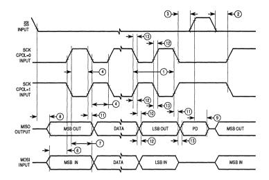
Figure A-3. SPI Timing — Slave, CPHA 0
