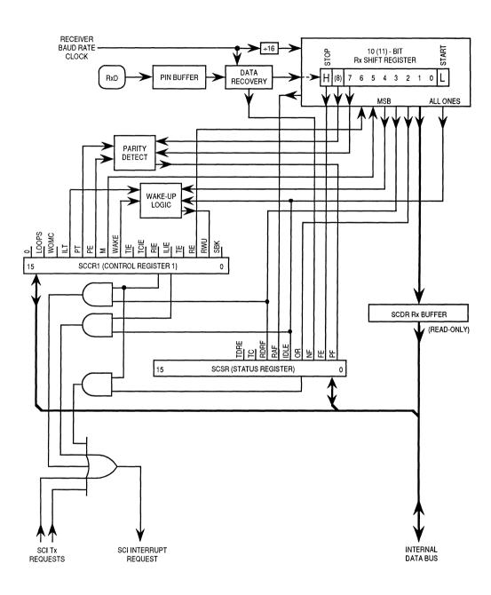
Figure 5-2. SCI Receiver Block Diagram
