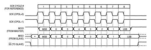
Figure 4-3. CPHA = 1 SPI Transfer Format
