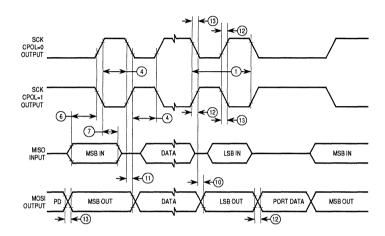
Figure A-1. SPI Timing — Master, CPHA 0
