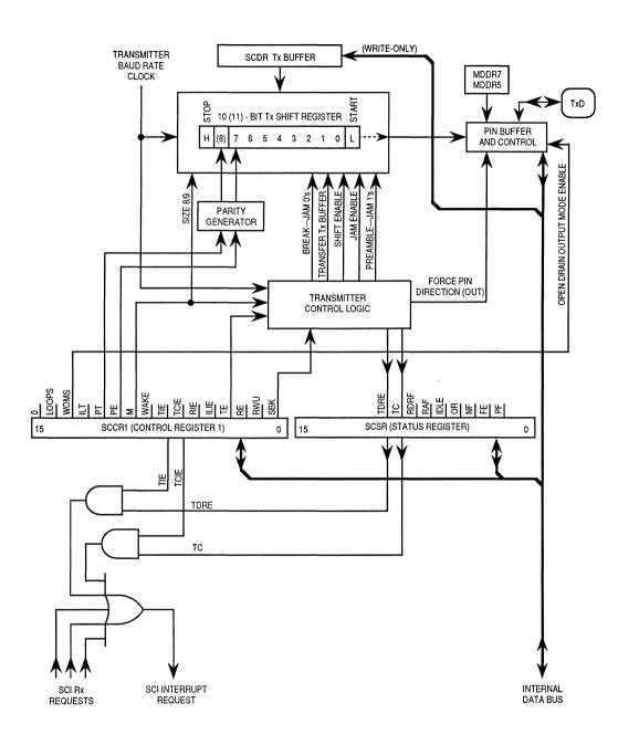
Figure 5-1. SCI Transmitter Block Diagram
