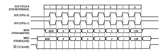
Figure 4-2. CPHA = 0 SPI Transfer Format
