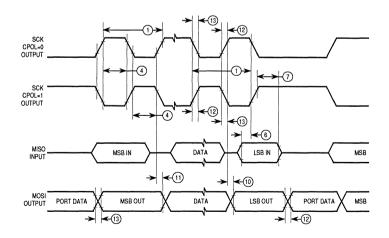
Figure A-2. SPI Timing - Master, CPHA 1
