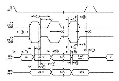
Figure A-4. SPI Timing — Slave, CPHA 1
