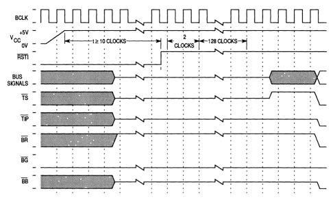
Figure 8-38. Initial Power-On Reset Timing
