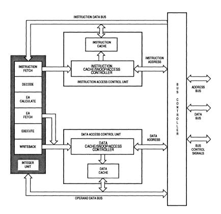
Figure 1-1. MC68EC040 Block Diagram
