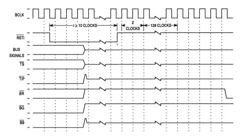
Figure 8-39. Normal Reset Timing
