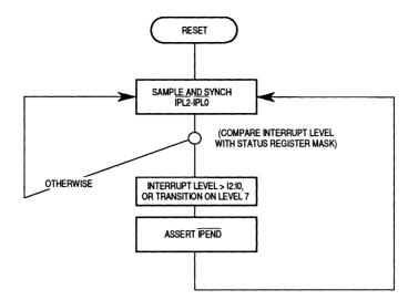
Figure 9-2. Interrupt Pending Procedure
