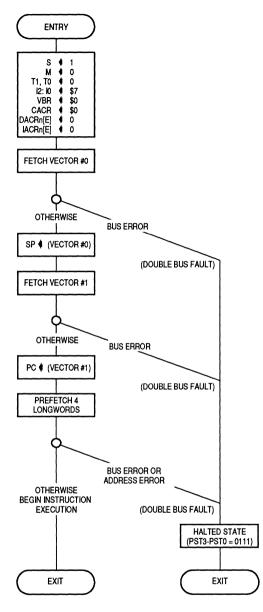
Figure 9-1. Reset Operation Flowchart
