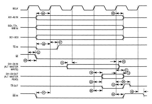
Figure 11-4. Snoop Hit Timing
