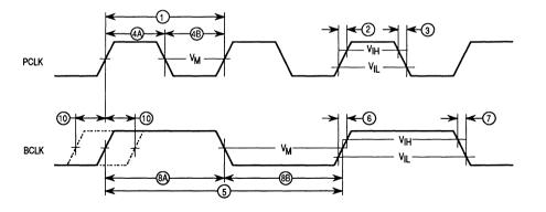
Figure 11-1. Clock Input Timing Diagram
