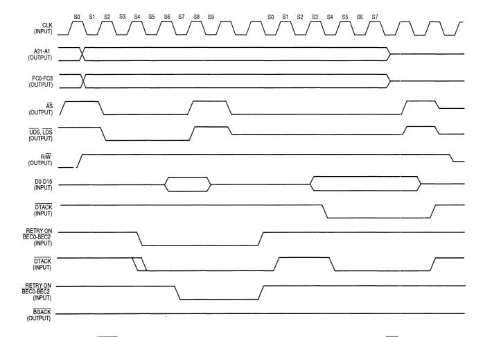
NOTE: Two alternatives of DTACK and retry are drawn in the first one. The second cycle is postponed for one additional cycle due to BEC synchronization.
