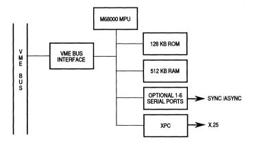
Figure 1-1. XPC System Configuration
