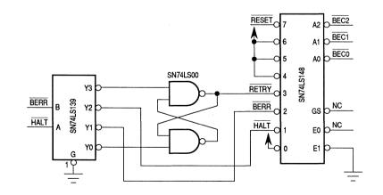
Figure 8-6. Example **BEC** Signal Generation Circuit
