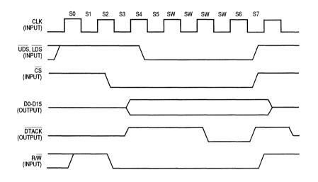
Figure 8-2. Host Processor Write Cycle
