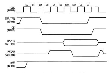
Figure 8-1. Host Processor Read Cycle
