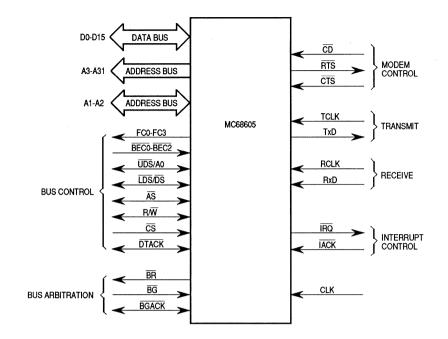
Figure 7-1. Input and Output Signals
