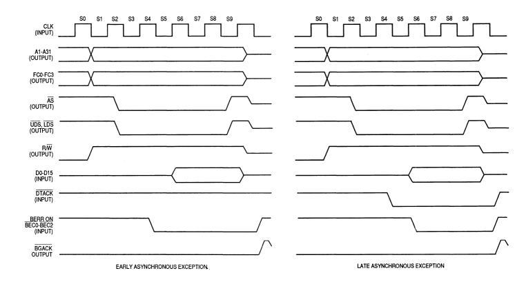
Figure 8-8. Read Cycle with Bus Error
