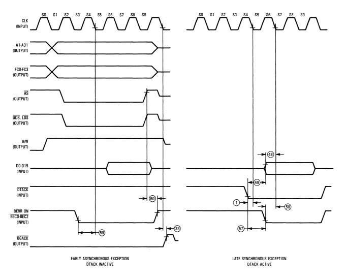
Figure 10-8. Read Cycle with Bus Error Timing Diagram
