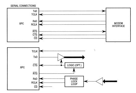
Figure 9-3. Serial Interface Examples
