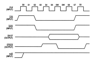
Figure 8-3. Interrupt Acknowledge Cycle
