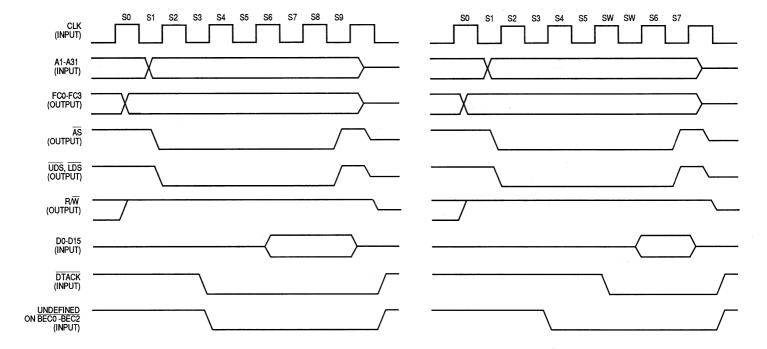
Figure 8-12. Read Cycle with Undefined BEC0-BEC2
