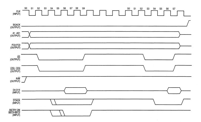
Figure 8-10. Read Cycle with Retry
