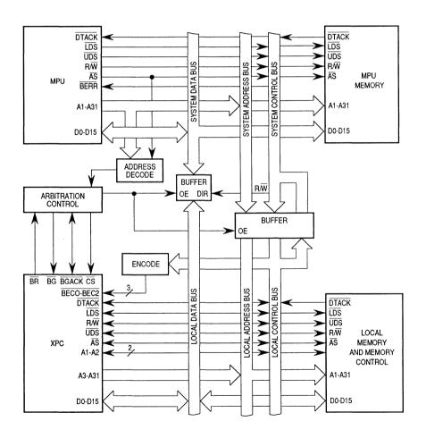
Figure 9-1. XPC-to-Host-Processor Interface
