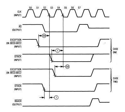
Two alternatives of  $\overrightarrow{\text{DTACK}}$  and exception. Case one has  $\overrightarrow{\text{DTACK}}$  occur after exception and case two has exception occur after  $\overrightarrow{\text{DTACK}}$ . Note that a HALT cycle can be terminated only by  $\overrightarrow{\text{DTACK}}$ .
