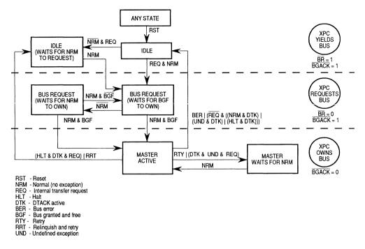
Figure 8-14. MC68605 Bus Arbitration Unit State Diagram
