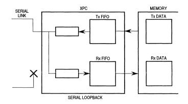
Figure 6-2. Serial Loopback Configuration
