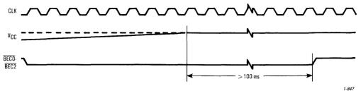
Figure 4-2. Reset Operation Timing Diagram
