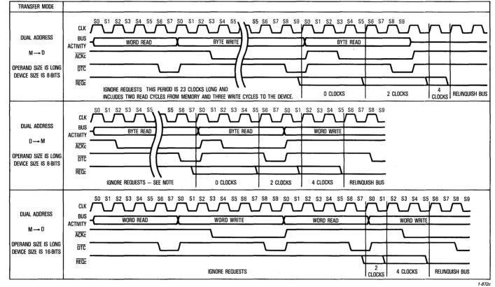
NOTE: This period is 19 clocks long and includes three read cycles from the device and one write cycle to memory.
