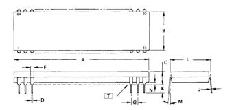
RC SUFFIX PIN GRID ARRAY CASE 765A-01 R SUFFIX PIN GRID ARRAY WITH STANDOFF (Dimensions essentially those of Case 765A-01. See Figure 7-1 for standoff detail.) NOTES:
