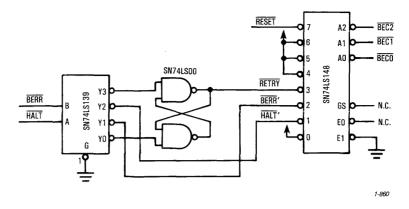
Figure 4-14. Example BEC Signal Generation Circuit
