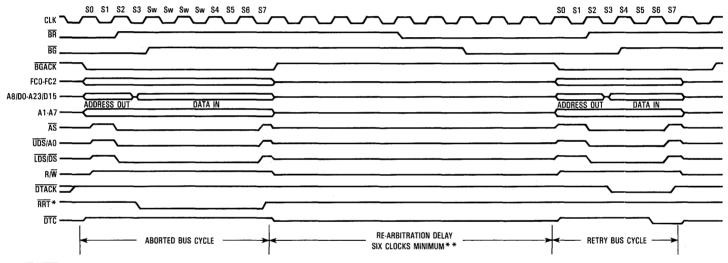
\*BEC2-BEC0 encoded to signal either normal (high) or relinquish and retry (low). \*\*This minimum delay will occur if BG is asserted prior to the clock edge on which BR is asserted.
