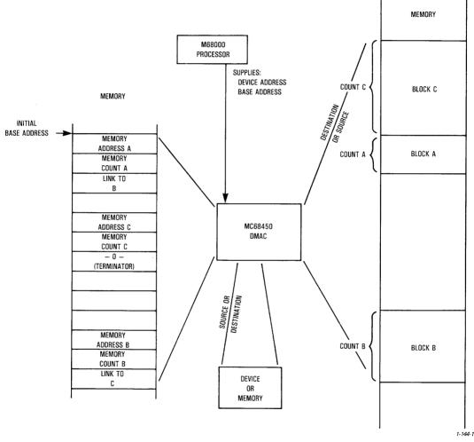
Figure 1-7. Linked Array Chain Transfer
