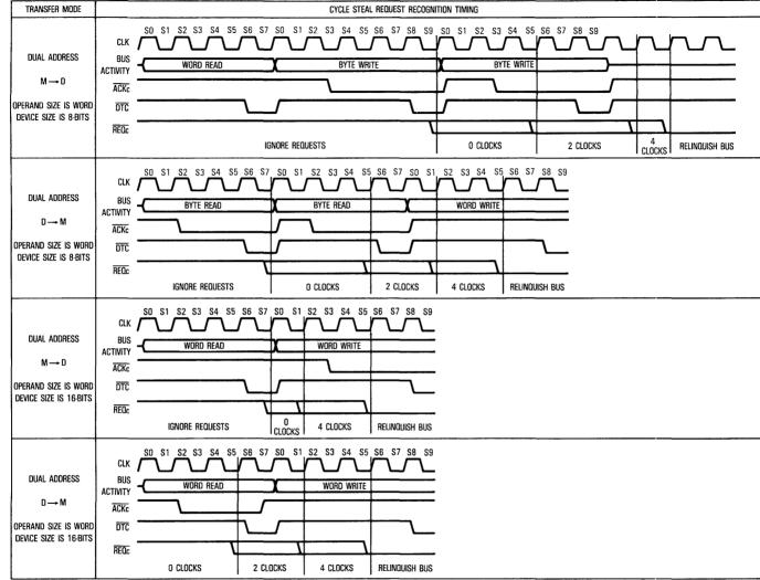
Figure 4-26. Inter-Cycle Overhead Timing Diagram (Sheet 3 of 5)
