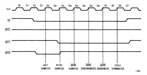
Figure 4-16. BEC Debouncer Timing Diagram
