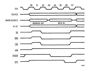
Figure 4-6. M68000 Type Dual Address Read Cycle Timing Diagram
