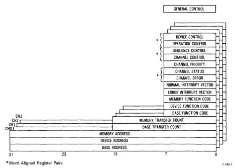
Figure 1-8. DMAC Programmer's Model
