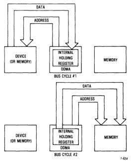
Figure 1-4. Dual-Address Transfer Sequence
