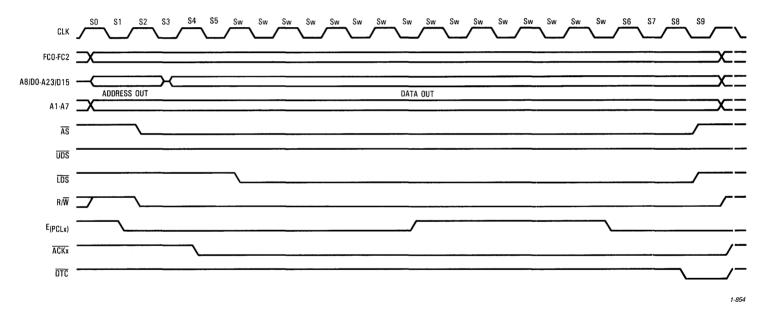
Figure 4-9. M6800 Type Write Cycle Timing Diagram
