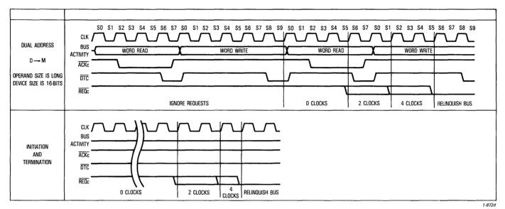
Figure 4-26. Inter-Cycle Overhead Timing Diagram (Sheet 5 of 5)
