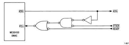
Figure 4-12. READY Circuit for Device with Acknowledge and Ready
