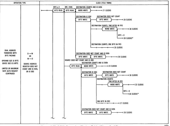
Figure 4-25. DMA Operation Timing Table (Sheet 6 of 7)
