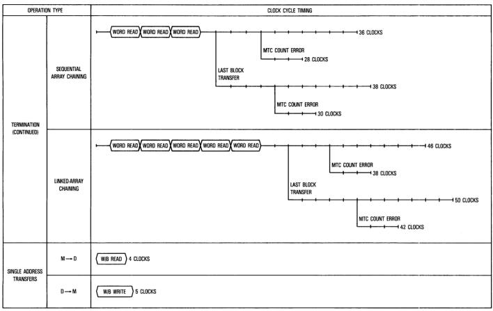
Figure 4-25. DMA Operation Timing Table (Sheet 2 of 7)
