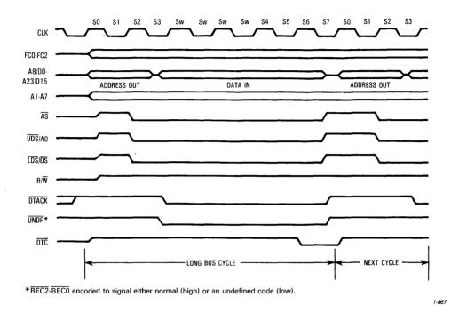
Figure 4-21. Undefined BEC Operation Timing Diagram
