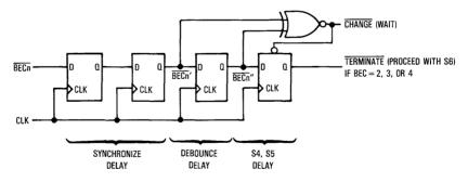
Figure 4-15. BEC Synchronizer Functional Diagram
