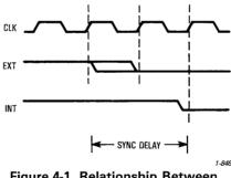
Figure 4-1. Relationship Between External and Internal Signals
