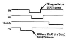
This timing diagram shows that the  $\overline{\text{BR}}$  is negated too early and may cause a bus contention between the MPU and DMAC. The problem occurs in the following conditions:
