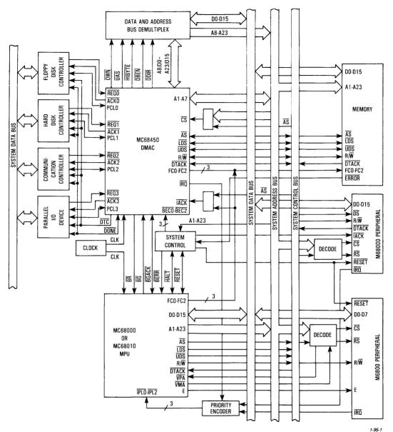
Figure 1-1. Typical M68000-Based System Configuration
