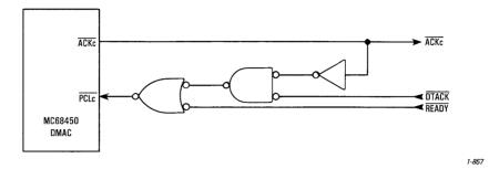
Figure 5-6. READY Circuit for Device With Acknowledge and Ready
