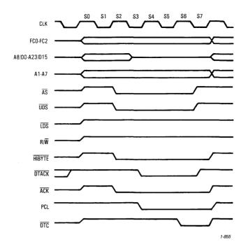
Figure 4-10. Single Address Read Cycle Timing Diagram
