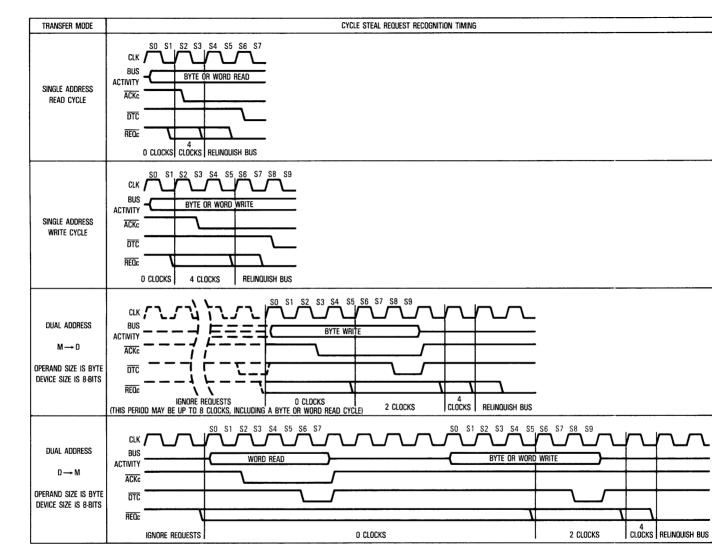
Figure 4-26. Inter-Cycle Overhead Timing Diagram (Sheet 1 of 5)
