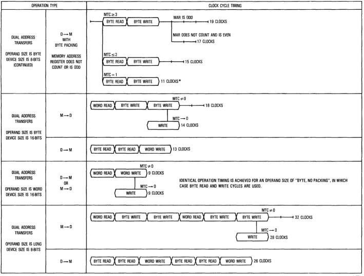
Figure 4-25. DMA Operation Timing Table (Sheet 4 of 7)
