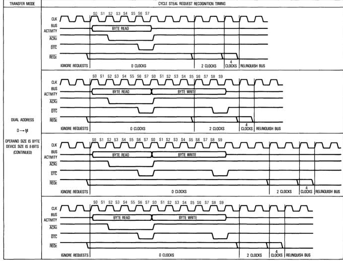
Figure 4-26. Inter-Cycle Overhead Timing Diagram (Sheet 2 of 5)
