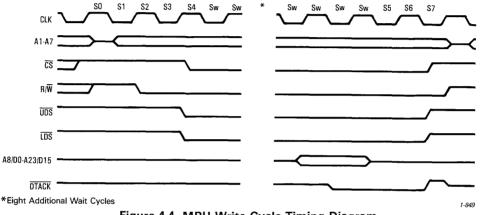
Figure 4-4. MPU Write Cycle Timing Diagram
