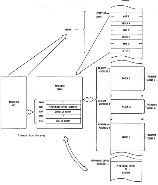
Figure 5-4. Sequential Array Chaining Mode Example
