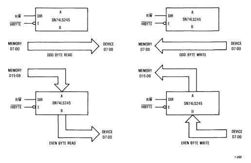
Figure 4-13. Implicitly Addressed 8-Bit Device with 16-Bit Memory Data Flow
