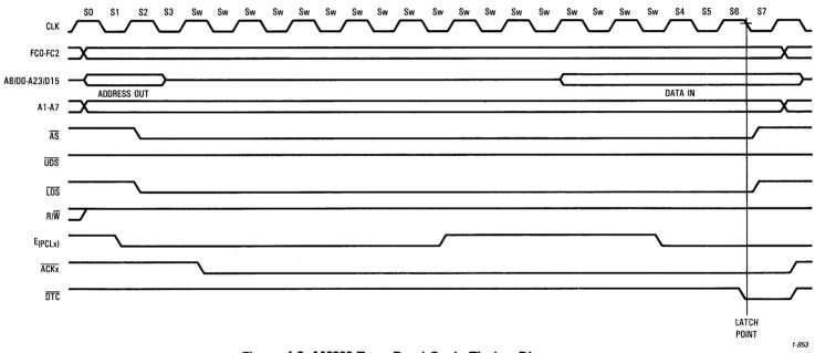
Figure 4-8. M6800 Type Read Cycle Timing Diagram
