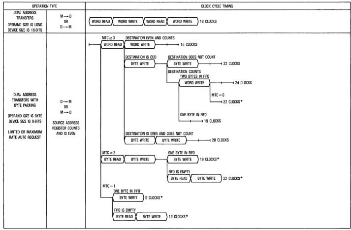
Figure 4-25. DMA Operation Timing Table (Sheet 5 of 7)
