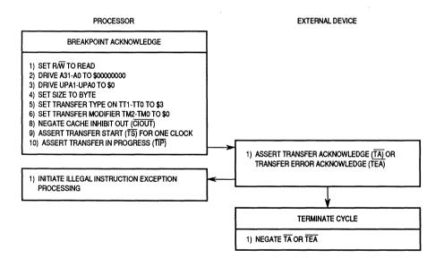
Figure 8-22. Breakpoint Operation Flow
