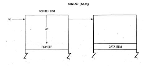
Figure 3-20. Indirect Addressing, Suppressed Index Register
