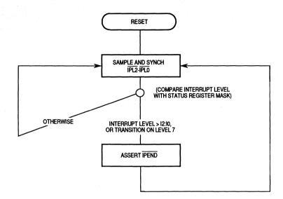
Figure 9-2. Interrupt Pending Procedure
