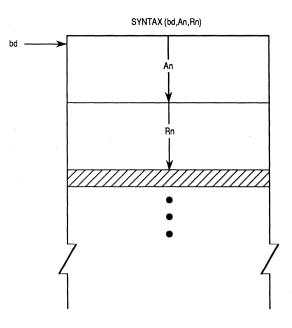
Figure 3-16. Using Absolute Address with Indexes
