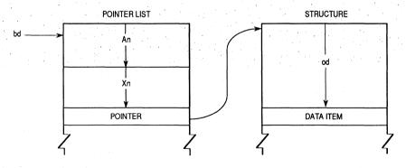
Figure 3-23. Preindexed Indirect with Outer Displacement
