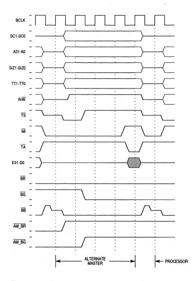
Figure 8-32. Snoop Access with Memory Response
