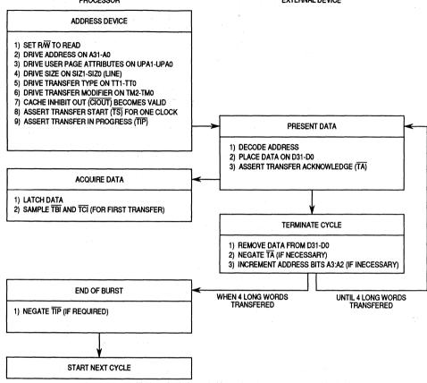
Figure 8-10. Line Read Cycle Flowchart
