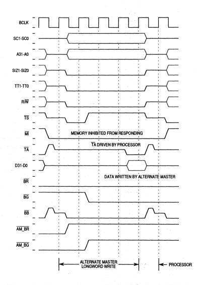
Figure 8-34. Snooped Longword Write, Memory Inhibited
