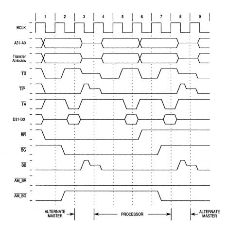
Figure 8-28. Processor Bus Request Example
