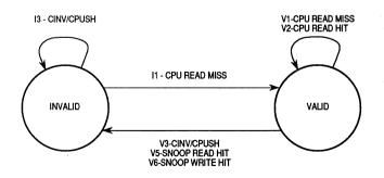
Figure 7-4. Instruction-Cache-Line State Diagram
