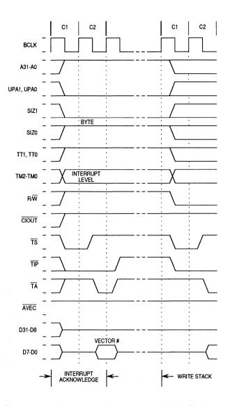
Figure 8-20. Interrupt Acknowledge Cycle Timing
