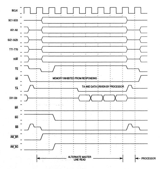
Figure 8-33. Snooped Line Read, Memory Inhibited
