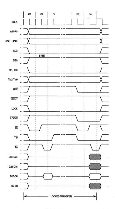
Figure 8-18. Locked Transfer for TAS Instruction
