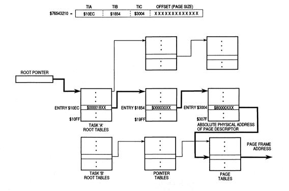
Figure 6-15. Translation Tree Using Indirect Descriptors — Example
