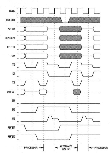
Figure 8-31. Snoop Inhibited Bus Cycle
