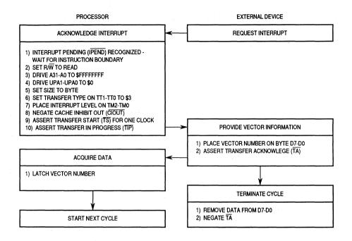
Figure 8-19. Interrupt Acknowledge Cycle Flowchart
