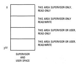
Figure 6-21. Logical Address Map with Shared Supervisor and User Address Spaces — Example
