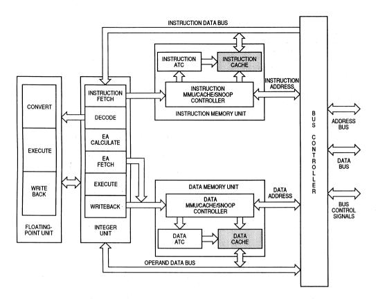
Figure 7-1. Overview of Internal Caches
