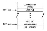
To implement the queue as a circular buffer, the "get" or "put" operation should be performed first, and then the relevant address register should be checked and adjusted, if necessary. The address register is adjusted by adding the buffer length (in bytes) to the register contents.
