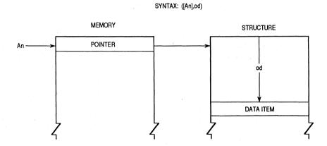
Figure 3-19. Accessing an Item in a Structure Using Pointer
