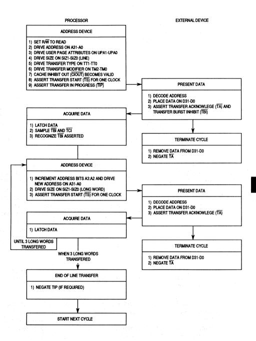
Figure 8-12. Burst-Inhibited Line Read Flowchart
