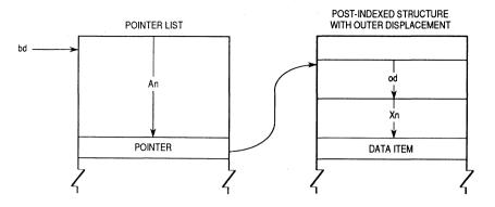
Figure 3-24. Postindexed Indirect Addressing with Outer Displacement
