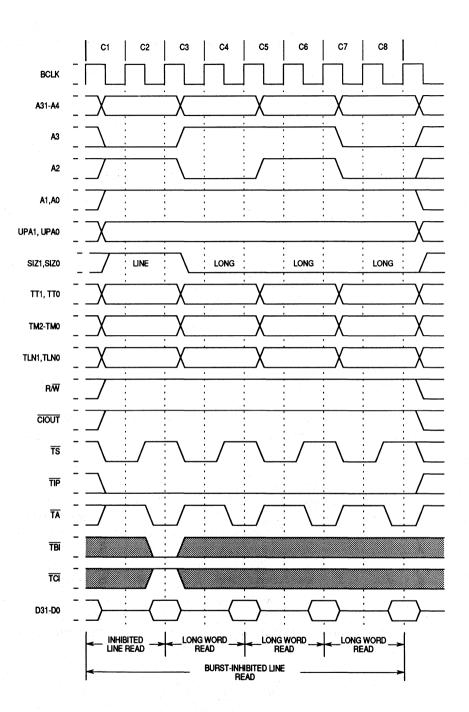
Figure 8-13. Burst-Inhibited Line Read
