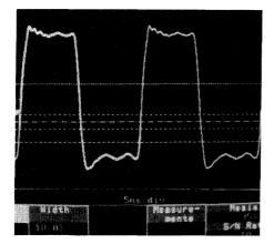
Fig. 1- K11040 Output Waveform Driving 50 pF Load
