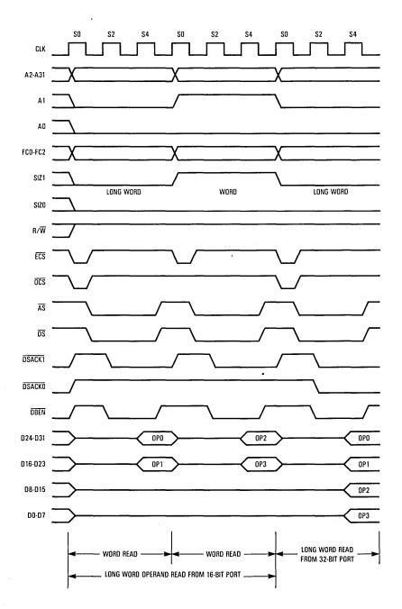
Figure 7-23. Long-Word Read — 16-Bit and 32-Bit Port
