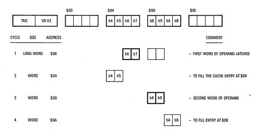
Figure 6-9. Single Entry Mode Operation — Misaligned Long Word and 16-Bit Port
