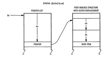
Figure 2-14. Postindexed Indirect Addressing with Outer Displacement
