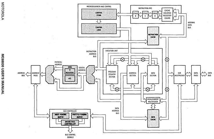
Figure 11-1. Block Diagram — Eight Independent Resources
