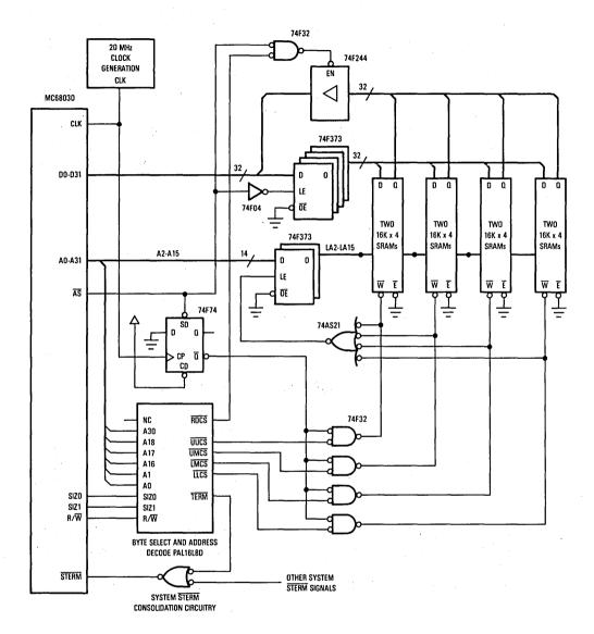
Figure 12-12. Example Two-Clock Read and Write Memory Bank
