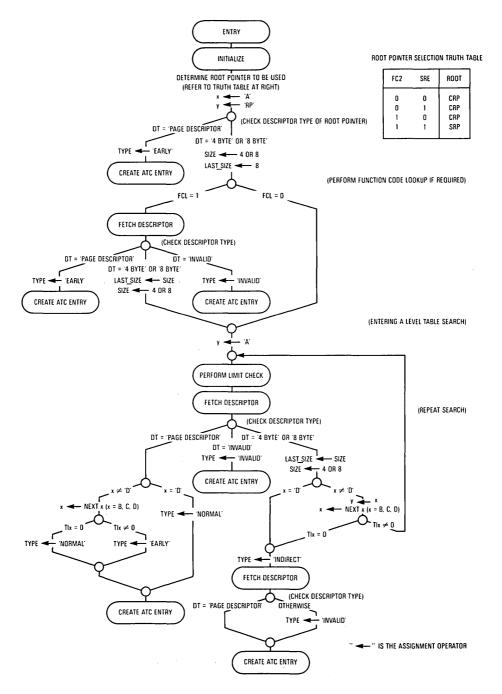
Figure 9-25. Detailed Flowchart of MMU Table Search Operation
