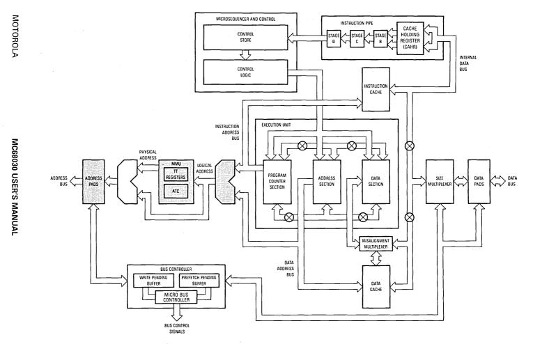
Figure 9-1. MMU Block Diagram
