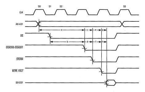
NOTE: This diagram illustrates access time calculations only. DSACKO/DSACK1 and STERM should never be asserted together during the same bus cycle.
