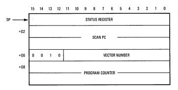
Figure 10-45. MC68030 Post-Instruction Stack Frame
