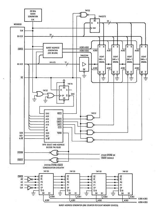
Figure 12-14. Example 2-1-1-1 Burst Mode Memory Bank at 20 MHz, 256K Bytes
