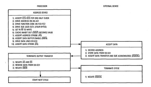
Figure 7-24. Asynchronous Write Cycle Flowchart
