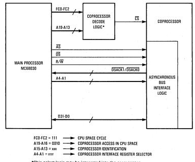
\*Chip select logic may be integrated into the coprocessor Address lines not specified above are "0" during coprocessor access
