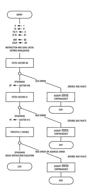
Figure 8-1. Reset Operation Flowchart
