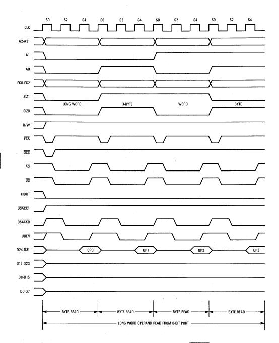
Figure 7-22. Long-Word Read — 8-Bit Port with CIOUT Asserted
