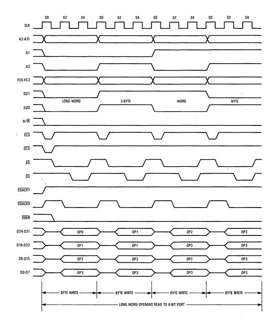
Figure 7-27. Long-Word Operand Write — 8-Bit Port
