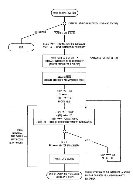
Figure 8-5. Interrupt Exception Processing Flowchart
