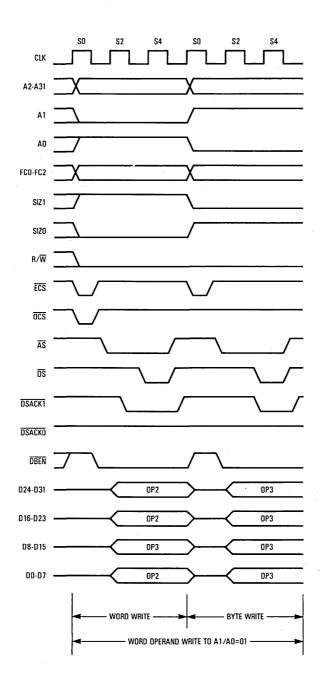
Figure 7-13. Misaligned Word Transfer to Word Port
