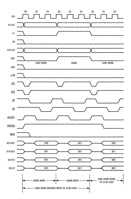
Figure 7-28. Long-Word Operand Write — 16-Bit Port
