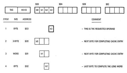
Figure 6-5. Single Entry Mode Operation — 8-Bit Port
