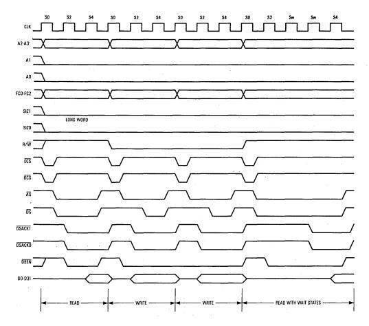
Figure 7-25. Asynchronous Read-Write-Read Cycles — 32-Bit Port
