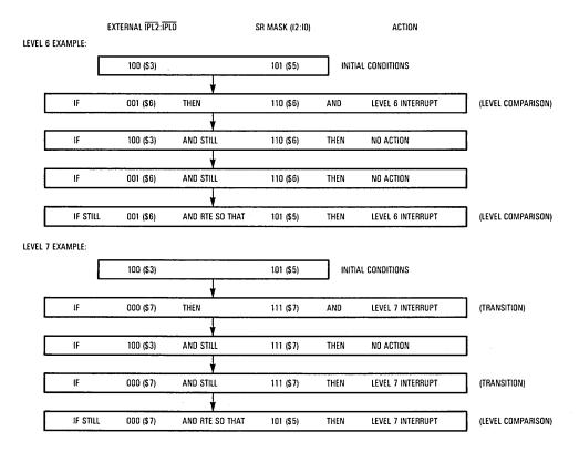
Figure 8-3. Interrupt Recognition Examples
