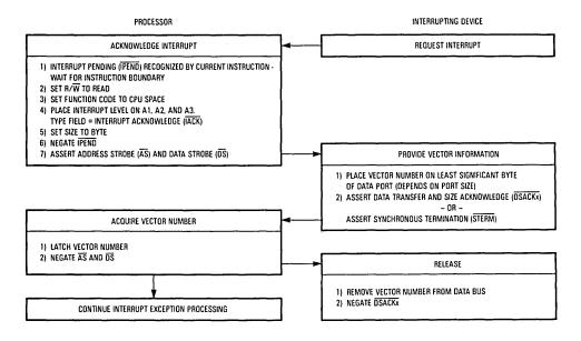
Figure 7-43. Interrupt Acknowledge Cycle Flowchart
