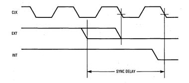
Figure 7-1. Relationship between External and Internal Signals
