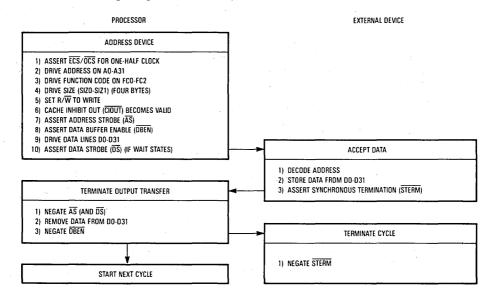
Figure 7-33. Synchronous Write Cycle Flowchart
