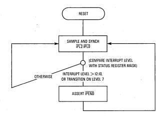
Figure 8-2. Interrupt Pending Procedure
