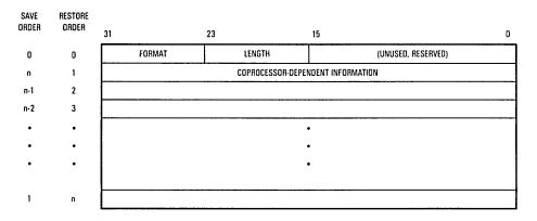
Figure 10-14. Coprocessor State Frame Format in Memory
