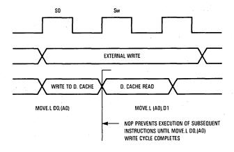
Figure 7-58. Bus Synchronization Example
