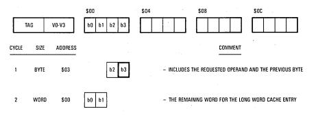
Figure 6-6. Single Entry Mode Operation — 16-Bit Port
