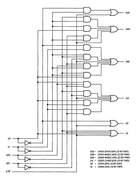
NOTE: These select lines can be combined with the address decode circuitry, or all can be generated within the same programmed array logic unit.
