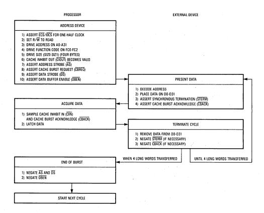
Figure 7-37. Burst Operation Flowchart — Four Long Words Transferred
