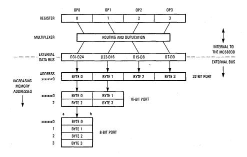
Figure 7-4. MC68030 Interface to Various Port Sizes
