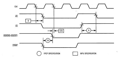
Figure 12-5. Bus Cycle Timing Diagram
