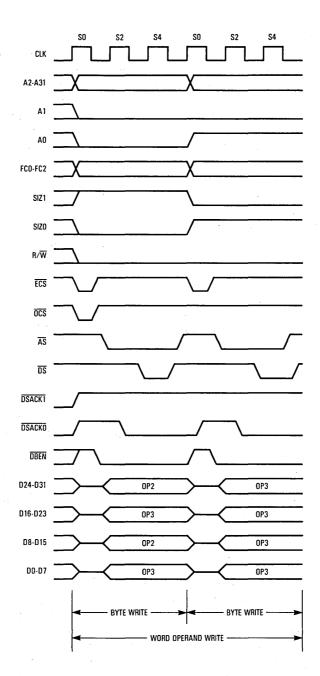
Figure 7-8. Word Operand Write Timing (8-Bit Data Port)
