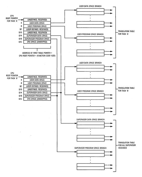
Figure 9-32. Example Translation Tree Structure for Two Tasks
