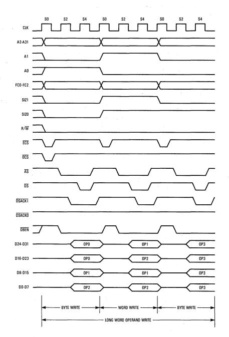
Figure 7-10. Misaligned Long-Word Transfer to Word Port
