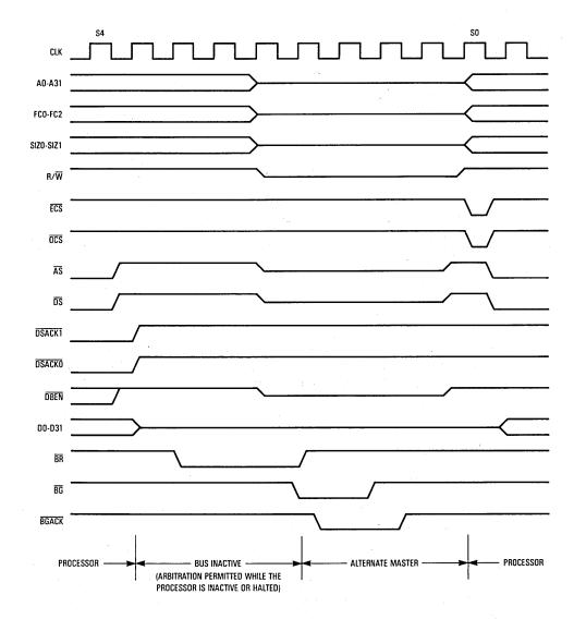
Figure 7-63. Bus Arbitration Operation (Bus Inactive)
