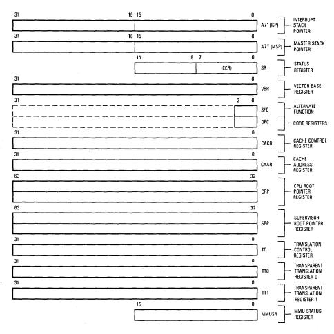
Figure 1-3. Supervisor Programming Model Supplement
