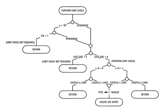
Figure 9-28. Limit Check Procedure Flowchart
