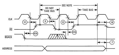
NOTE: The alternate bus master must sample AS high on two consecutive rising edges of the clock (after BGACK is recognized low) before taking the bus.
