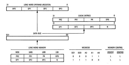
Figure 7-17. Misaligned Cachable Long-Word Transfer from Long-Word Bus
