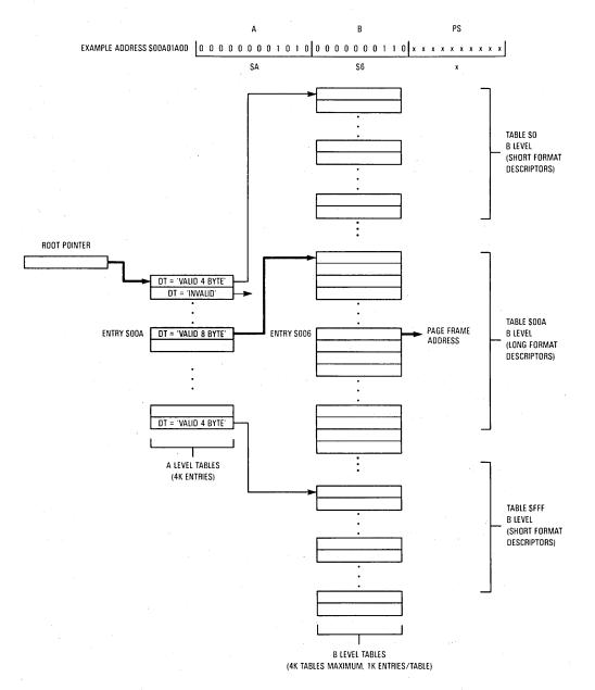
Figure 9-7. Example Translation Tree Using Different Format Descriptors
