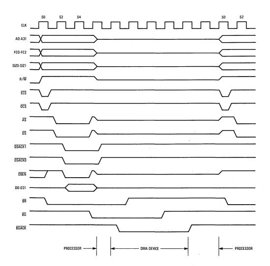
Figure 7-60. Bus Arbitration Operation Timing
