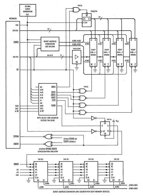
Figure 12-15. Example 3-1-1-1 Pipelined Burst Mode Memory Bank at 20 MHz, 256K Bytes
