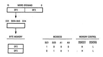
Figure 7-7. Example of Word Transfer to Byte Port
