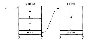
Figure 2-13. Preindexed Indirect Addressing with Outer Displacement
