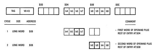
Figure 6-10. Single Entry Mode Operation — Misaligned Long Word and 32-Bit DSACKx Port
