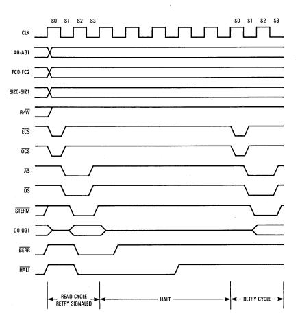
Figure 7-55. Synchronous Late Retry
