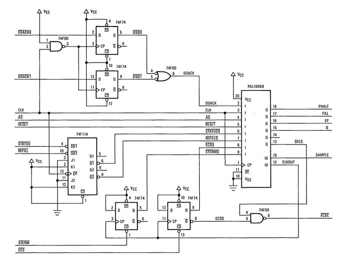
Figure 12-23. Trace Interface Circuit
