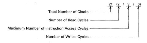
The total numbers of bus-activity clocks and internal clocks (not overlapped by bus activity) of the instruction in this example are derived as follows:
