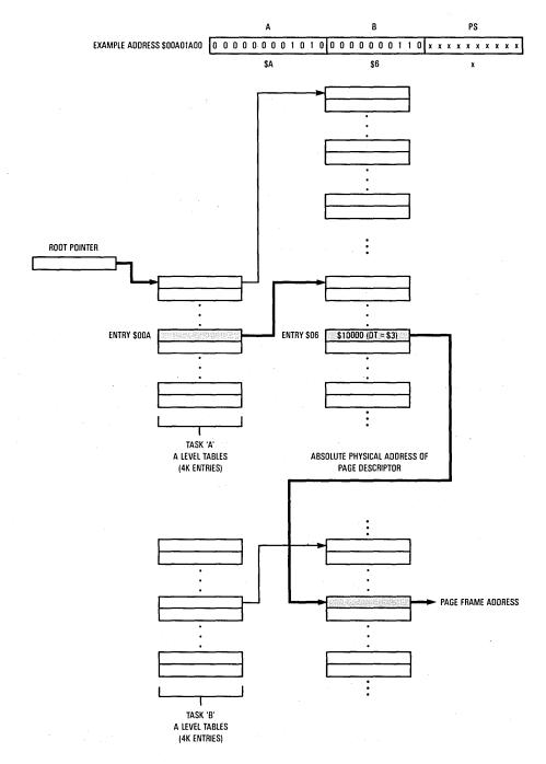
Figure 9-22. Example Translation Tree Using Indirect Descriptors
