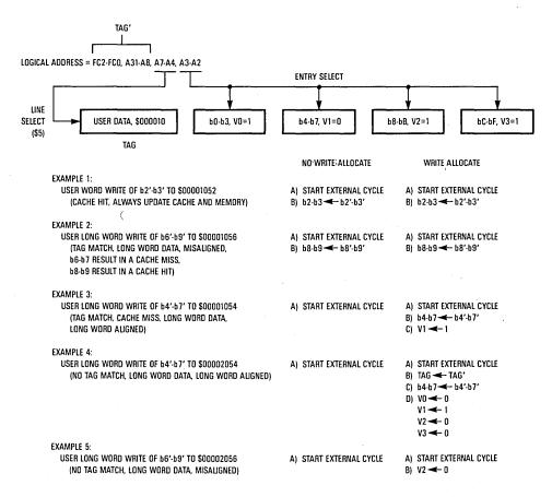
Figure 6-4. No-Write-Allocation and Write-Allocation Mode Examples
