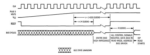
Figure 7-64. Initial Reset Operation Timing
