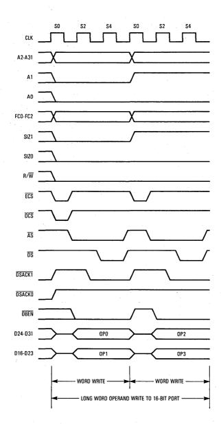
Figure 7-6. Long-Word Operand Write Timing (16-Bit Data Port)
