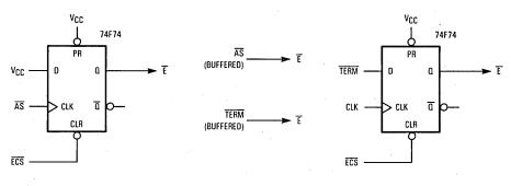
Figure 12-16. Additional Memory Enable Circuits
