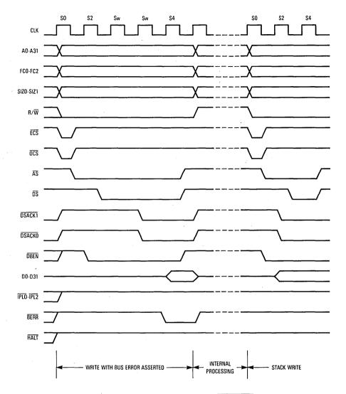
Figure 7-50. Late Bus Error with DSACKx
