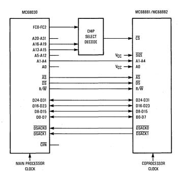
Figure 12-2. 32-Bit Data Bus Coprocessor Connection
