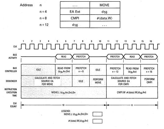
Figure 11-5. Processor Activity — Odd Alignment
