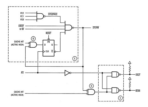
Figure 12-18. Example Early Termination Control Circuit
