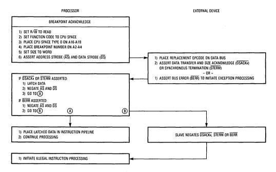
Figure 7-46. Breakpoint Operation Flow
