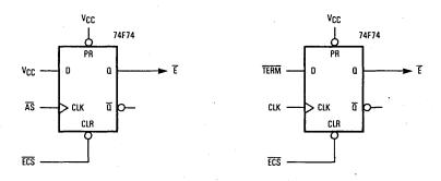
Figure 12-11. Additional Memory Enable Circuits
