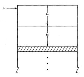
Figure 2-6. Using Absolute Address with Indexes
