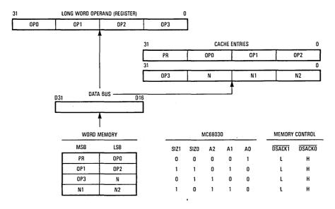
Figure 7-11. Misaligned Cachable Long-Word Transfer from Word Port Example
