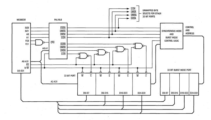
Figure 12-6. Example MC68030 Byte Select PAL System Configuration
