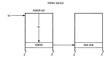
Figure 2-10. Indirect Addressing, Suppressed Index Register
