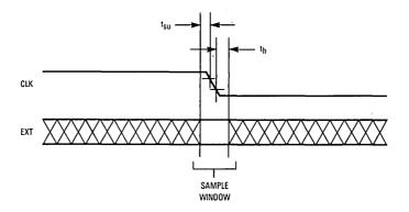
Figure 7-2. Asynchronous Input Sample Window
