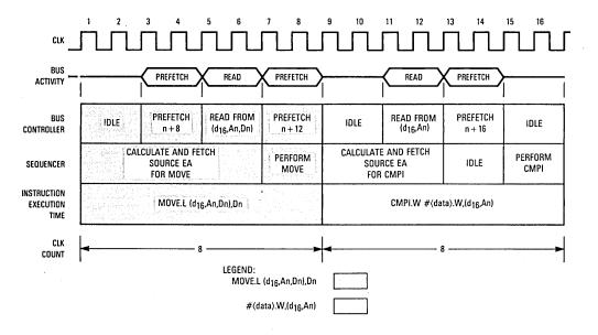
Figure 11-4. Processor Activity — Even Alignment
