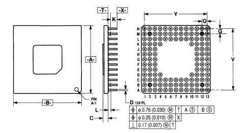
NOTES: 1. DIMENSIONING AND TOLERANCING PER ANSI Y14.5M, 1982. 2. CONTROLLING DIMENSION: INCH. 3. DIMENSION D INCLUDES LEAD FINISH.
