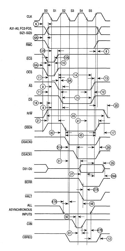
Figure 11. Asynchronous Read Cycle Timing Diagram
