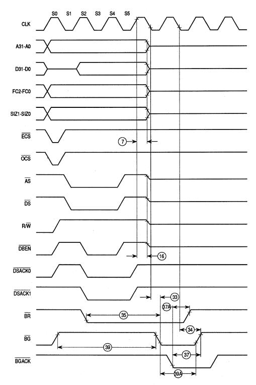
NOTE: Timing measurements are referenced to and from a low voltage of 0.8 V and a high voltage of 2.0 V, unless otherwise noted. The voltage swing through this range should start outside and pass through the range such that the rise or fall will be linear between 0.8 V and 2.0 V.
