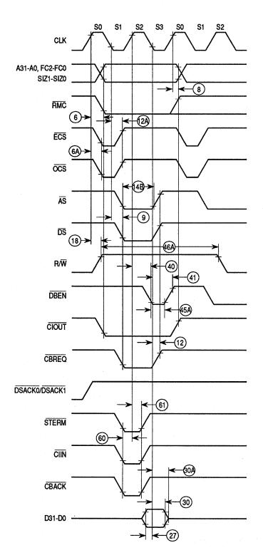
Figure 13. Synchronous Read Cycle Timing Diagram
