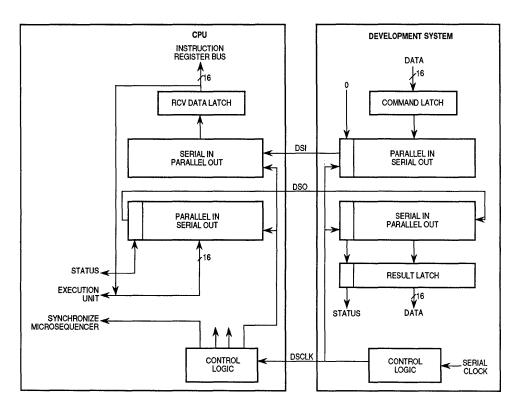
Figure 7-5. Debug Serial I/O Block Diagram
