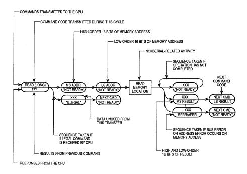
Figure 7-10. Command-Sequence-Diagram Example
