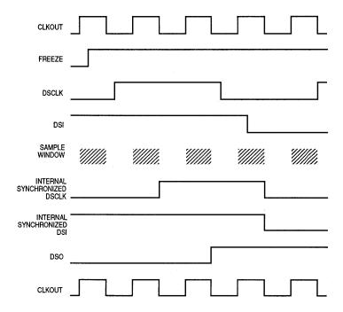
Figure 7-6. Serial Interface Timing Diagram
