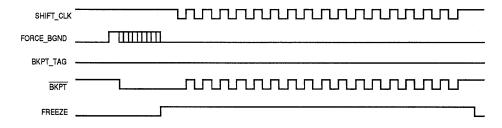
Figure 7-8. BKPT Timing for Forcing BDM
