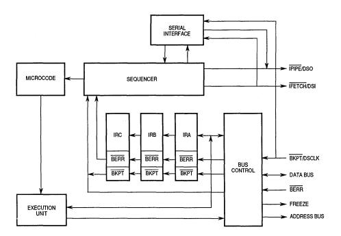
Figure 7-3. BDM Block Diagram
