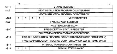
Figure 6-8. Format \$C - Four- and Six-Word BERR Stack
