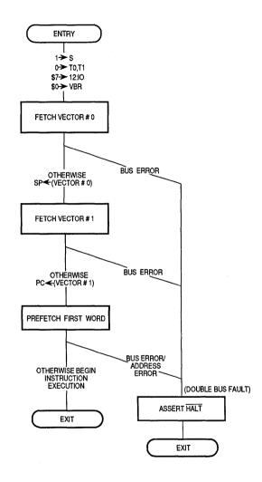
Figure 6-2. Reset Operation Flowchart
