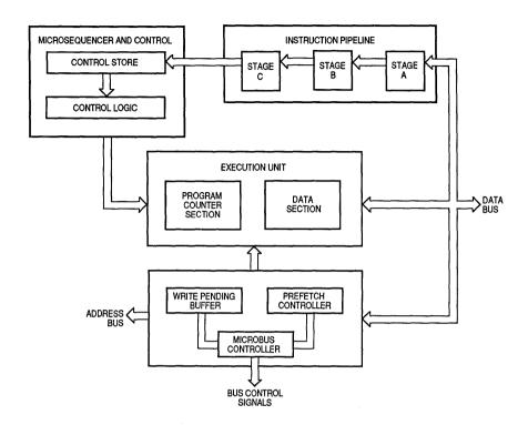
Figure 8-1. Block Diagram of Independent Resources
