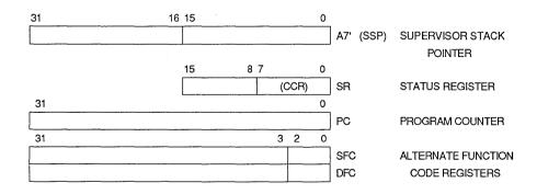
Figure 2-2. Supervisor Programming Model Supplement
