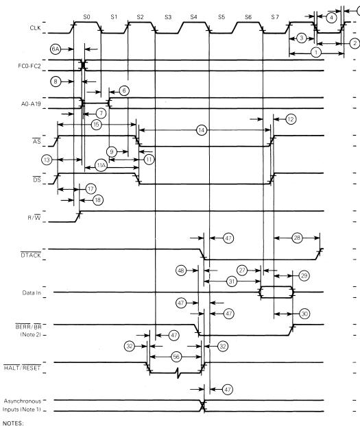
Setup time for the asynchronous inputs IPLO/2, IPL1, and VPA guarantees their recognition at the next falling edge of the clock.
