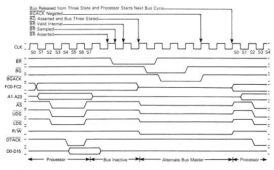
Figure 4-19. Bus Arbitration Timing Diagram-Bus Inactive
