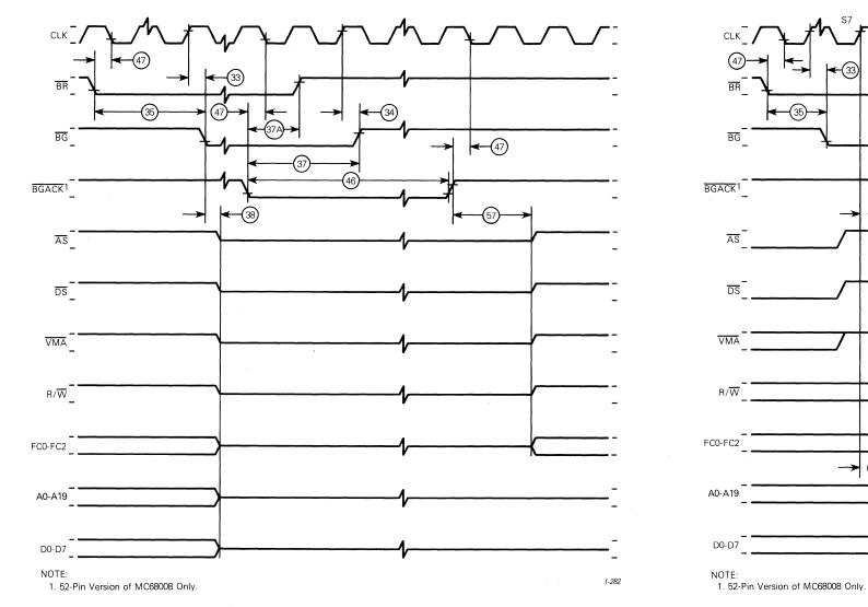
Figure 8-10. Bus Arbitration Timing – Idle Bus Case
