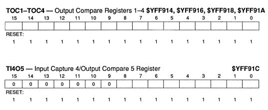
Figure 3-7. Output Compare Registers (TOC1-4/TI4O5)
