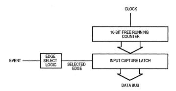
Figure 1-2. Input Capture Simplified Block Diagram
