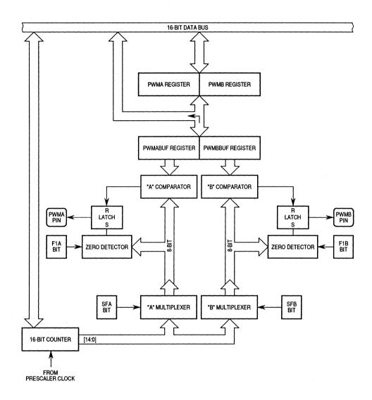
Figure 6-1. PWM Block Diagram
