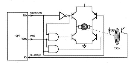
Figure 10-1. Motor Control Example
