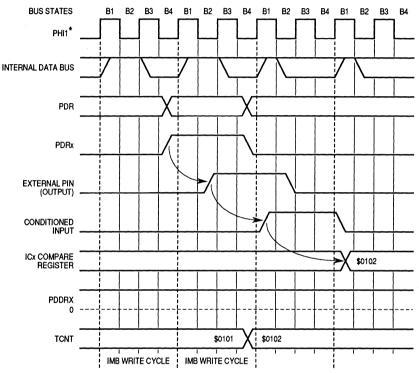
\*PHI1 is the same frequency as the system clock; however, it does not have the same timing.
