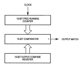
Figure 1-3. Output Compare Simplified Block Diagram
