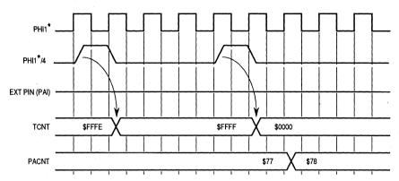
TCNT counts as a result of PHI1\*/4; PACNT counts when TCNT overflows from \$FFFF to \$0000 and the conditioned PAI signal is asserted.
