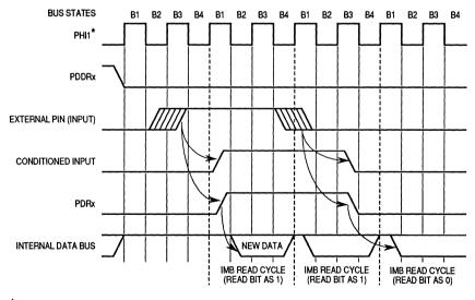
\* PHI1 is the same frequency as the system clock; however, it does not have the same timing.
