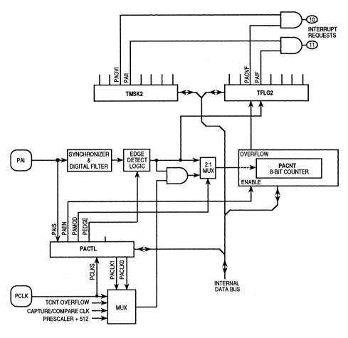
Figure 4-1. Pulse Accumulator Block Diagram
