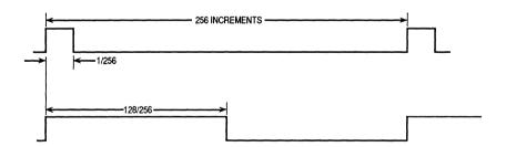
Figure 1-5. Pulse-Width Modulation Example
