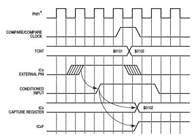
The conditioned input signal causes the current value of the TCNT to be latched by the ICx capture register. The ICxF flag is set at the same time.
