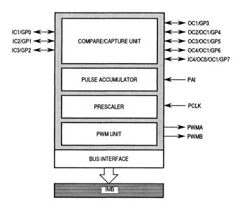
Figure 1-1. GPT Block Diagram
