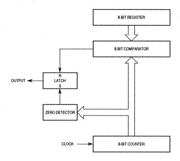
Figure 1-6. Pulse-Width Modulation Simplified Block Diagram
