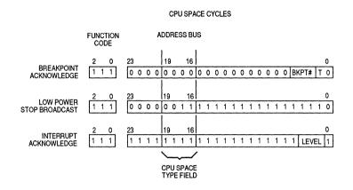
Figure 3-17. CPU Space Address Encoding
