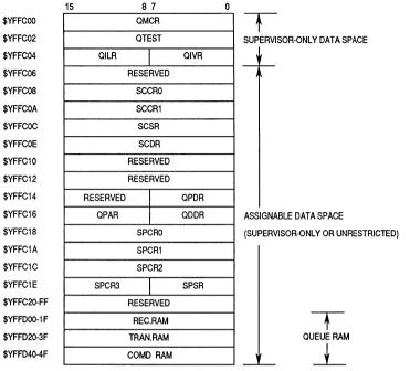
Y = m111 where m is the modmap bit in the SIM MCR (Y = \$7 or \$F).
