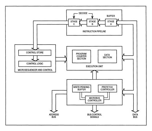
Figure 7-9. CPU32 Block Diagram
