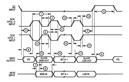
Figure 5-27. QSPI Timing Slave, CPHA 1
