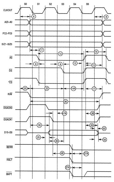
NOTE: All timing with respect to 20% and 70% V  $_{DD}$ \*Timing dependent on programed options (i.e., timed with respect to  $\overline{DS}$  or  $\overline{AS}$  assertion)
