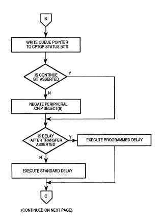
Figure 5-20. Flowchart of QSPI Master Operation (Part 2)
