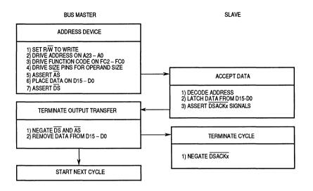
Figure 3-15. Write Cycle Flowchart
