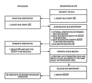
Figure 3-30. Bus Arbitration Flowchart for Single Request
