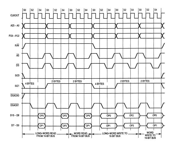
Figure 3-12. Long-Word and Word Read and Write Timing — 16-Bit Port
