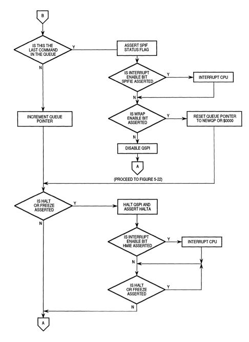
Figure 5-23. Flowchart of QSPI Slave Operation (Part 2)
