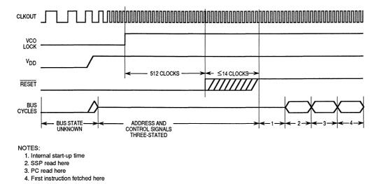
Figure 3-33. Initial Reset Operation Timing
