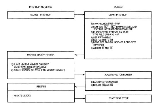
Figure 3-22. Interrupt Acknowledge Cycle Flowchart
