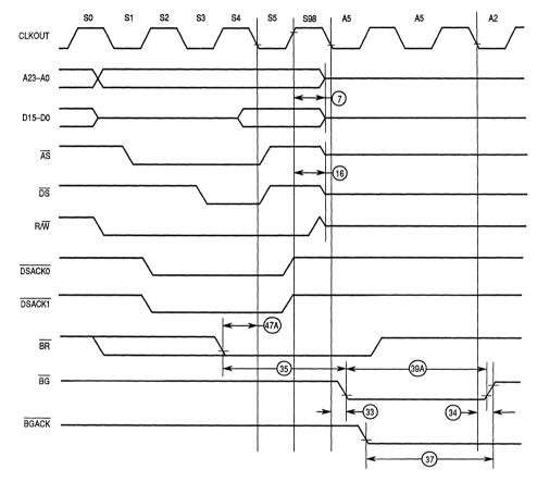
NOTE: All timing with respect to 20% and 70% V  $_{\mbox{DD}}$
