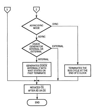
Figure 4-15. Flow Diagram for Chip Select (Sheet 3 of 3)
