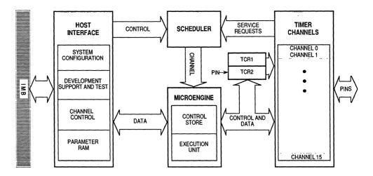
Figure 8-1. TPU Simplified Block Diagram
