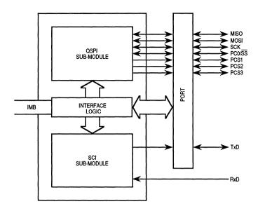
Figure 5-1. QSM Block Diagram
