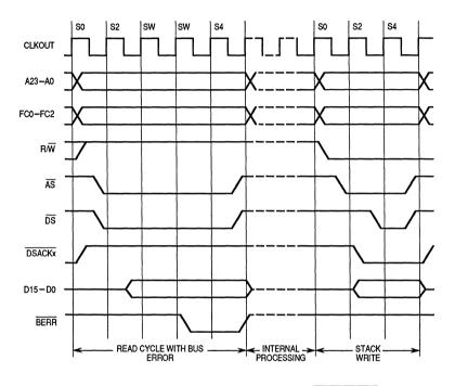
Figure 3-25. Bus Error without DSACKx
