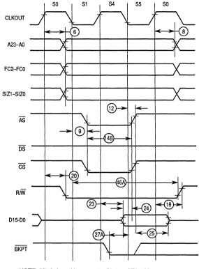
NOTE: All timing with respect to 20% and 70%  $\rm V_{DD}$
