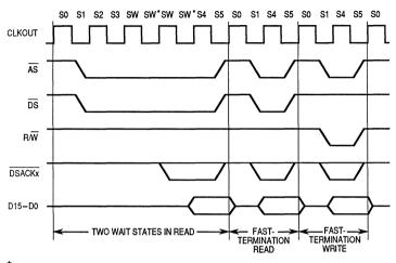
\* DSACKx only internally asserted for fast-termination cycles
