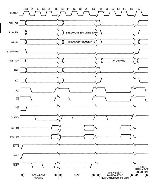
Figure 3-20. Breakpoint Acknowledge Cycle Timing (Opcode Returned)
