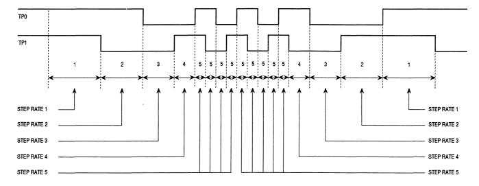
Figure 8-9. Full-Stepping Waveforms, Counterclockwise Rotation
