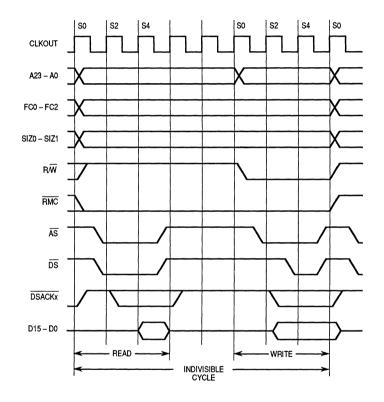
Figure 3-16. Read-Modify-Write Cycle Timing
