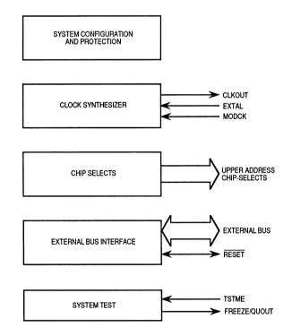
Figure 4-1. System Integration Module Block Diagram
