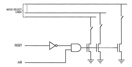
Figure 3-32. Mode Select Conditioning for Reset Operation
