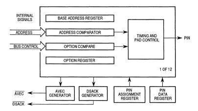
Figure 4-14. Chip-Select Circuit Block Diagram
