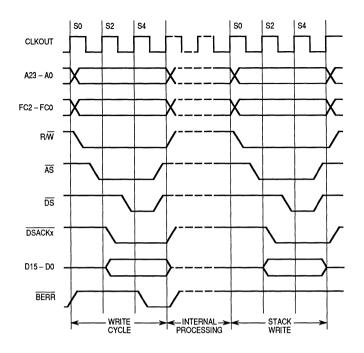
Figure 3-26. Late Bus Error with DSACKx
