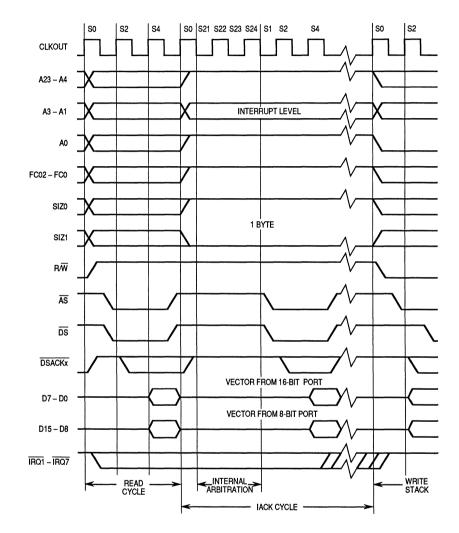
Figure 3-23. Interrupt Acknowledge Cycle Timing
