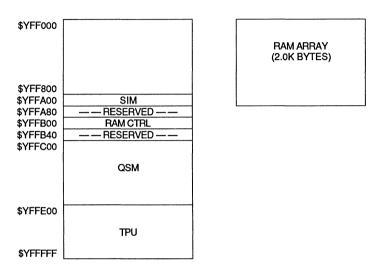
Y = M111, where M is the modmap signal state on the IMB, which reflects the state of the modmap bit in the module configuration register of the system integration module (Y=  $r^{3}$  or  $r^{5}$ ).
