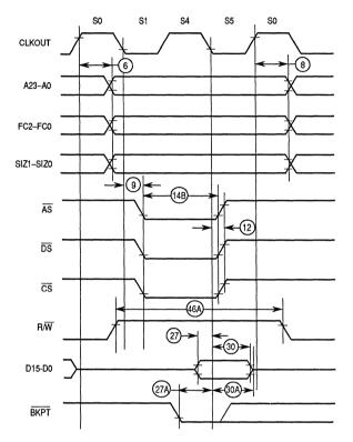
NOTE: All timing with respect to 20% and 70% V  $_{\mbox{DD}}$
