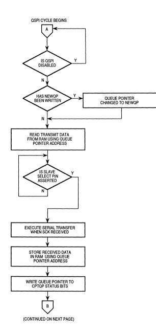
Figure 5-22. Flowchart of QSPI Slave Operation (Part 1)
