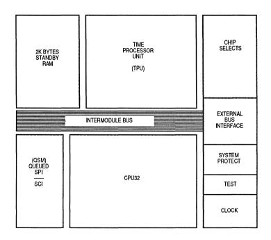
Figure 1-1. Block Diagram of MC68332
