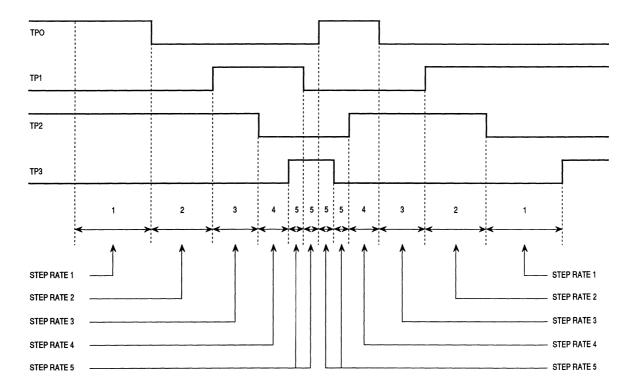
Figure 8-10. Half-Stepping Waveforms, Counterclockwise Rotation
