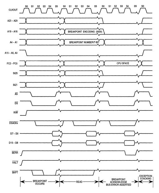
Figure 3-21. Breakpoint Acknowledge Cycle Timing (Exception Signaled)
