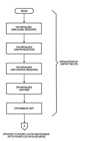
Figure 5-18. Flowchart of QSPI Initialization Operation
