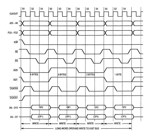
Figure 3-10. Long-Word Write Operand Timing to 8-Bit Port
