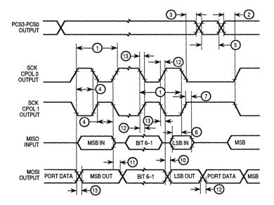
Figure 5-25. QSPI Timing Master, CPHA 1
