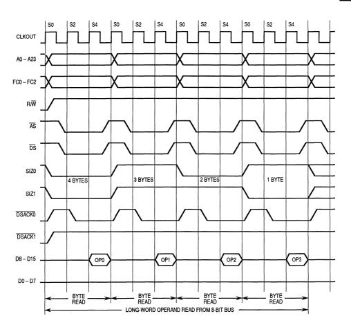
Figure 3-9. Long-Word Operand Read Timing from 8-Bit Data Port
