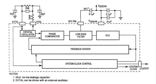
Figure 4-12. Clock Submodule Block Diagram
