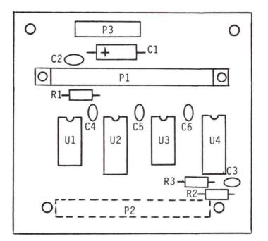
FIGURE 2. Interconnect Adapter Parts Location
