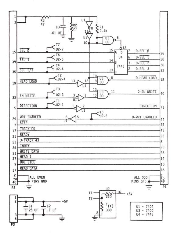
FIGURE 3. Interconnect Adapter Schematic Diagram
