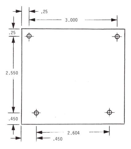
FIGURE 1. Mounting Dimensions
