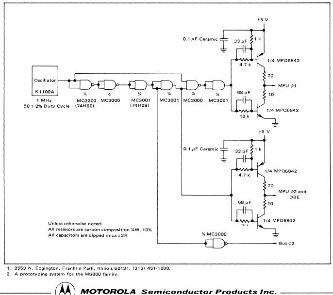
FIGURE 7 – MPU CLOCK CIRCUIT
