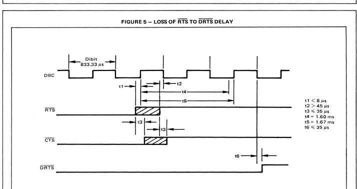
A positive transition of  $\overline{\text{RTS}}$  after  $\overline{\text{CTS}}$  has become active can result in different functional characteristics of the  $\overline{\text{CTS}}$  and  $\overline{\text{DRTS}}$  output signals, depending on the time duration that  $\overline{\text{RTS}}$  remains inactive.
