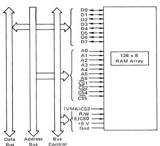
sized systems, this address decoding will be sufficient to distinguish all packages in the system without using any additional address decoding packages.
