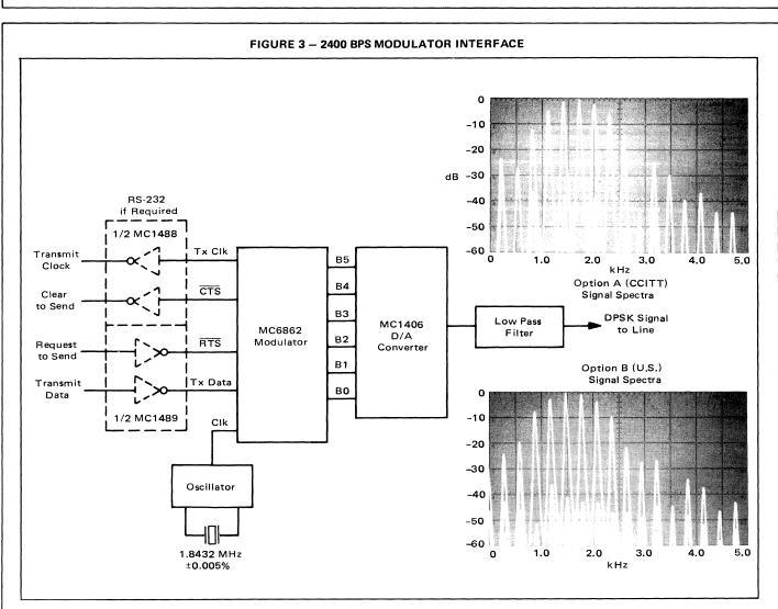
$\overline{\text{CTS}}$  will go low within 35  $\mu$ s after the positive transition of the Dibit Clock (see Figure 4) except when the no-delay option is selected. For the no-delay option,  $\overline{\text{CTS}}$  follows  $\overline{\text{RTS}}$  within 35  $\mu$ s.
