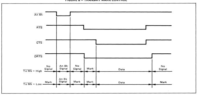
FIGURE 6 – TRANSMIT MARK CONTROL
