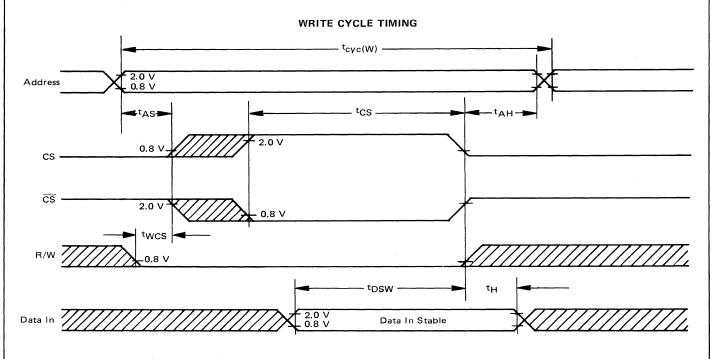
Note: CS and  $\overline{CS}$  can be enabled for consecutive write cycles provided R/W is strobed to V<sub>1H</sub> before or coincident with the Address change, and remains high for time t<sub>AS</sub>.
