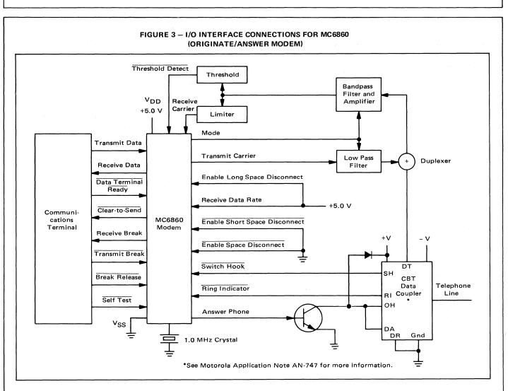
34 ms. The local modem then sends a 3 s continuous space and hangs up provided the Enable Space Disconnect is low. If the remote modem hangs up before 3 s, loss of Threshold Detect will cause loss of Clear-to-Send, which marks the line in Answer Mode and turns the carrier off in the Originate Mode.
