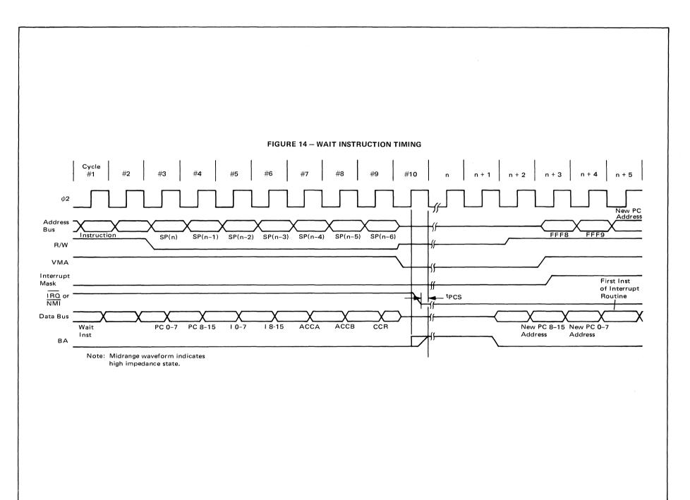
MPU status. When BA is low, the MPU is in the process of executing the control program; if BA is high, the MPU has halted and all internal activity has stopped.
