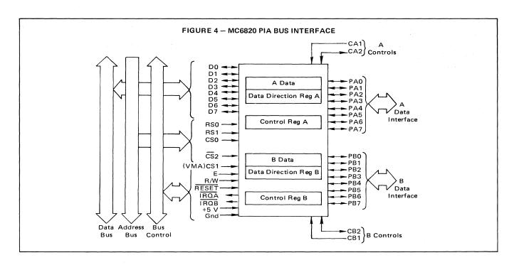
The Reset line is used to initialize the PIA. The Register Select lines RS0 and RS1 serve the same purpose in the PIA as address lines do in memory. They address the control and status registers, thereby making the PIA look like memory to the microprocessor.
