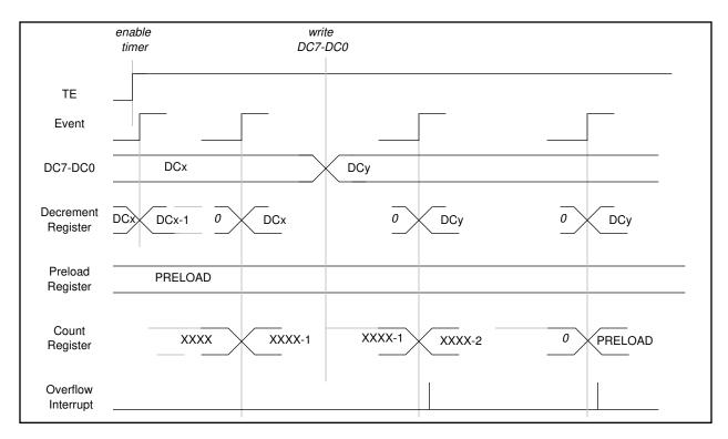
Figure 7-9 Write to DC7-DC0 when the Timer is Enabled
