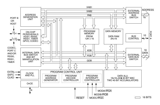
Figure 1-3 Detailed ROM Based Part Block Diagram
