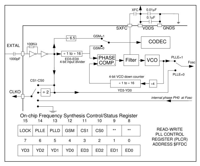
Figure 9-1 Frequency Synthesis Block Diagram and Control Register
