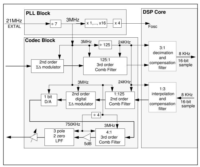
Figure 6-21 Example 2 functional block diagram
