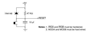
Figure B-4 Reset Circuit
