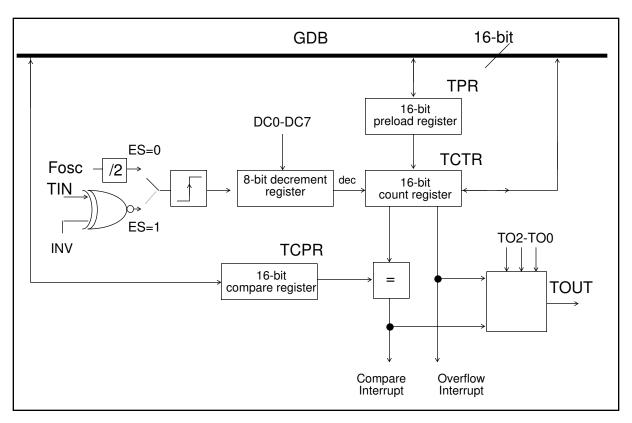
Figure 7-1 16-bit Timer General Block Diagram
