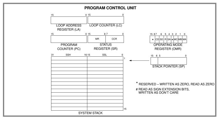
Figure 1-10 DSP56156 Programming Model
