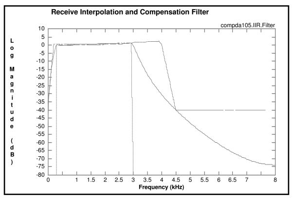
Figure 6-31 Example of a Receive Reconstruction-interpolation IIR Filter
