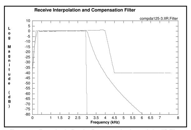
Figure 6-25 Example of a Receive Reconstruction-interpolation IIR Filter
