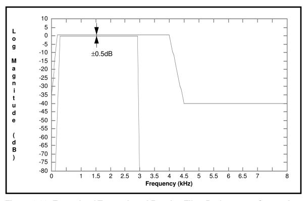
Figure 6-28 Example of Transmit and Receive Filter Performance Constraints
