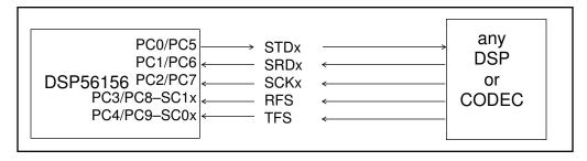
Figure 8-4 SSIx External Clock, Asynchronous Operation
