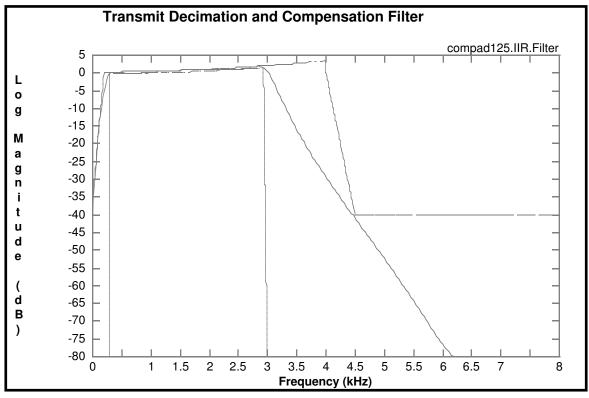
Figure 6-17 Example of a Transmit Antialiasing-decimation IIR Filter
