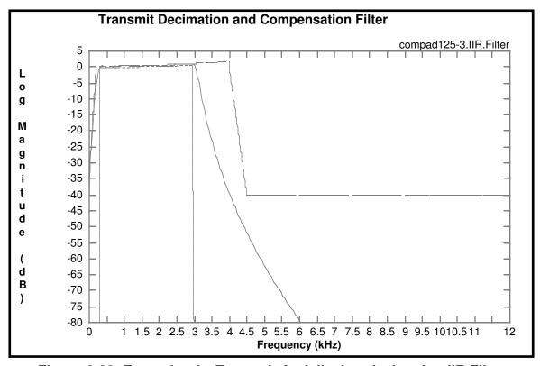
Figure 6-23 Example of a Transmit Antialiasing-decimation IIR Filter
