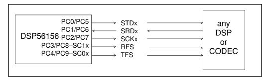
Figure 8-3 SSIx Internal Clock, Asynchronous Operation
