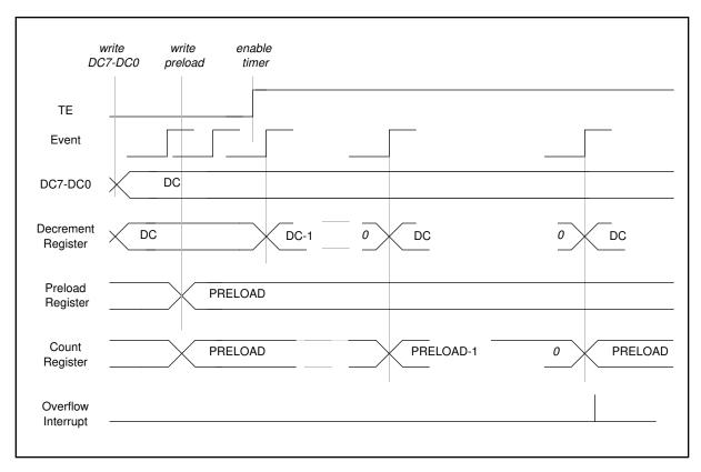
Figure 7-4 Standard Timer Operation with Overflow Interrupt
