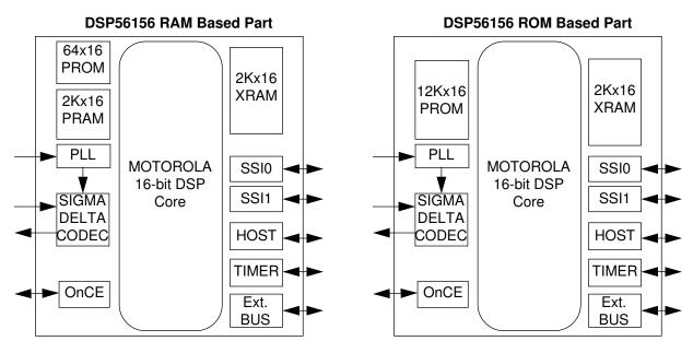
Figure 1-4 DSP56156 RAM and ROM Based Functional Block Diagram
