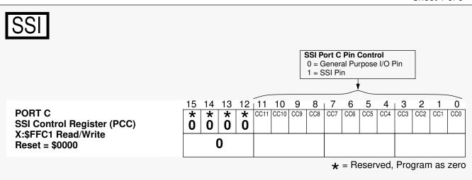
Figure C-32 SSI Control Register (PCC)
