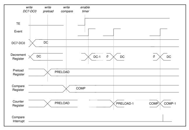
**Figure 7-10 Standard Timer Operation with Compare Interrupt**
