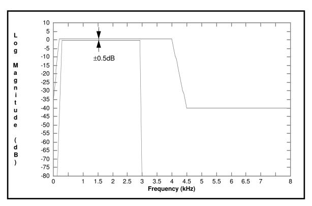
Figure 6-34 Example of Transmit and Receive Filter Performance Constraints
