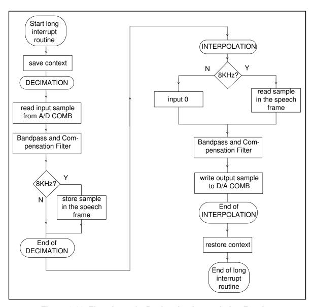
Figure 6-39 Flowchart of a Decimation/Interpolation Routine
