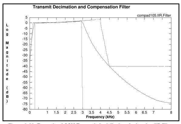
Figure 6-29 Example of GSM Transmit Antialiasing-decimation IIR Filter
