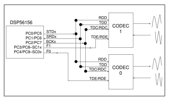
Figure 8-5 SSIx Internal Clock, Synchronous Operation Dual Codec Interface
