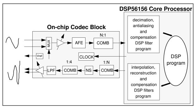
Figure 6-1 DSP56156 On-chip Sigma/Delta Functional Diagram
