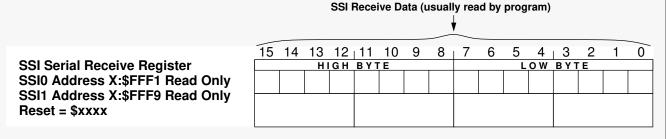
Figure C-33 SSI Serial Receive Register
