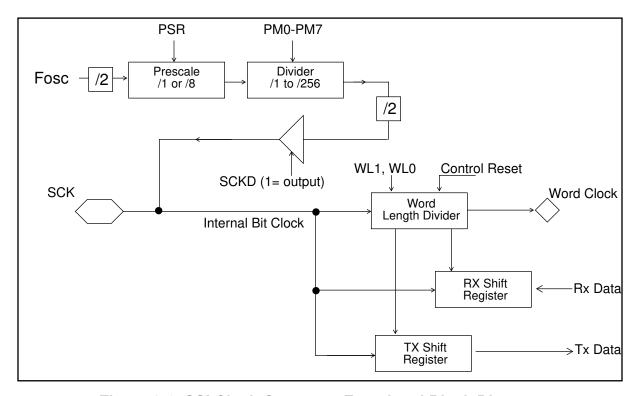
Figure 8-6 SSI Clock Generator Functional Block Diagram
