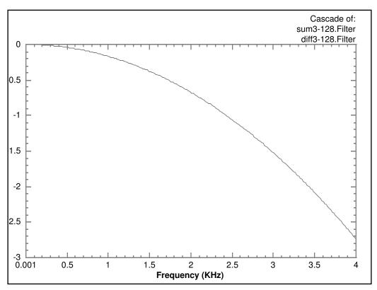
Figure 6-5 Log Magnitude Frequency Response of the A/D Comb Filter in the 0-4 KHz Band for F=2.048 MHz and D=128
