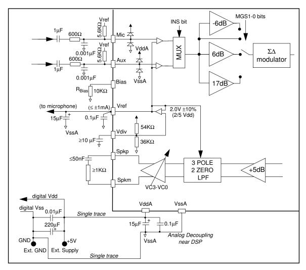
Figure 6-2 DSP56156 Analog Input and Output Diagram
