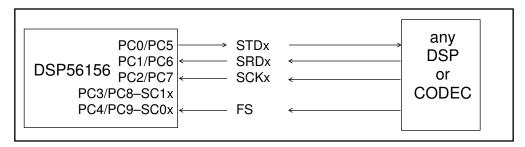
Figure 8-2 SSIx External Clock, Synchronous Operation
