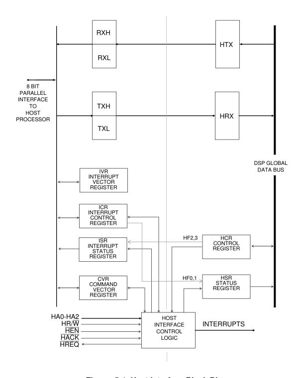
Figure 5-1 Host Interface Block Diagram
