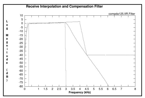
Figure 6-19 Example of a Receive Reconstruction-interpolation IIR Filter
