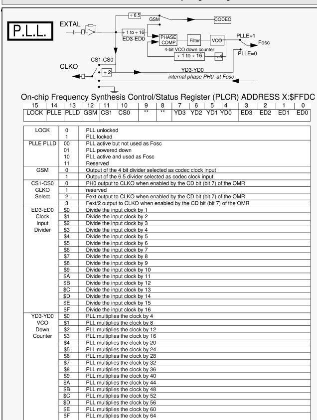
Figure C-7 On-chip Frequency Synthesizer Programming Model Summary
