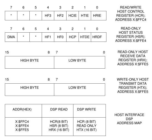
Figure 5-2 Host Interface - DSP Programming Model
