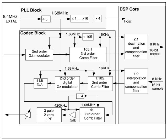
Figure 6-27 Example 3 functional block diagram
