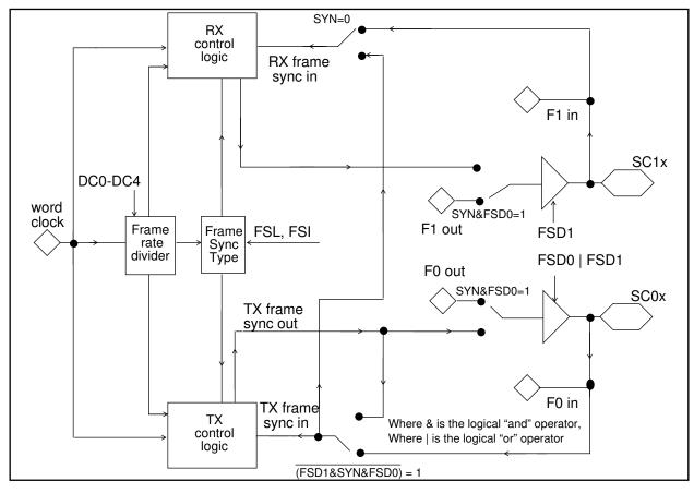
Figure 8-7 SSIx Frame Sync Generator Functional Block Diagram
