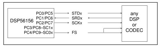
Figure 8-1 SSIx Internal Clock, Synchronous Operation
