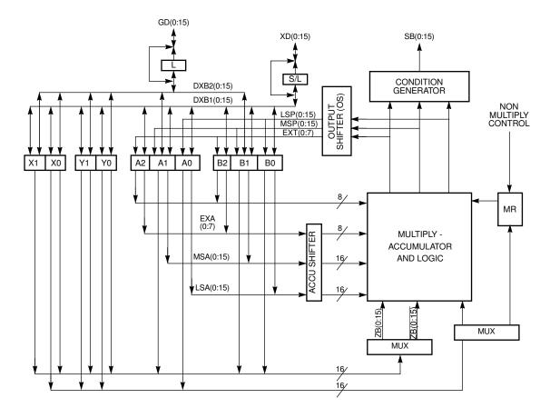
Figure 1-6 Data ALU Architecture Block Diagram
