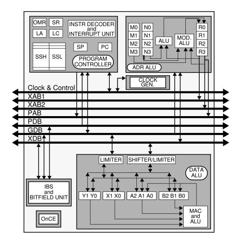
Figure 1-5 DSP56100 CORE Block Diagram
