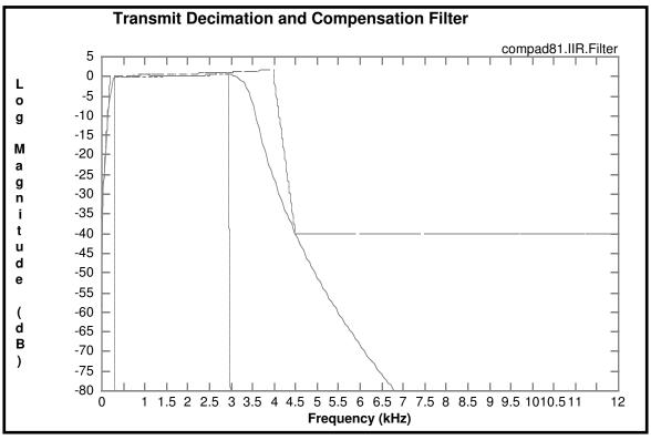
Figure 6-35 Example of a Transmit Antialiasing-decimation IIR Filter
