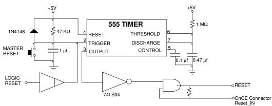
Figure B-5 Reset Circuit Using 555 Timer
