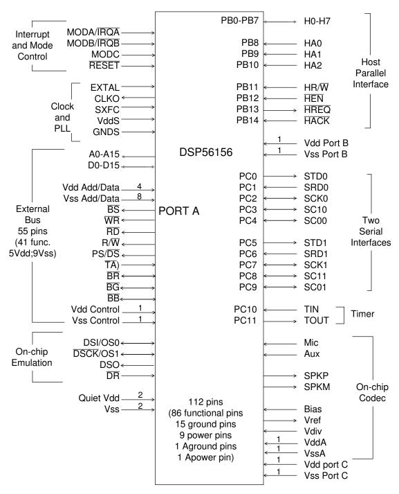
Figure 2-2 DSP56156 Pinout
