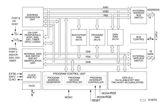
Figure 1-2 Detailed RAM Based Part Block Diagram
