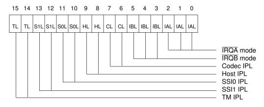
Figure 1-8 Interrupt Priority Register IPR (Address X:\$FFDF)
