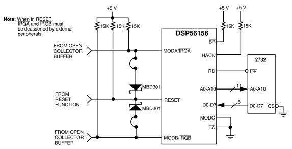
Figure B-1 No Glue Logic, Low Cost Memory Port Bootstrap — Mode 0
