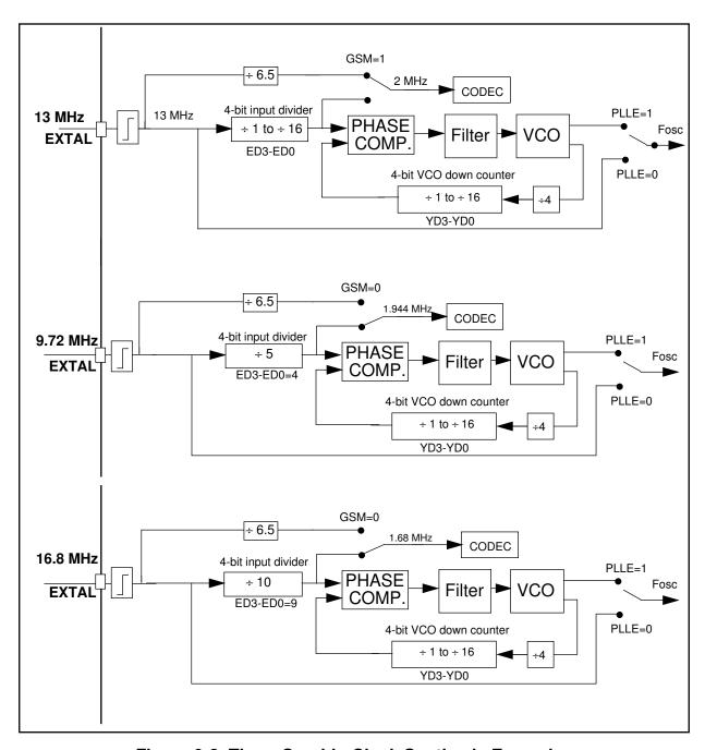
Figure 9-2 Three On-chip Clock Synthesis Examples
