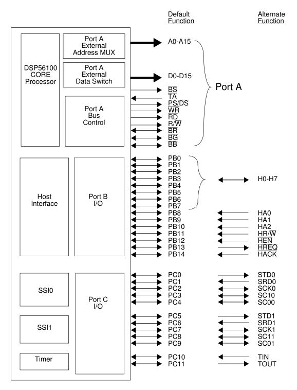
Figure 4-1 DSP56156 Input / Output Block Diagram
