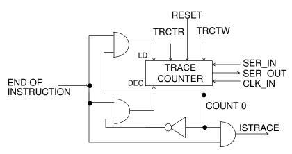
Figure 10-4 Trace Counter Logic
