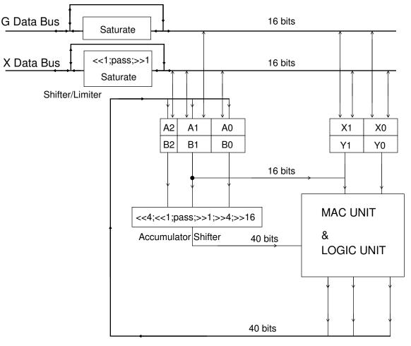
Figure 3-2 Data ALU Functional Block Diagram
