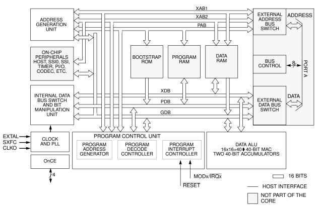
Figure 1-2 DSP56100 Family Core CPU Block Diagram
