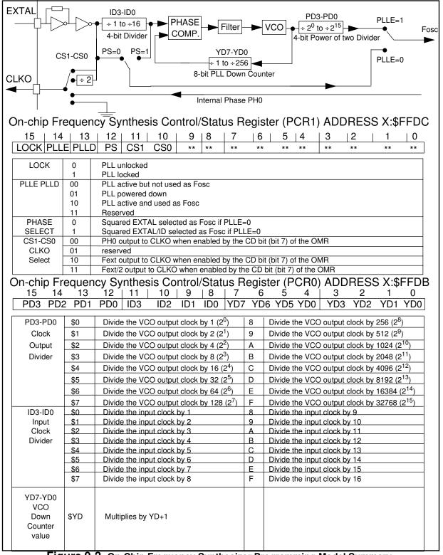
Figure 9-2 On-Chip Frequency Synthesizer Programming Model Summary.
