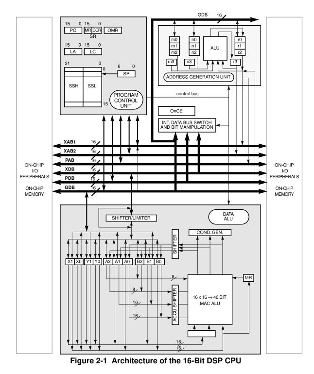
Address Registers are 16-bit registers which may contain address or data. Each Address Register may be output to the PAB and XAB1. R3 may be accessed for output to XAB2
