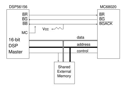
Figure 8-7 Bus Arbitration Between a DSP56156 and an MC68020
