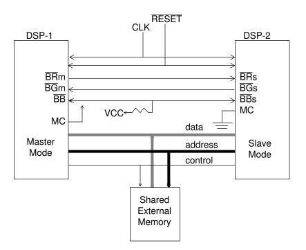
Figure 8-3 Bus Arbitration Between Two 16-bit DSPs
