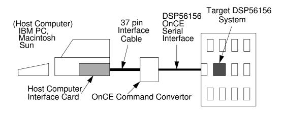
Figure 11-2 Target Circuit Emulation
