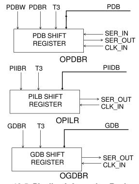
Figure 10-5 Pipeline Information Registers
