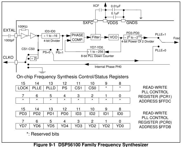
Block Diagram and Control Registers
