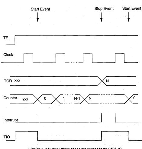
Figure 7-9 Pulse Width Measurement Mode (INV=1)
