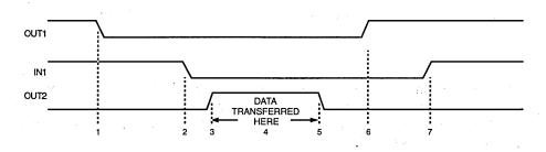
Figure 4-13 Two DSPs with External Bus Arbitration Timing
