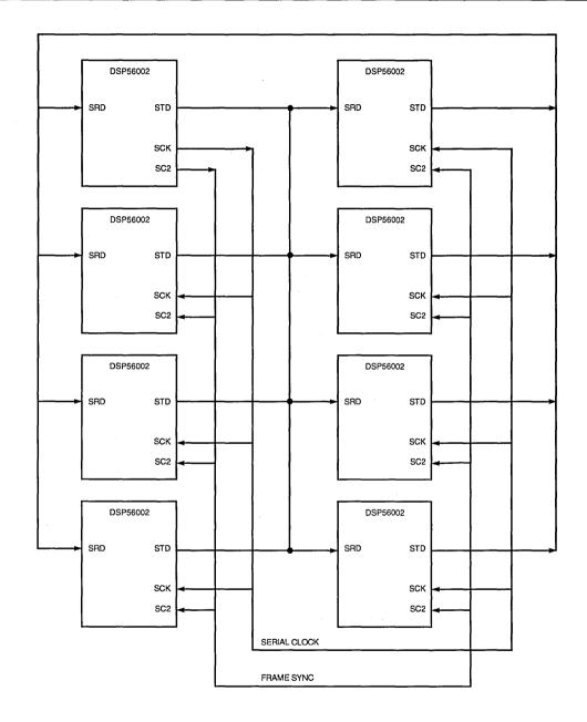
Figure 6-93 SSI TDM Connected Parallel Processing Array
