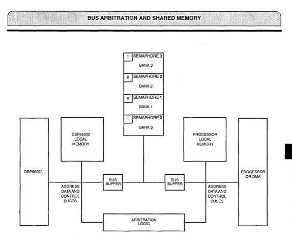
Figure 4-17 Signaling Using Semaphores
