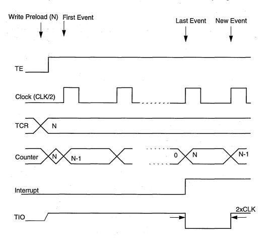
Figure 7-6 Standard Timer Mode, Internal Clock, Output Pulse Enabled (INV=1)
