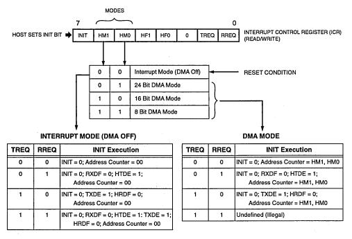
INIT is used by the HOST to force initialization of the HI hardware. The HI hardware automatically clears INIT when the command is executed. INIT is cleared by DSP RESET.
