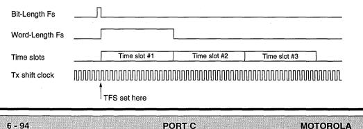
Data written to the transmit data register during the time slot when TFS is set will be transmitted (in network mode) during the second time slot in the frame. TFS is useful in network mode to identify the start of the frame. This is illustrated in a typical transmit interrupt handler:
