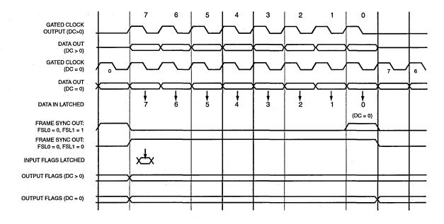
Figure 6-60 Internally Generated Clock Timing (8-Bit Example)
