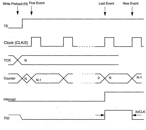
Figure 7-5 Standard Timer Mode, Internal Clock, Output Pulse Enabled (INV=0)
