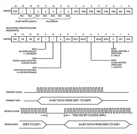
**NOTE:** Two SSI bit clock times are automatically inserted between each data word. This guarantees frame sync will be low between every data word transmitted and the clock will not be continuous for two consecutive data words.
