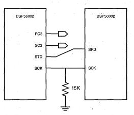
Figure 6-84 On-Demand Mode Example — Hardware Configuration
