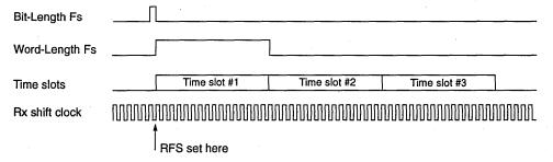
When RFS is clear and a word is received, it indicates (only in network mode) that the frame sync did not occur during reception of that word. RFS is useful in network mode to identify the start of the frame. This feature is illustrated in a typical receive interrupt handler:
