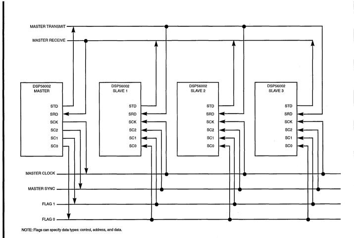
SYNCHRONOUS SERIAL INTERFACE (SSI)
