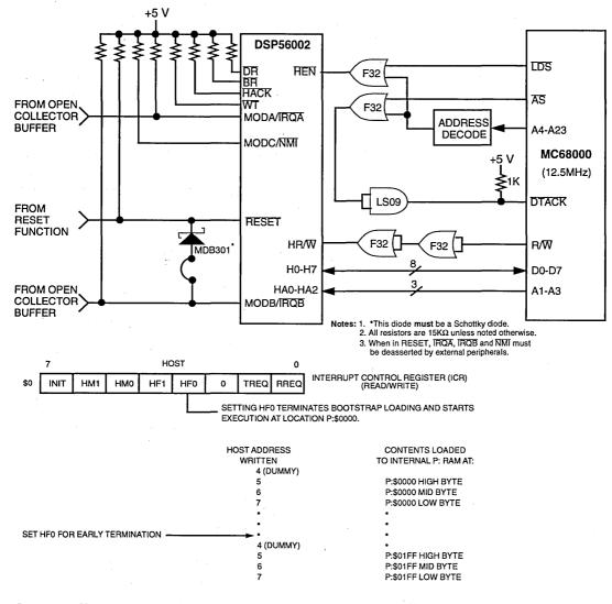
• Because the DSP56002 is so fast, host handshaking is generally not required.
