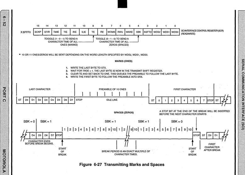
If TE remains cleared for a longer period, the output will remain high for an even number of character frames until TE is set. (4) Write the first byte to follow the preamble into SRX before the preamble is complete and resume normal transmission. Sending a break follows the same procedure except that instead of clearing TE, SBK is set in the SCR to send breaks and then reset to resume normal data transmission.
