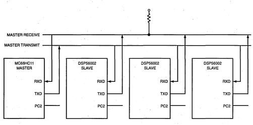
Figure 6-40 Master-Slave System Example
