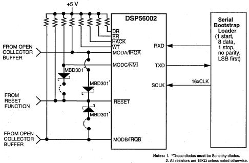
3. When in RESET, IRQA, IRQB and NMI must be deasserted by external peripherals.
