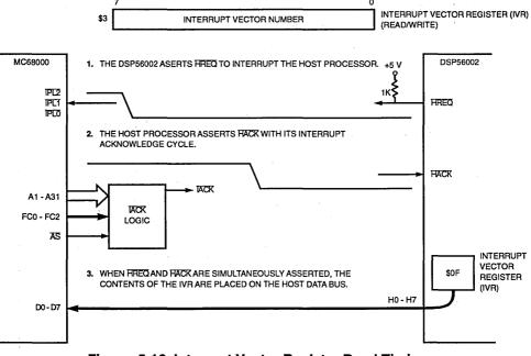
Figure 5-16 Interrupt Vector Register Read Timing
