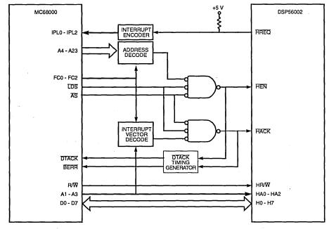
MC68000 — USE MOVEP for multiple byte transfers. MC68020 or MC68030 — Any Memory references will work due to dynamic bus sizing.
