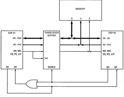
Figure 4-15 Bus Arbitration Using BR and BG, and WT and BS with No Overhead
