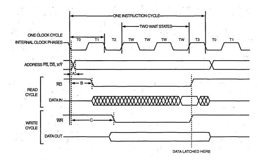
Figure 4-7 Port A Bus Operation with Two Wait States
