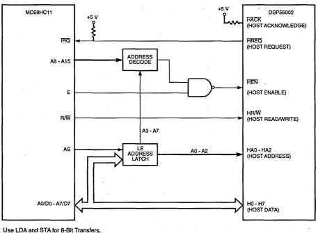
Use LDA and STA for 8-Bit Transfers. Use LDD and STD for 16-Bit Transfers.
