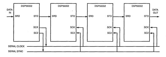
Figure 6-91 SSI Cascaded Multi-DSP System
