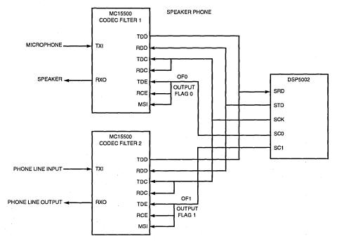
NOTE: SC0 and SC1 are output flag 0 and 1 used to software select either filter 1 or 2.
