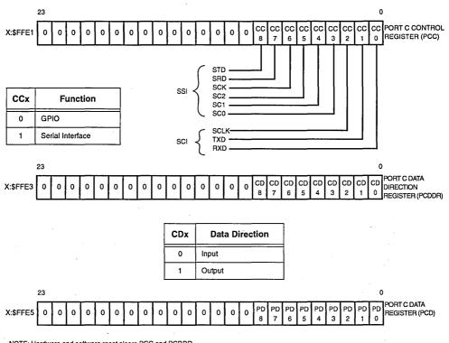
NOTE: Hardware and software reset clears PCC and PCDDR.
