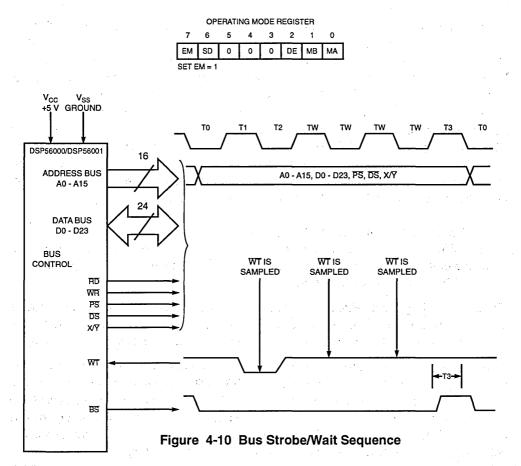
Adding wait states to external memory accesses can substantially reduce power requirements. Consult the *DSP56002 Technical Data Sheet* (DSP56002/D) for specific power consumption requirements.
