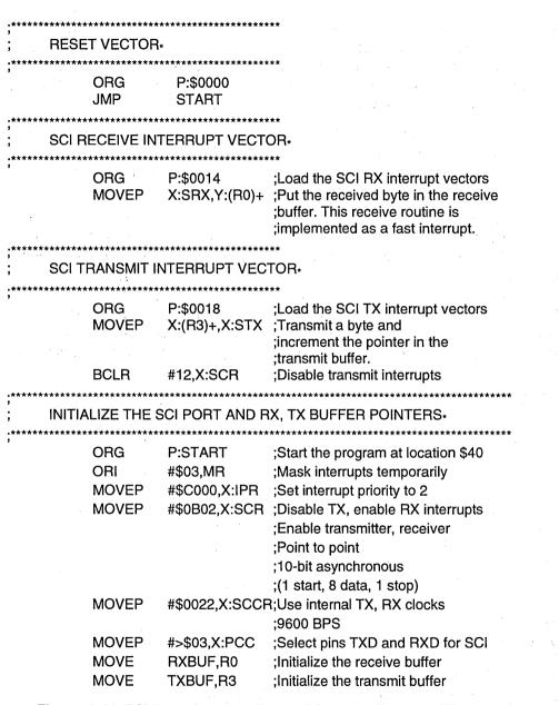
Figure 6-28 SCI Asynchronous Transmit/Receive Example (Sheet 2 of 3)
