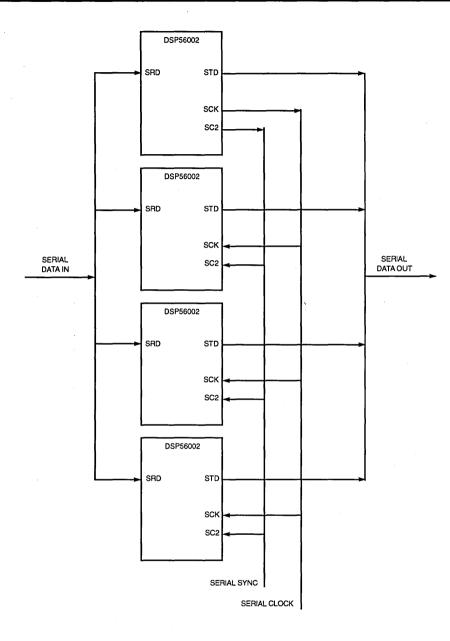
Figure 6-92 SSI TDM Parallel DSP Network
