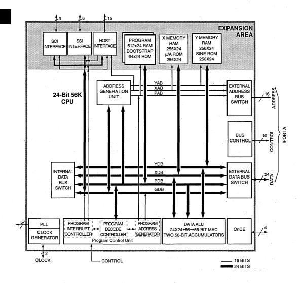
Figure 1-2 DSP56002 Block Diagram
