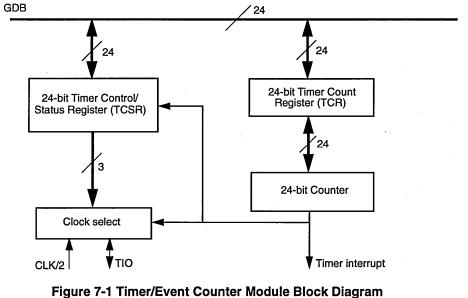
\* The first version of the DSP56002 (mask number D41G) did not have the timer/event counter. Later versions of the DSP56002 which have different mask numbers do have the timer/event counter. This mask number can be found below the part number on each chip.
