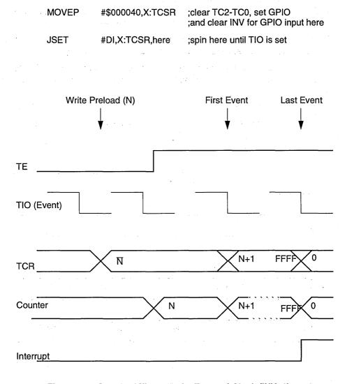
Figure 7-13 Standard Timer Mode, External Clock (INV=1)
