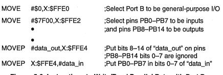
Figure 5-6 Instructions to Write/Read Parallel Data with Port B
