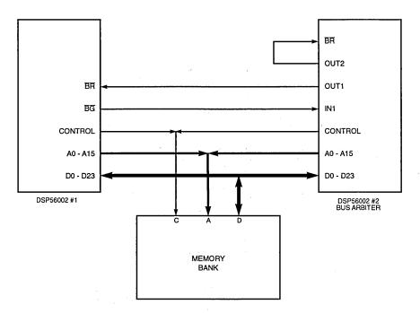
Figure 4-12 Bus Arbitration Using Only BR and BG with Internal Control
