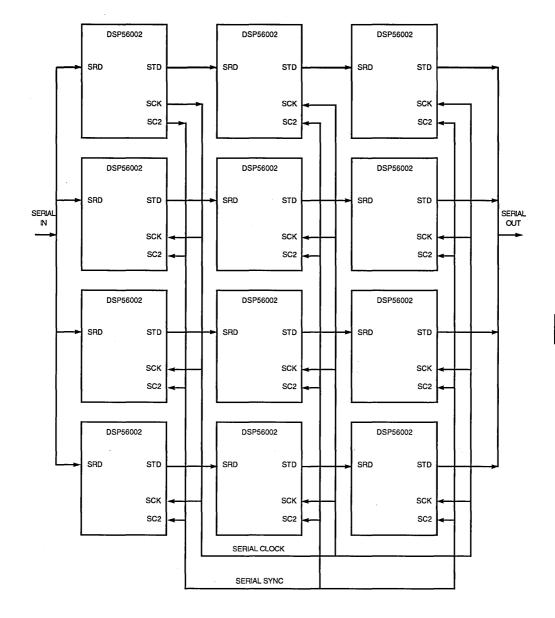
Figure 6-94 SSI TDM Serial/Parallel Processing Array
