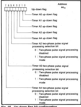
Fig. 16 Up-down flag bit configuration
