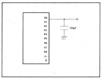
Fig. 1 Testing circuit for ports P0~P8,  $\phi_1$
