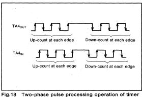
Fig.18 Two-phase pulse processing operation of timer A4
