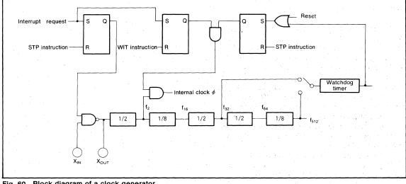
Block diagram of a clock generator Fig. 60
