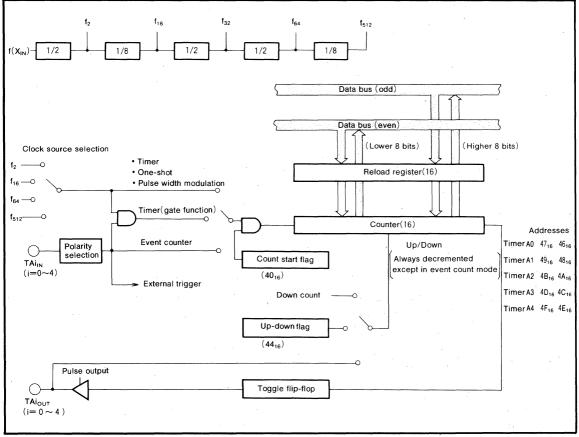
Fig. 11 Block diagram of timer A
