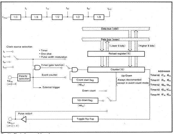
Fig. 11 Block diagram of timer A
