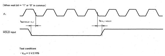
• Input timing voltage : V<sub>IL</sub>=1.0V, V<sub>IH</sub>=4.0V
