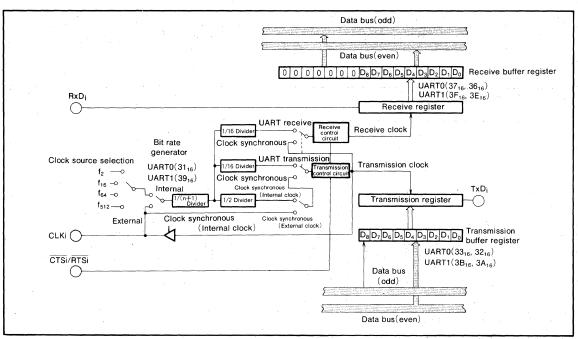
Fig. 38 Serial I/O port block diagram
