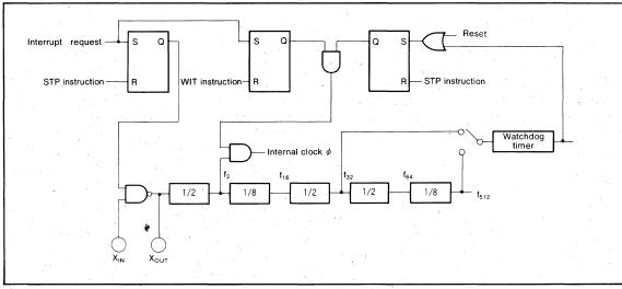
Fig. 55 Block diagram of a clock generator
