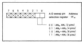
Fig. 50 A-D sweep pin selection register configuration
