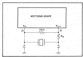
Fig. 56 Circuit using a ceramic resonator
