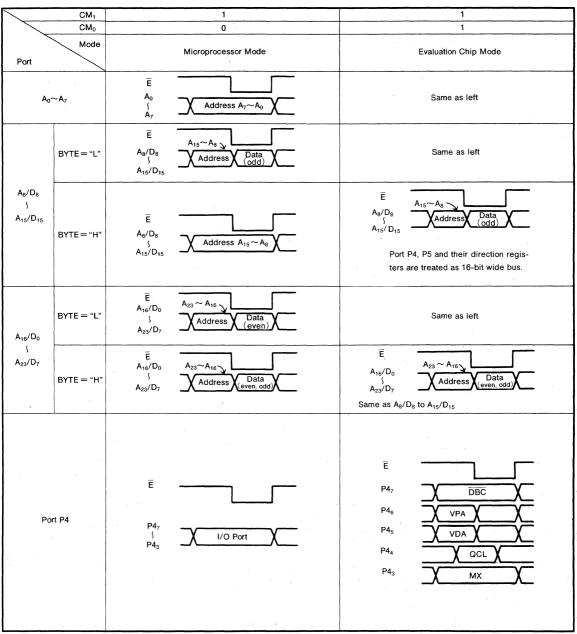
Fig. 54 Processor mode and A<sub>0</sub> to A<sub>7</sub> pins, A<sub>8</sub>/D<sub>8</sub> to A<sub>23</sub>/D<sub>7</sub> pins and port P4 functions
