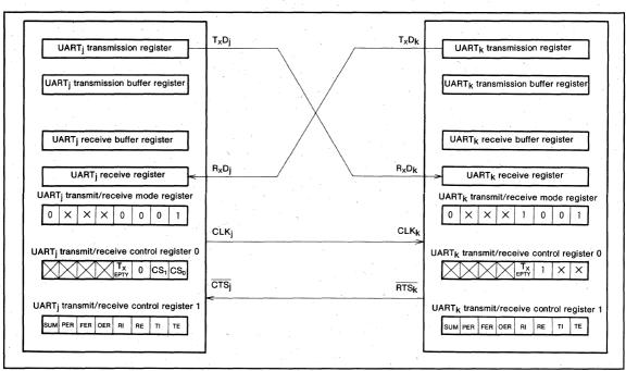
Fig.38 Clock synchronous serial communication
