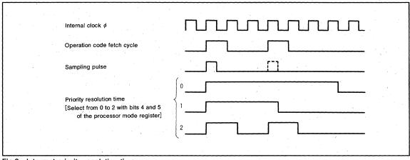
Fig.9 Interrupt priority resolution time
