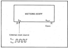
Fig. 57 External clock input circuit
