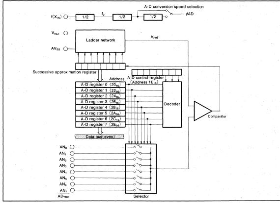
Fig.43 A-D converter block diagram
