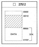
2) Address 0<sub>16</sub> to 10<sub>16</sub> are the area for storing the data on model designation and options. This area must be written with the data shown below. Details for option data are given next in the section describing the STP instruction option. Address and data are written in hexadecimal notation.
