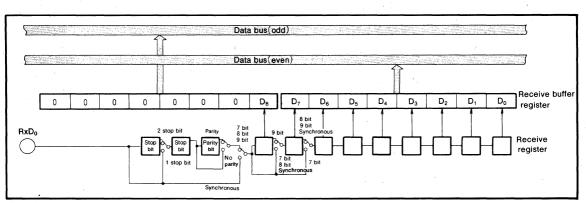
Fig. 40 Receiver block diagram
