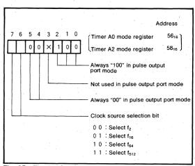
Fig. 35 Timer A0, A2 mode register bit configuration in pulse output port mode
