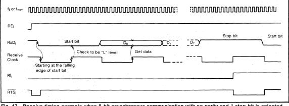
Receive timing example when 8-bit asynchronous communication with no parity and 1 stop bit is selected Fig. 47
