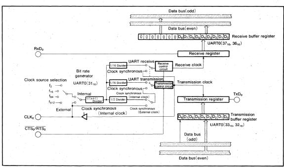
Fig. 38 Serial I/O port block diagram
