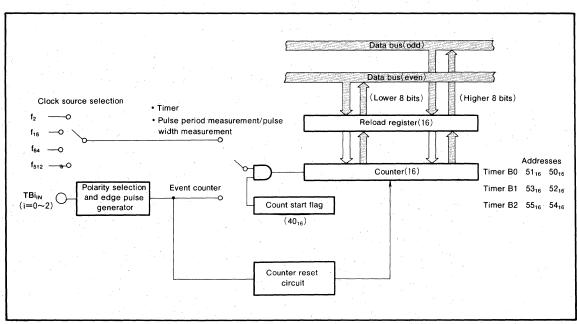
Fig. 27 Timer B block diagram
