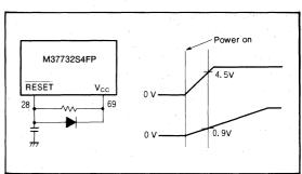
Fig. 54 Example of a reset circuit (perform careful evaluation at the system design level before using)
