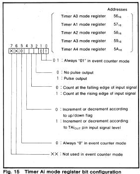
Timer Ai mode register bit configuration during event counter mode
