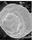
Fig.4 Au-Al plague formation on bonding pad
