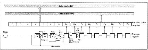
Fig. 40 Receiver block diagram
