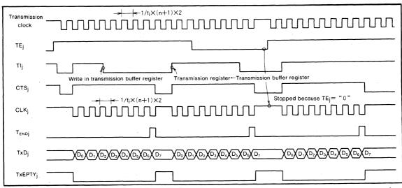
Fig. 44 Clock synchronous serial I/O timing
