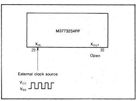
Fig. 62 External clock input circuit
