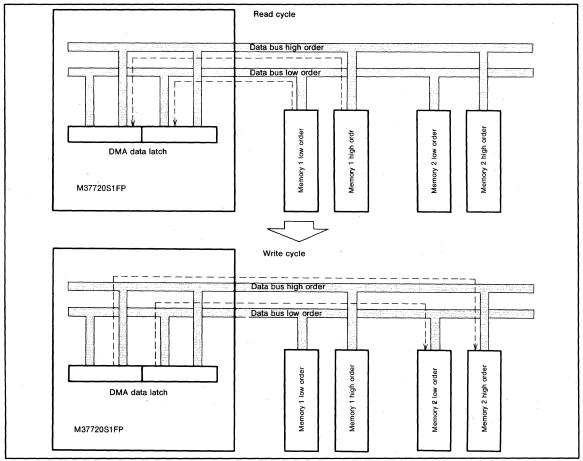
Fig.51 Two bus cycle transfer example
