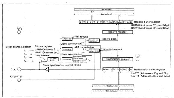
Fig.33 Serial I/O port block diagram
