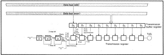
Fig. 41 Transmitter block diagram
