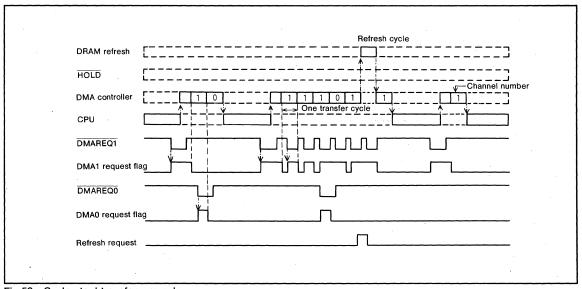
Fig.59 Cycle steal transfer example
