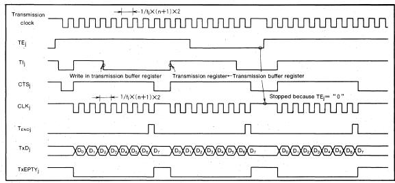
Fig. 44 Clock synchronous serial I/O timing
