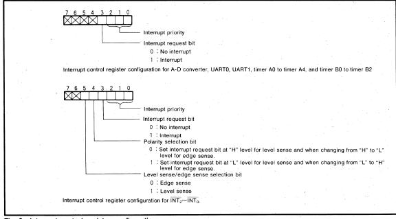
Fig. 6 Interrupt control register configuration
