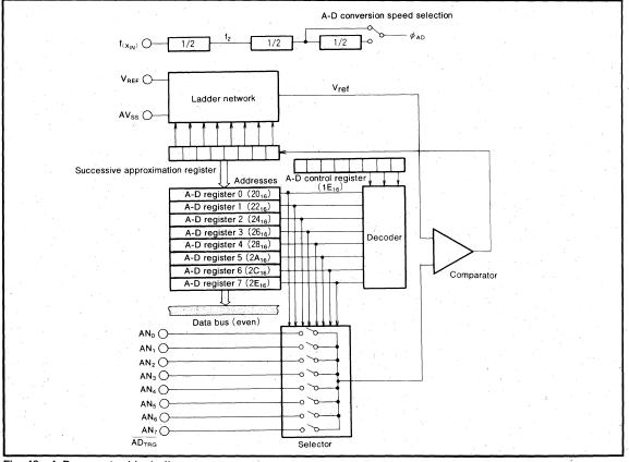
Fig. 43 A-D converter block diagram
