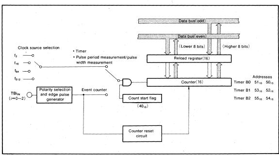
Fig. 27 Timer B block diagram
