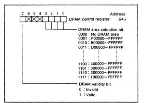
Fig.74 DRAM control register bit configuration
