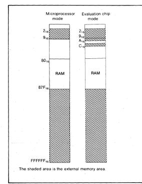
Fig. 58 External memory area for each processor mode
