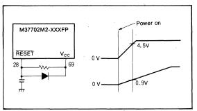
Fig. 49 Example of a reset circuit (perform careful evaluation at the system design level before using)
