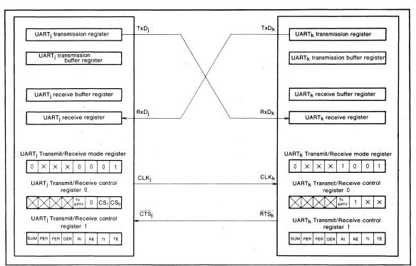
Fig. 43 Clock synchronous serial communication
