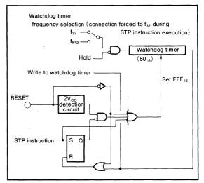
Fig. 51 Watchdog timer block diagram
