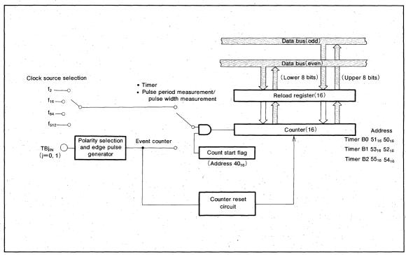
Fig.27 Timer B block diagram
