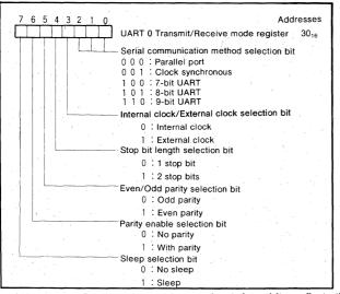
Fig. 39 UART 0 Transmit/Receive mode register bit configuration
