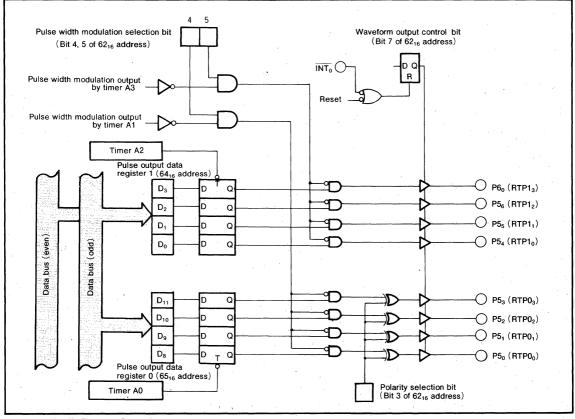
Fig. 33 Block diagram for pulse output port mode
