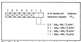
Fig. 45 A-D sweep pin selection register configuration
