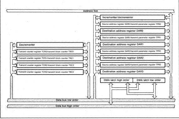
Fig.46 DMA controller block diagram
