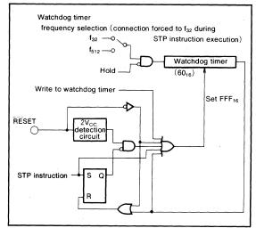
Fig. 48 Watchdog timer block diagram
