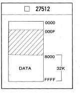
Address 0<sub>16</sub> to 0F<sub>16</sub> are the area for storing the data on model designation. This area must be written with the data shown below.
