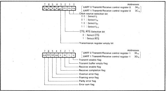
Fig. 42 UARTI Transmit/Receive control register bit configuration
