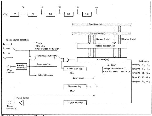
Fig. 11 Block diagram of timer A
