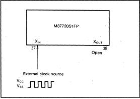
Fig.92 External clock input circuit
