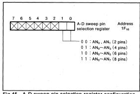
A-D sweep pin selection register configuration Fia.45
