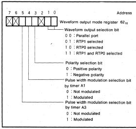
Fig. 34 Waveform output mode register bit configuration
