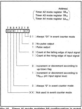
Fig.15 Timer Aj mode register bit configuration in event counter mode
