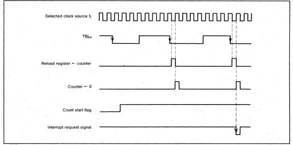
Fig.31 Pulse period measurement mode operation
