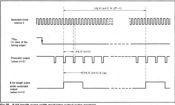
Fig.26 8-bit length pulse width modulator output pulse example
