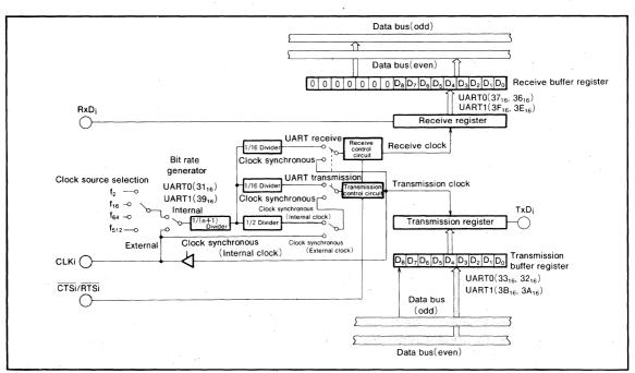
Fig. 33 Serial I/O port block diagram
