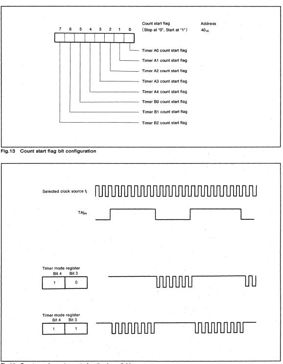
Fig.14 Count waveform when gate function is available
