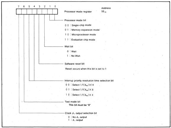
Fig. 51 Processor mode register bit configulation
