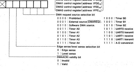
Fig.49 DMAi controll register bit configuration
