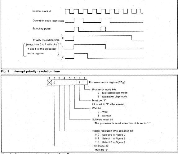
Fig. 10 Processor mode register configuration
