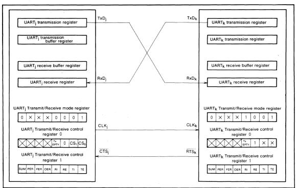
Fig. 43 Clock synchronous serial communication
