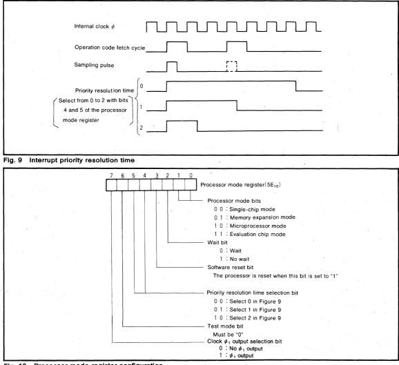
Fig. 10 Processor mode register configuration
