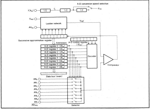
Fig. 48 A-D converter block diagram
