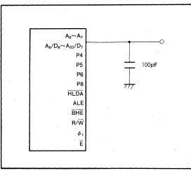
Fig. 60 Testing circuit for each terminal
