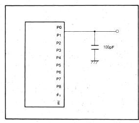
Fig. 1 Testing circuit for ports P0~P8,  $\phi_1$
