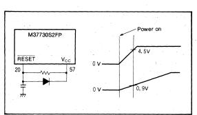
Fig. 51 Example of a reset circuit (perform careful evaluation at the system design level before using)
