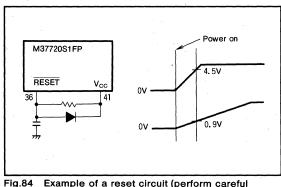
Fig.84 Example of a reset circuit (perform careful evaluation at the system design before using)
