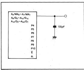
Fig.93 Testing circuit for ports
