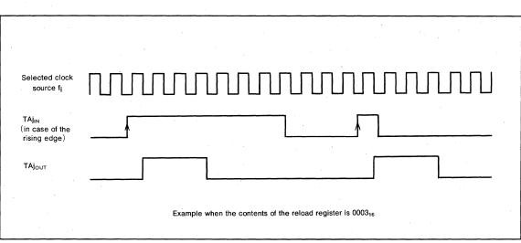
Fig.22 Pulse output example when external rising edge is selected
