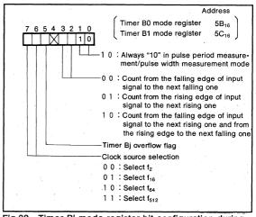
Fig.30 Timer Bj mode register bit configuration during pulse period measurement/pulse width measurement mode
