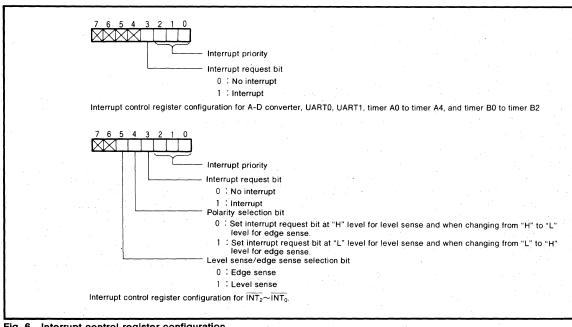
Fig. 6 Interrupt control register configuration
