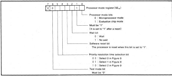
Fig. 10 Processor mode register configuration
