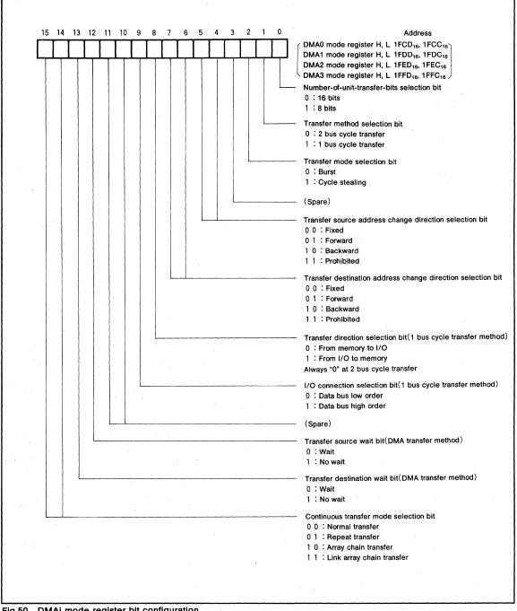
DMAi mode register bit configuration Fig.50
