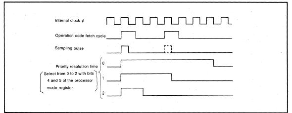
Fig. 9 Interrupt priority resolution time
