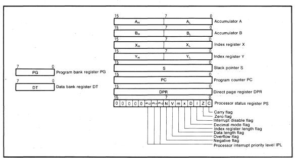
Fig. 3 Register structure
