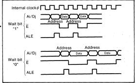
Fig. 59 Relationship between wait bit and access time
