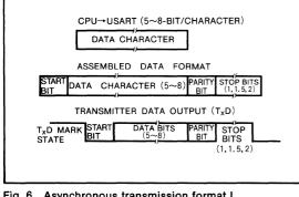
Fig. 6 Asynchronous transmission format I (transmission)
