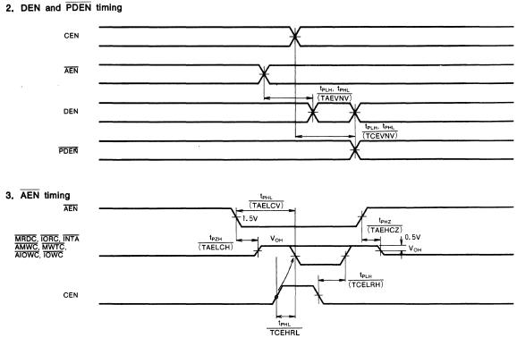
Note 6 : CEN must be low or valid prior to  $T_2$  to prevent the command from being generated.
