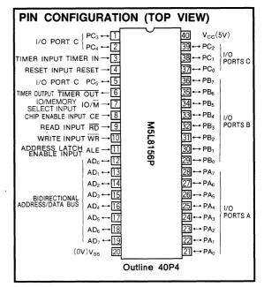
shake mode. The counter/timer is composed of 14-bit down counter (events or time) and it can generate square wave pulses that can be used for counting and timing.
