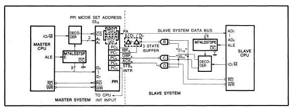
Fig. 13 A circuit for an application using mode 2
