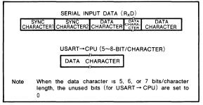
Fig. 9 Synchronous transmission format II (reception)
