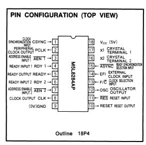
The frequency/crystal selection input  $F/\overline{C}$  can be used to select the crystal oscillator circuit output or an external clock input as the input for the divide-by-three counter.
