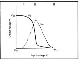
Fig. 3 Single-stage inverter voltage transfer and supply current vs. input voltage characteristics
