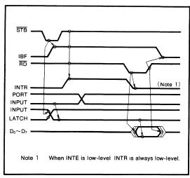
Fig. 4 Timing diagram
