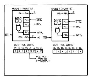
Fig. 3 An example of mode 1 input state
