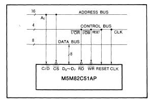
Fig. 1 M5M82C51AP interface to CPU system bus
