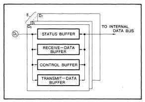
Fig. 2 Data-bus-buffer structure
