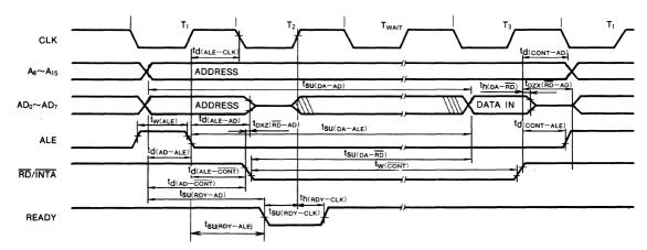
Note : READY must remain stable during setup and hold times
