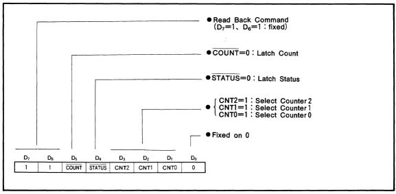
Fig. 8 Read Back Command Format
