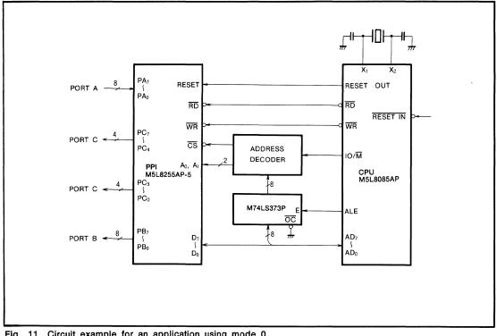
Fig. 11 Circuit example for an application using mode 0.
