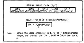
Fig. 9 Synchronous transmission format II (reception)
