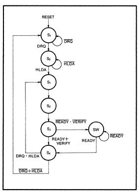
Fig. 1 DMA Operation state transition diagram
