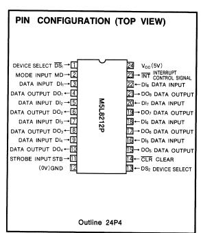
When MD is high, the data in the data latches is transferred to the data outputs. When  $\overline{\text{DS}_1}$  is low and  $\text{DS}_2$  is high, the data inputs are latched in the data latches. The low-level clear input  $\overline{\text{CLR}}$  resets the data latches and sets the service request flip-flop SR, but the state of the output buffers is not changed.
