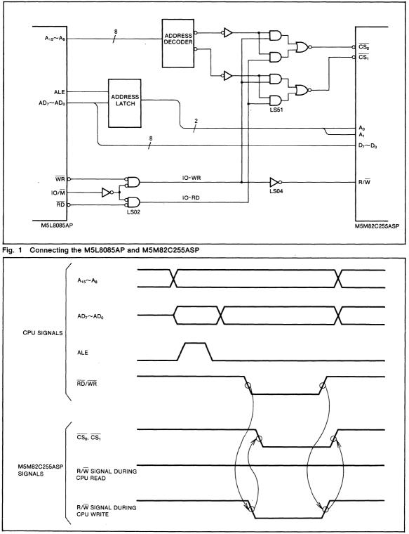
Fig. 2 Timing Diagram
