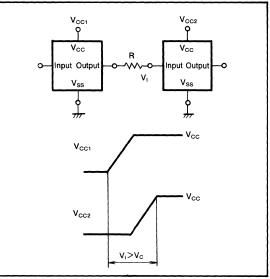
Fig. 12 Preventing latchup when dual power supplies are used
