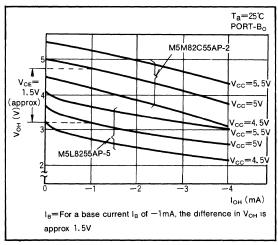
Fig. 16 M5L8255AP-5/M5M82C55AP-2 V<sub>OH</sub> output characteristics comparison
