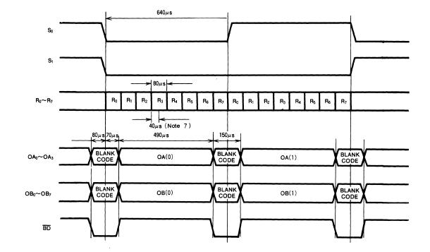
DISPLAY (This example is encoded display, left entry mode with internal clock cycle 10µ sec. Scan timing output S<sub>2</sub>, S<sub>3</sub> are not shown.)
