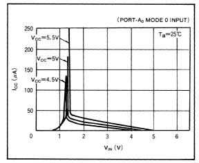
Fig. 4 Input voltage vs. dissipation current M5M82C55AP-2
