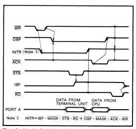
Fig. 9 Mode 2 timing diagram
