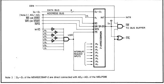
Fig. 7 Example of interface with the MELPS86
