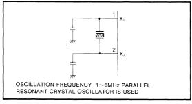
Fig. 7 Connections when crystal is used for  $X_1$  and  $X_2$  inputs
