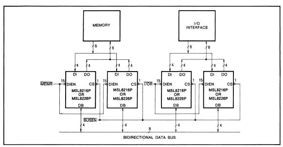
Fig. 2 Memory and I/O interface to bidirectional data bus
