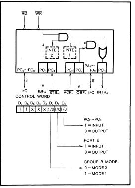
Fig. 10 An example of mode 2 operation
