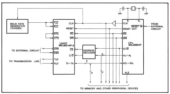
Fig. 11 Example of circuit using the asynchronous mode
