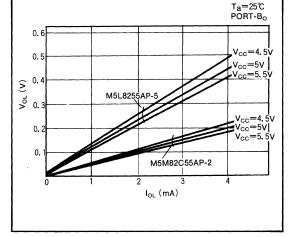
Fig. 17 M5L8255AP-5/M5M82C55AP-2 V<sub>OL</sub> output characteristics comparison
