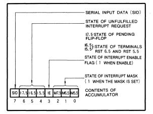
Fig. 9 Relation of the instruction RIM with the accumulator
