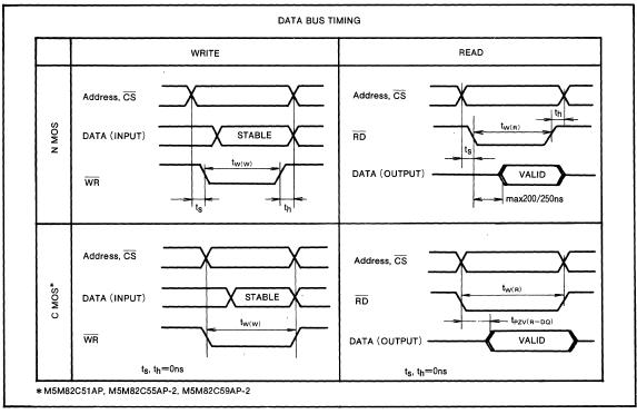
Fig. 11 Bus timing characteristics
