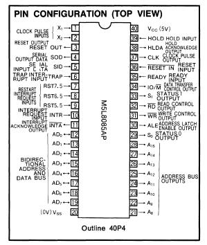
rupt signals are synchronized with the clock pulse. For simple serial data transfer it provides both a serial input data (SID) line and a serial output data (SOD) line. It also has three maskable restart interrupts and one non-maskable trap interrupt.
