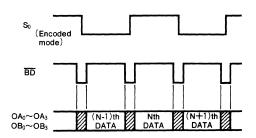
Note 5 : Values of the output data shown in the slanted line areas are decided upon the clear command executed last to become the value of the display RAM after the reset. The values in the slanted areas after reset will go low-level. In the same manner, the values OA<sub>0</sub>~OA<sub>3</sub>, OB<sub>0</sub>~OB<sub>3</sub> are dependent on the clear command executed last. When the both A and B are blanked, the signal BD will be in low-level.
