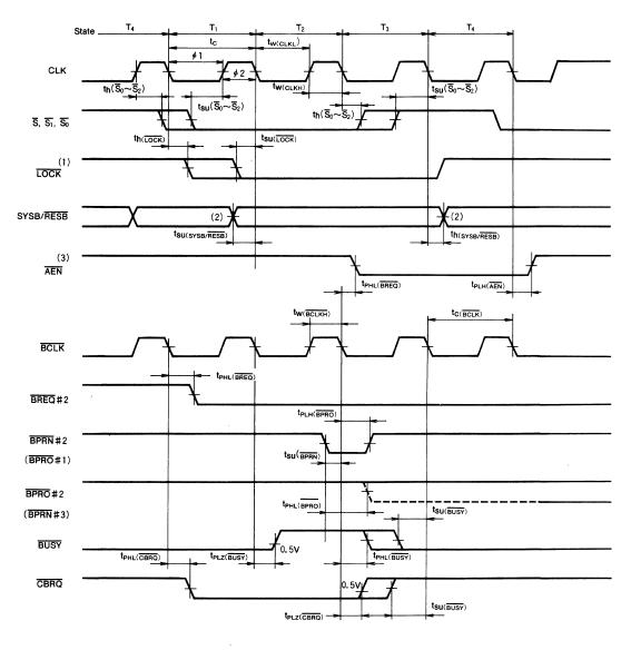
Note 1 : LOCK can be active during any state as long as the relation ships shown above with the respect to CLK are maintained.
