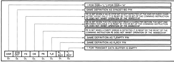
Fig. 10 Status information  $C/\overline{D} = "H"$ ,  $\overline{RD} = "L"$ )
