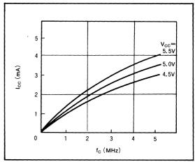
Fig. 6 Operating frequency vs. power dissipation M5M82C37AP-5
