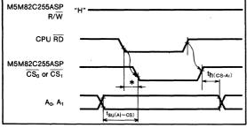
Fig. 3 Read operation of the M5M82C255ASP
