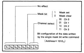
Fig.5 Mask register (write single bit)
