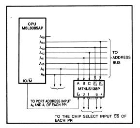
Fig. 15 PPI address decoding (case 2)
