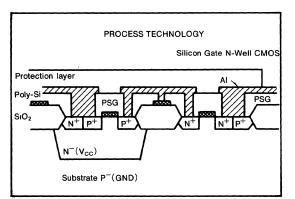
Fig. 1 Single-stage inverter construction
