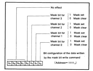
Fig.4 Mask register (write all bit)
