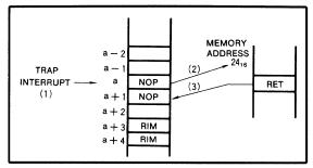
Fig. 2 TRAP interrupt processing
