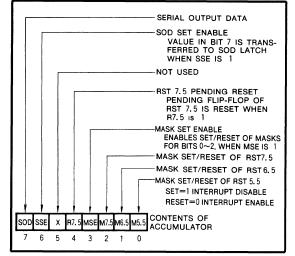
Fig. 10 Relation of the SIM instruction with the accumulator
