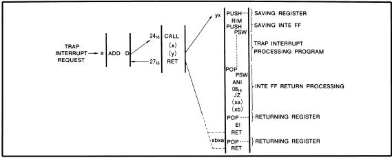
Fig. 4 TRAP interrupt processing routine
