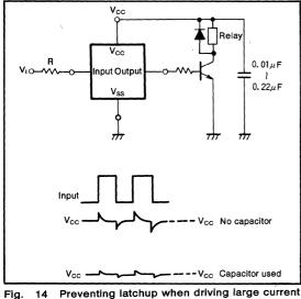
Fig. 14 Preventing latchup when driving large curren circuits
