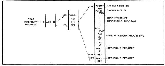
Fig. 4 TRAP interrupt processing routine
