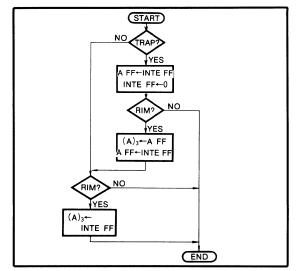
Fig.3 TRAP interrupt and INTE FF processing
