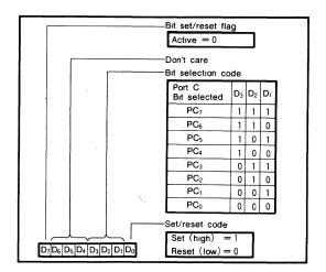
Fig. 1 Control word format for port C set/reset
