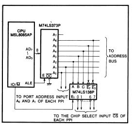
Fig. 14 PPI address decoding (case 1)
