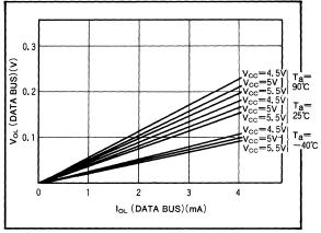
Fig. 9 IoL-VoL characteristics M5M82C55AP-2
