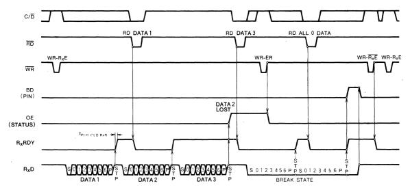
Note 15: Example format= 7 bits/character with parity & 2 stop bits
