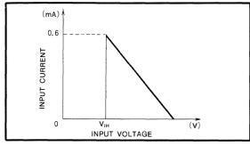
Fig. 6 RESET IN input current vs input voltage
