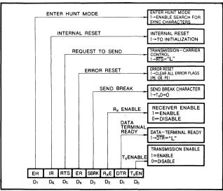
Fig. 5 Command-instruction format  $(C/\overline{D} = "H" \quad \overline{WR} = "L")$
