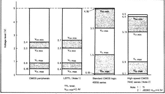
Fig. 7 DC noise margin comparison ( $V_{CC}$ =5.0V)
