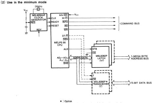
Required when the number of devices driving the bus increases
