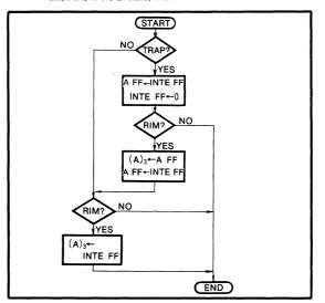
Fig.3 TRAP interrupt and INTE FF processing
