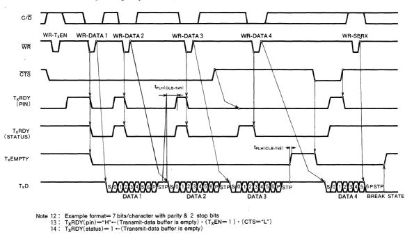
Transmitter Control & Flag Timing (Async Mode)
