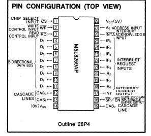
and priority will output an INT to the CPU. After that, when an INTA signal is received from the CPU or the system controller, a CALL instruction and a programmed vector address is released onto the data bus.
