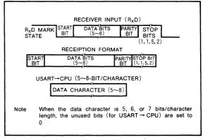
Fig. 7 Asynchronous transmission format II (reception)
