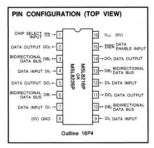
The terminal DIEN controls the data flow. The data flow control is performed by placing one of a pair of buffers in high-impedance state and allowing the other to transfer the data.
