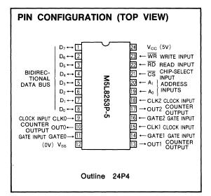
hardware triggered strobe. The count can be monitored and set at any time. The counter operates with either the binary or BCD system.
