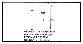
Fig. 5 Connections when crystal is used for  $X_1$  and  $X_2$  inputs
