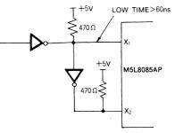
Pullup resistors are required to assure that the high level voltage of the input is at least 4V
