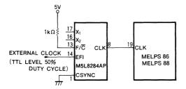
The frequency should be three times the CPU cycle frequency
