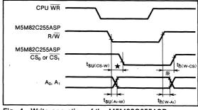
Fig. 4 Write operation of the M5M82C255ASP
