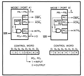
Fig. 5 An example of mode 1 output state
