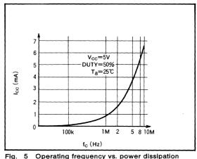
Fig. 5 Operating frequency vs. power dissipation M5M82C54P
