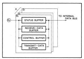
Fig. 2 Data-bus buffer structure
