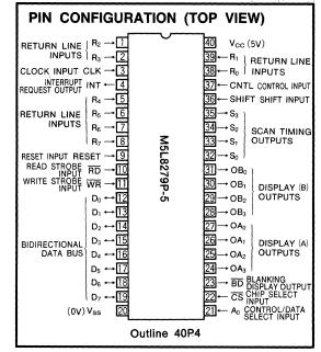
debounce buffer and an  $8 \times 8$ -bit FIFO/SENSOR RAM. It operates in any one of the scanned keyboard mode, scanned sensor matrix mode or strobed entry mode. The display portion is provided with a 16  $\times$  8-bit display RAM that can be organized into a dual 16 $\times$  4 configuration. Also, an 8-digit display configuration is possible by means of programming.
