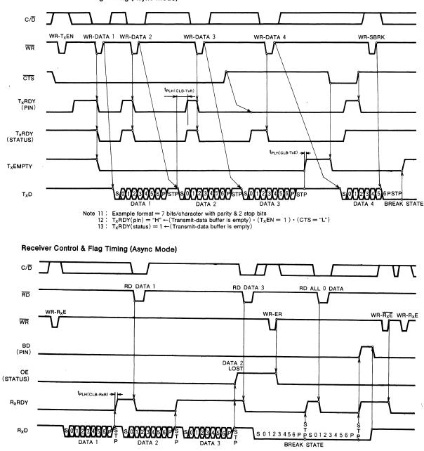
Transmitter Control & Flag Timing (Async Mode)
