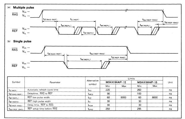
Fig. 1.40 Automatic refresh timing
