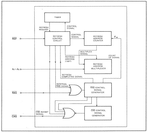
Fig..1.27 Refresh circuit block diagram
