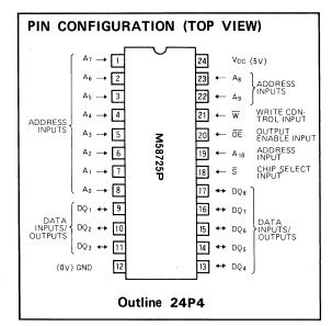
During a read cycle, when a location is designated by address signals  $A_0 \sim A_{10}$  the  $\overline{OE}$  signal is kept low to keep the DQ terminals in the output mode, signal  $\overline{W}$  goes high, and the data of the designated address is available at the I/O terminals.
