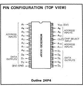
to the address inputs  $(A_0 \sim A_{12})$  make the data contents of the designated address location available at the data input/output  $(D_0 \sim D_7)$ .
