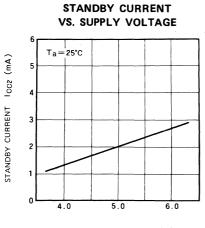
SUPPLY VOLTAGE  $V_{CC}(V)$
