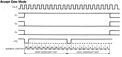
Note 3: The address is designated by two one-of-ten-coded digits. The figure shows designation of the address 99.
