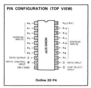
When  $\overline{S}$  is high, the chip is in the non-selectable state, disabling both reading and writing. In this case the output is in the floating (high-impedance) state, useful for OR-ties with other devices.
