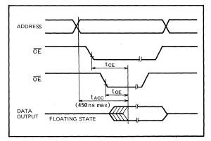
Fig. 3.7 Read timing diagram
