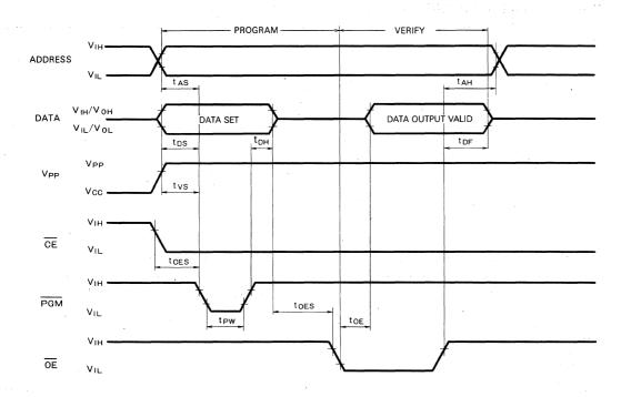
Test conditions for A.C. characteristics Input rise and fall time:  $\leq 20$ ns Input voltage: V<sub>IL</sub> = 0.45V, V<sub>IH</sub> = 2.4V Reference voltage at timing measurement: Input 1V and 2V Outputs 0.8V and 2V
