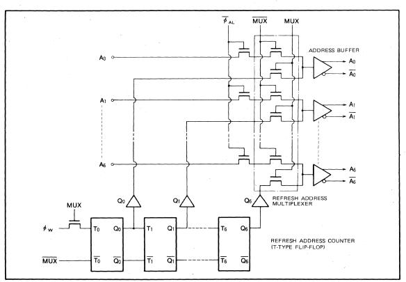
Fig. 1.28 Refresh address counter and multiplexer circuits
