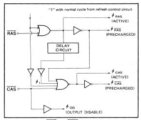
Fig. 1.12 Internal RAS and CAS clock generating circuit
