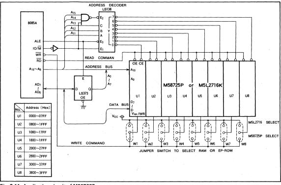
Fig. 2.11 Application circuit of M58725P
