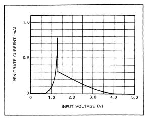
Fig. 2.17 Penitrate current of CMOS inverter
