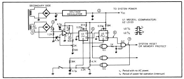
Fig. 2.21 Power-fail-detect circuit
