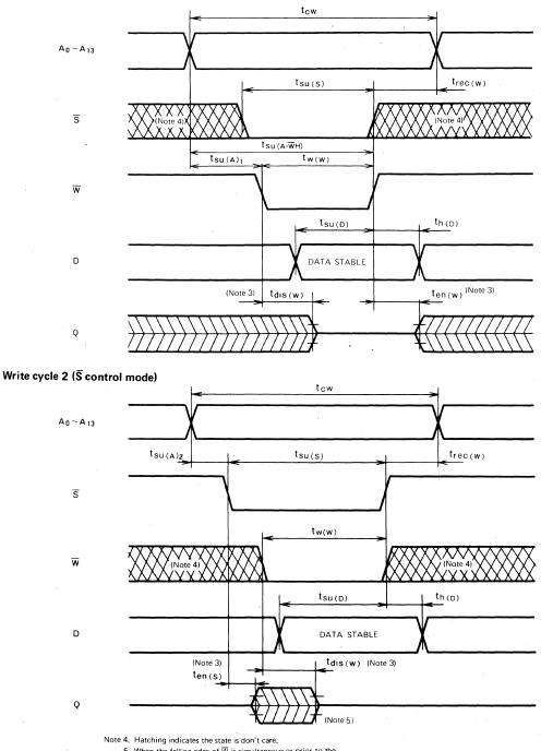
5. When the falling edge of  $\overline{W}$  is simultaneous or prior to the falling edge of  $\overline{S}$ , the output is maintained in the high impedance.
