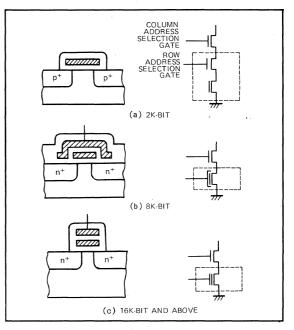
Fig. 3.1 Memory transistor construction
