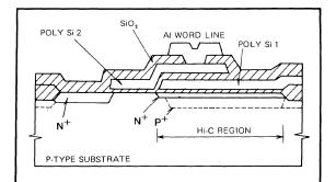
Fig. 1.1 Hi-C structure memory cell cross-section
