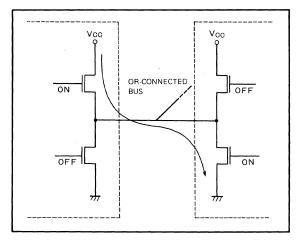
Fig. 3.6 Fighting for an OR-connected bus
