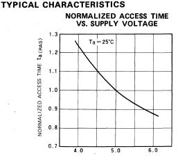
SUPPLY VOLTAGE  $V_{CC}$  (V)
