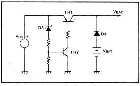
Fig. 2.23 Transistor-coupled switching circuit
