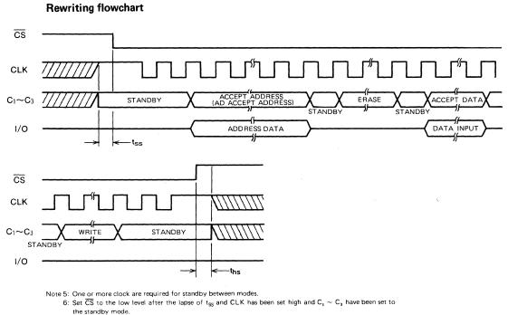
7: Keep CLK to the high level and  $C_1 \sim C_3$  to "standby" from the time when  $\overline{CS}$  is set high to the lapse of the
