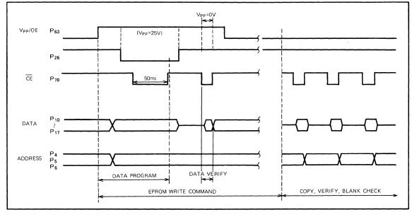
Fig. 3.14 2732 Programming timing
