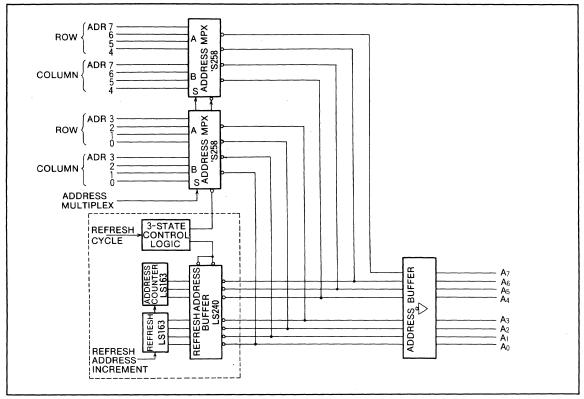
Fig. 1.41 Address multiplexer and refresh address counter
