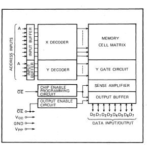
Fig. 3.5 EPROM Block diagram
