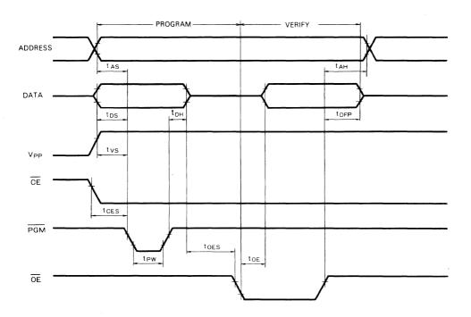
Test conditions for A.C. characteristics Input rise and fall time:  $\leq$ 20ns Input voltage:  $V_{IL}$  = 0.45V,  $V_{IH}$  = 2.4V Reference voltage at timing measurement: Input 0.8V and 2V Outputs 0.8V and 2V
