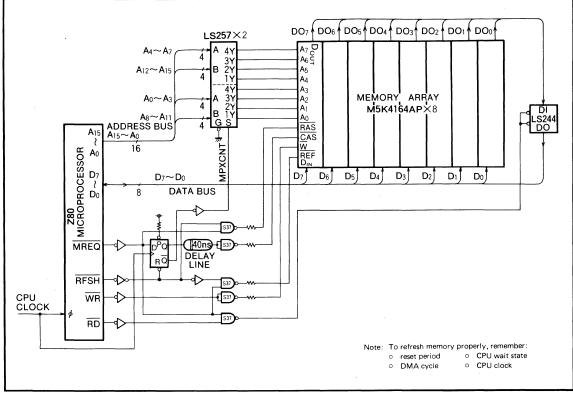
Fig. 1.50 Design example of microprocessor interface (Synchronous)
