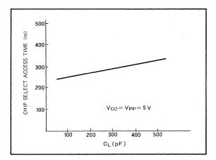
Fig. 3.9 2716 Chip select access time load capacitance dependency
