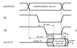
Output Load: 1 TTL gate, CL = 100pF
