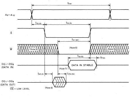
Note 4: Test conditions Input pulse level: 0,4 ~ 2,4V Input pulse risetime and falltime: 10ns Load: 1TTL, CL = 100pF Reference level: 1.5V Note 5: Hatching indicates the don't care inputs.
