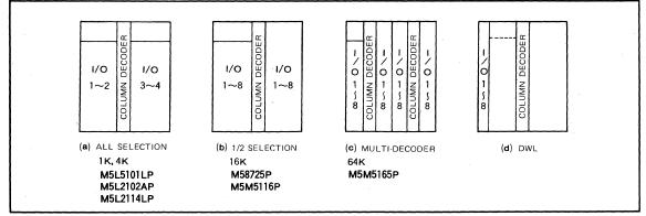
Fig. 2.2 Examples of memory cell array
