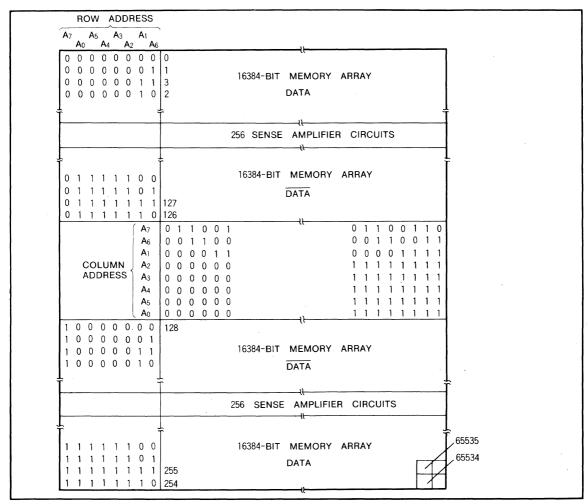
Fig. 1.35 Address decoder location
