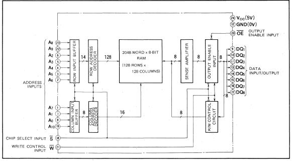
Fig. 2.5 Block diagram of M58725P
