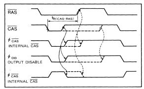
Fig. 1.15 Relationship of RAS and CAS rising edges to internal clock timing
