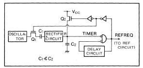
Fig. 1.29 Timer circuit block diagram
