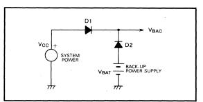
Fig. 2.22 Diode-coupled switching circuit
