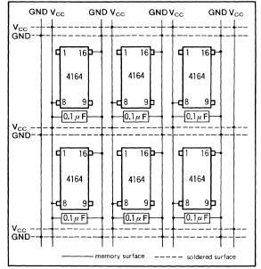
Fig. 1.39 (a) Gridded power distribution and decoupling capacitors
