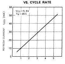
CYCLE RATE  $1/t_{CR}$  (MHz)
