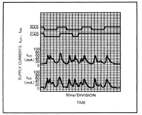
Fig. 1.37 Supply current vs time RAS/CAS cycle RAS-only cycle
