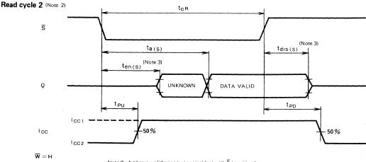
Note 2. Addresses valid prior to or coincident with  $\overline{S}$  transition low. 3. Transition is measured ±500mV from steady state voltage with specified loading in Figure 2.
