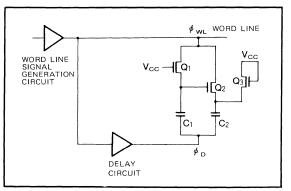
Fig. 1.6 Bootstrapped word line voltage generation circuit
