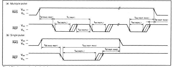
Fig. 1.31 Automatic refresh timing
