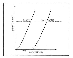
Fig. 3.2 Variation in memory transistor threshold voltage (V<sub>GO</sub>: Read gate voltage, both vertical and horizontal scales are arbitrary)
