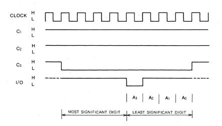
Note 3: In the AD accept address mode, the higher four are set high, and the lower four digits are designated by one of the four coded digits. This address mode allows designation of addresses from A<sub>0</sub> to A<sub>3</sub>. Each address has a 16 bits. The above figure shows designation of address A<sub>3</sub>.
