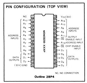
When the  $\overline{\text{CE}}$  or  $\overline{\text{OE}}$  signal is high, data output are in a floating state.
