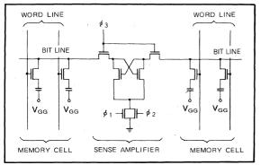
Fig. 1.8 Sense amplifier circuit
