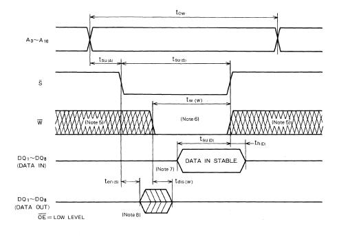
Note 4: Test conditions  $\label{eq:loss} \begin{array}{l} \mbox{Input pulse level: } 0.4 \sim 2.4 \mbox{V} \\ \mbox{Input pulse risetime and falltime: 10ns} \\ \mbox{Load: 1TTL, } C_L = 100 \mbox{P} \\ \mbox{Reference level: } 1.5 \mbox{V} \end{array}$
