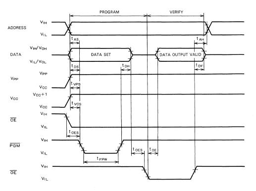
Test conditions for A.C. characteristics Input voltage:  $v_{IL}\!=\!0.45V, \, v_{IH}\!=\!2.4V$  Input rise and fall times:  $\leq\!20ns$  Reference voltage at timing measurement: Input 1V and 2V Output 0.8V, and 2V
