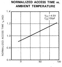
AMBIENT TEMPERATURE  $T_{a}\left(^{\circ}C\right)$
