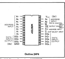
Fig. 2.6 Pin configuration of M58725P
