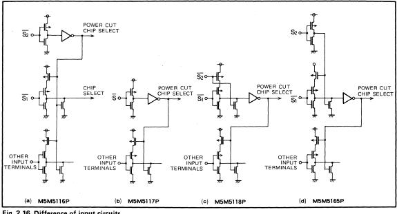
Fig. 2.16 Difference of input circuits
