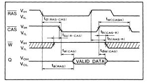
Fig. 1.19 Read cycle timing
