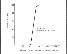
Fig. 3.10 Erasure characteristics example for 2716 and 2732
