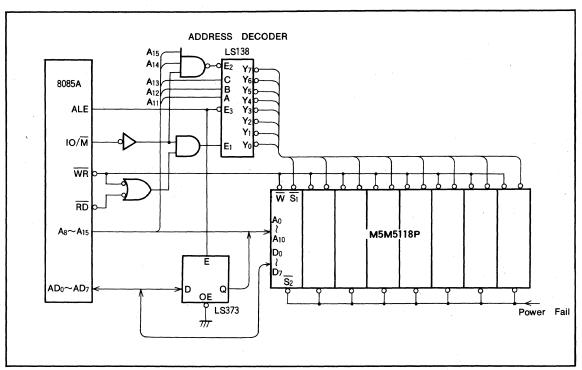
Fig. 2.14 Circuit diagram for preventing data bus contention (Application circuit of M5M5118P)
