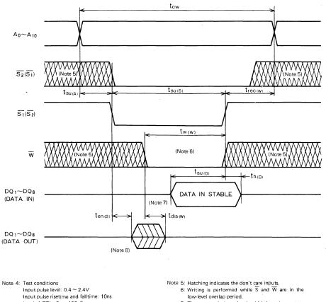
Load: 1 TTL, C<sub>L</sub> = 100pF Reference level: 1.5V
