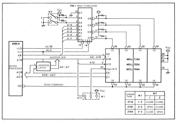
Fig. 3.11 Microprocessor-EPROM interface example
