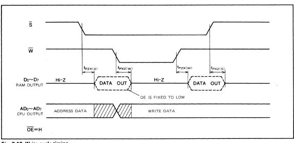
Fig. 2.12 Write cycle timing
