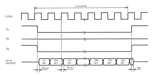
The 1st bit of output data is output after access time of  $t_{a(C)}$  from the mode control transition. And other bits are output after  $t_{a(C)}$  from positive edge of clock.
