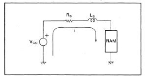
Fig. 1.38 (a) PC board trace equivalent circuit
