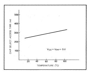
Fig. 3.8 2716 Chip select access time temperature characteristics example
