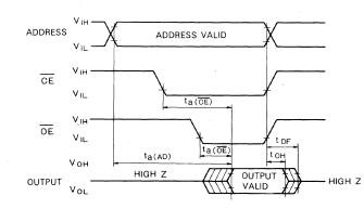
Test conditions for A.C. characteristics Input voltage: VIL = 0.45V, VIH = 2.4V Input rise and fall times:  $\leqq 20ns$  Reference voltage at timing measurement: Inputs 1V and 2V Output 0.8V, and 2V
