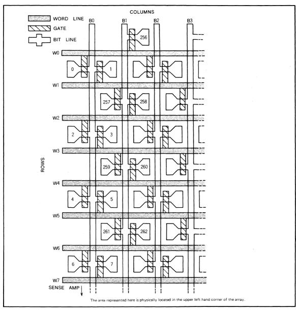
Fig. 1.36 Simplified internal bit topology
