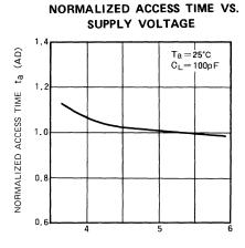
SUPPLY VOLTAGE  $V_{CC}$  (V)
