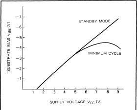
Fig. 1.3 Substrate bias vs supply voltage
