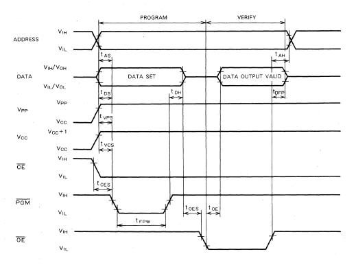
Test conditions for A.C. characteristics Input voltage:  $v_{IL}$  = 0.45V,  $v_{IH}$  = 2.4V Input rise and fall times:  $\leq 20$ ns Reference voltage at timing measurement: Input 0.8V and 2V Output 0.8V, and 2V
