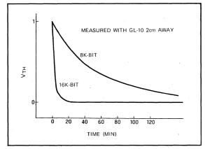
Fig. 3.4 Variation in V<sub>TH</sub> with erasure time
