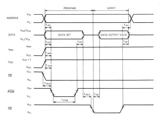
Test conditions for A.C. characteristics I lnput voltage:  $V_{IL}$  =0.8V,  $V_{IH}$  =2.2V lnput rise and fall times:  $\leq 20 ns$  Reference voltage at timing measurement: Input 1V and 2V Output 0.8V, and 2V
