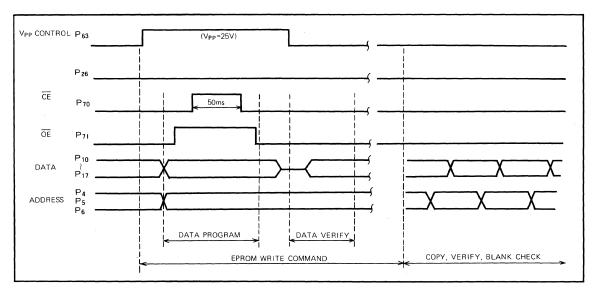
Fig. 3.13 2716 Programming timing
