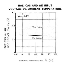
RAS, CAS AND WE INPUT **VOLTAGE VS. AMBIENT TEMPERATURE** 3.0 V<sub>CC</sub>=4.5V INPUT VOLTAGE VIH, VIL (V) 2.0 RAS, CAS AND WE ViH (min.) 1.0 ViL (max.) 0 60 100 - 20 0 20 40 80
