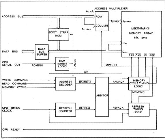
Fig. 1.46 Block diagram of the design example (Ansynchronous)
