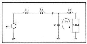
Fig. 1.38 (b) PC board trace equivalent circuit with decoupling capacitors
