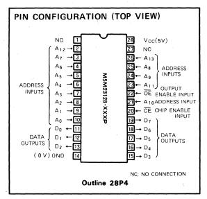
When the  $\overrightarrow{\text{CE}}$  or  $\overrightarrow{\text{OE}}$  signal is high, data output are in a floating state.
