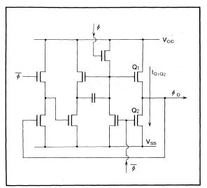
Fig. 1.4 Driver circuit
