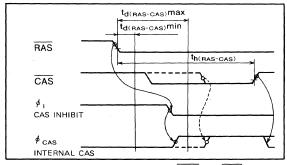
Fig. 1.14 The timing relationship of RAS and CAS falling edges to internal clock signals (gated CAS operation)
