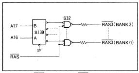
Fig. 1.42 (b) RAS decoder using REF pin
