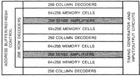
Fig. 1.9 M5K4164AP Chip arrangement
