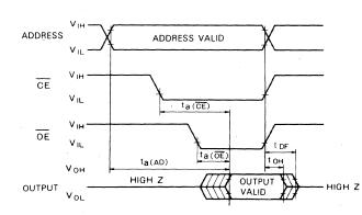
Test conditions for A.C. characteristics . Input voltage: VIL=0.45V, VIH=2.4V Input rise and fall times:  $\leq 20$ ns Reference voltage at timing measurement: Inputs 1V and 2V Output 0.8V, and 2V
