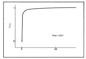
Fig. 3.3 Dependency of V<sub>TH</sub> on write pulse width (16K-bit and 32K-bit)
