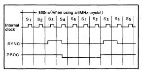
Fig.11 Clock and generated cycle signals
