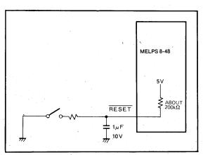
Fig. 13 Example of a reset circuit
