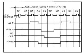
Fig.11 Clock and generated cycle signals
