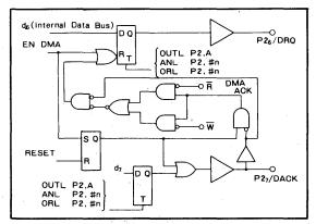
Fig.17 Internal configuration of DMA control
