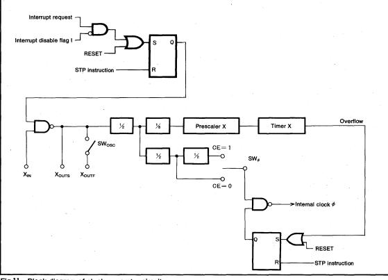
Fig.11 Block diagram of clock generator circuit
