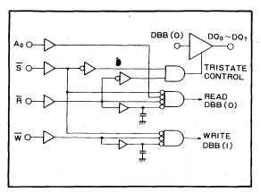
Fig.6 Internal configuration of data bus control
