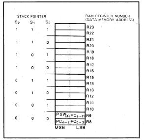
Fig. 6 Relation between the program counter stack and the stack pointer
