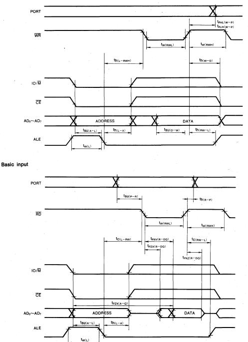
TIMING DIAGRAM (reference level, high-level=2V, low-level=0.8V) Basic output
