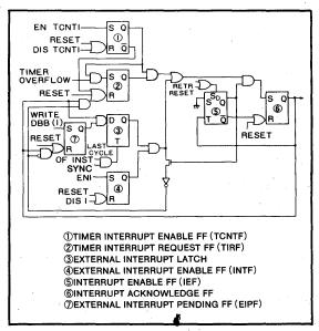
Fig.8 Interrupt control section configuration
