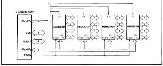
Fig.2 Expansion interface example
