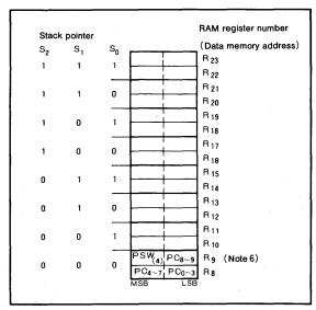
Fig.3 Relationship between program counter stack and stack pointer
