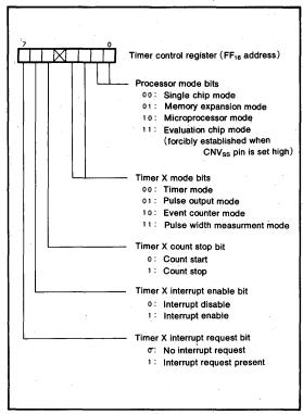
Fig.5 Configuration of timer control register
