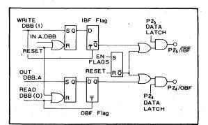
Fig.19 Internal configuration of IBF/OBF
