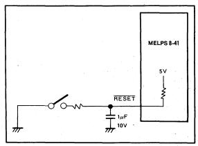
Fig.13 Example of reset circuit
