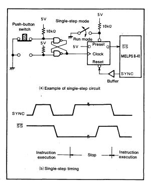
Fig.14 Single-step operation circuit and timing
