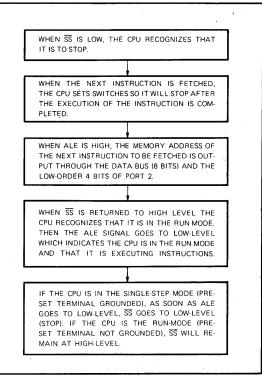
Fig. 15 CPU operation in single-step mode
