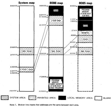
Solid line means that addresses are the same between each area. Solid line means that each area has the different address from others.
