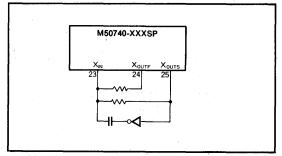
Fig.14 External RC circuit
