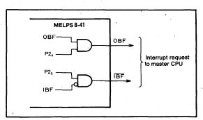
Fig.18 Interrupt request to master CPU
