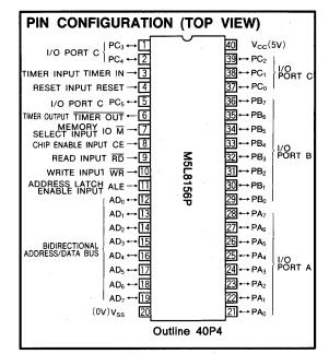
bits that can be used to count down (events or time) and it can generate square wave pulses that can be used for counting and timing.
