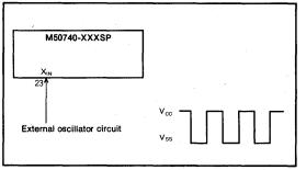
Fig.13 External clock input circuit
