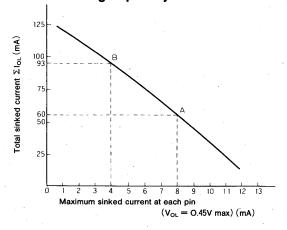
Each of the 16 I/O lines of the M5L8243P is capable of sinking 5mA simultaneously ( $V_{OL} = 0.45V$  max). However, the drive capacity of each line depends upon whether all lines are sinking current simultaneously and on the degree of loading. This is illustrated in the curve shown. Example
