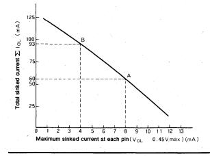
Each of the 16 I/O lines of the M5M82C43P is capable of sinking 5mA simultaneously ( $V_{OL} = 0.45V$  max). However, the drive capacity of each line depends upon whether all lines are sinking current simultaneously and on the degree of loading. This is illustrated in the curve shown. Example:
