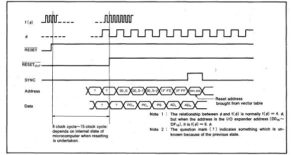
Fig.6 Timing diagram during resetting
