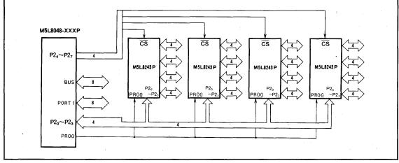
Fig.2 Expansion interface example
