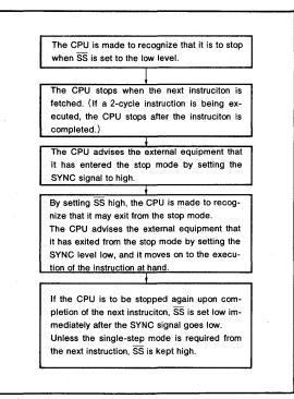
Fig.15 CPU operation in single-step mode
