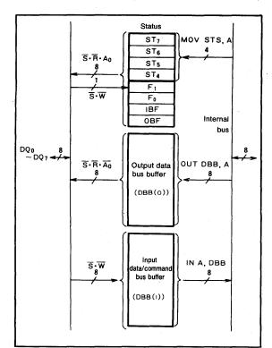
Fig.7 Internal configuration of data bus
