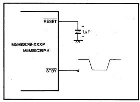
Fig. 2 Control circuit example for standby mode
