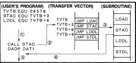
Note : The processing order is ①, ②, ③, ④, ⑤, A transfer vector is used to set the entry address of each subroutine.
