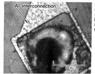
Fig. 8 Corrosion of vapordeposited aluminum interconnection, analyzed by metallurgical microscope interconnection, at a high current density region, caused by the operating life test. This test is performed as a step stress test to investigate IC degradation and failure by temperature and voltage. This phenomenon is due to aluminum electromigration, which is observed when high-current loads are applied to a vapor-deposited aluminum interconnection.
