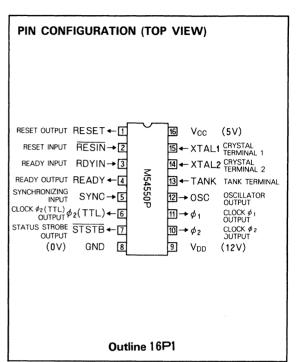
system power-up time, a reset signal is generated; and the system is reset automatically. When a signal from a CPU is applied to the SYNC, STSTB is generated. The RDYIN input sends a synchronous "wait request" signal to the internal D-type flip-flop, and a synchronized READY signal is generated.
