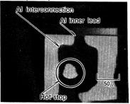
Fig. 10 Surge destruction, analyzed by metallurgical microscope
