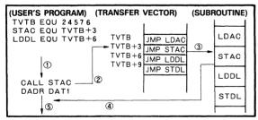
Note 1 : The processing order is ①, ②, ③, ④ and ⑤. A transfer vector is used to set the entry address of each subroutine.
