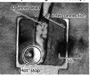
Fig.11 Enlargement of aluminum bridge in Fig. 10, analyzed by XMA-Al kα
