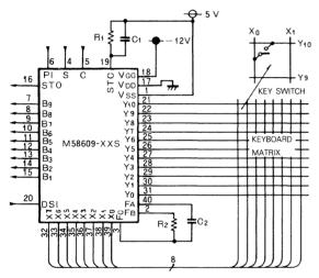
Note 4 :  $R_1 = 1.5M \Omega$ ,  $C_1 = 0.001 \mu$ F provides approximately 1.5ms delay time. 5 :  $R_2 = 75k \Omega$ ,  $C_2 = 50$ pF provides approximately 50kHz clock frequency.
