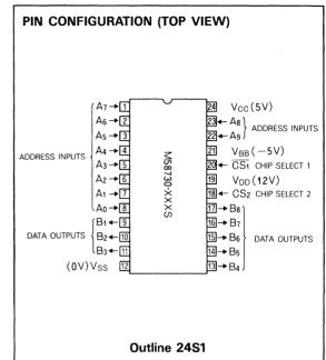
to data outputs  $B_1 \sim B_8$ . Chip select 1 ( $\overline{CS_1}$ ) and chip select 2 ( $CS_2$ ) are used to connect two or more M58730-XXXS ROMs. When  $\overline{CS_1}$  is high or  $CS_2$  is low, all outputs are disabled and will assume a floating (high-impedance) states.
