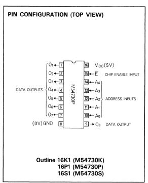
read out in parallel on data outputs  $0_1 \sim 0_8$ . All inputs are TTL-compatible. An external decoder is not necessary. All outputs are open-collector outputs, so it is possible to AND-tie them to other ROMs and TTL devices. The AND-tie fanout of each output can accommodate up to 10 standard TTL loads. The chip enable  $\overline{E}$  is used to inhibit data ouputs  $0_1 \sim 0_8$ .
