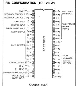
comparator generates a coincidence signal for clock control and delay circuit. This clock control stops the clock signals to the ring counter and data outputs  $(B_1 \sim B_9)$  stabilizing the selected 9-bit code. The stabilization is indicated by a valid signal on the strobe output. A strobe output signal is generated at the time set by the externally controlled delay circuit which receives the coincidence signal. Data outputs and strobe output remain stable until the key is released.
