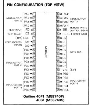
bit data port, which may be programmed to be an input or an output, and one 4-bit control-data port used for handshaking and interrupt control signals. Mode 2 is used with group A only, as one 8-bit bidirectional bus port and one 5-bit control port.
