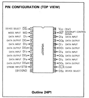
request flip-flop SR is set. Also, the strobed input STB is active, the data inputs  $DI_1 \sim DI_8$  are latched in the data latches, and the service request flip-flop SR is reset.
