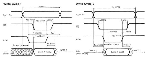
Note 2 : The input signals from the external circuits should not be applied to the I/O terminals (keeping them three-state) for during this period the I/O terminals are in the output mode.
