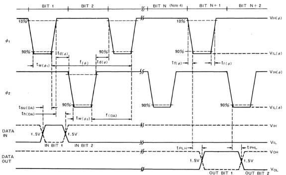
Note 2 :  $t_{su(DA)}$  and  $t_{h(DA)}$  have the same value concerning  $t_{w(\phi 2)}$ .
