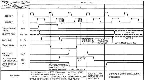
Besides the states shown in Fig.3, there is a state T<sub>H</sub>, in which the CPU stays in the hold state after the machine cvcle.
