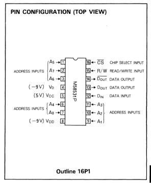
The M58531P has two power supply terminals,  $V_{DD}$  for the memory cell part in which the data is stored, and  $V_D$  for the read/write control circuit. Power dissipation is low since, during standby, current is supplied only to the memory cell part for data storage, and read/write operation is not performed.
