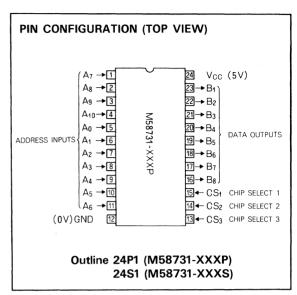
of the address. The three chip select inputs are programmable during the masking process, and any combination of active high-level and active low-level may be used for chip selection. When a chip is selected, the contents of the ROM are read out; and under other conditions, the data outputs  $(B_1 \sim B_8)$  are in the floating (high-impedance) state.
