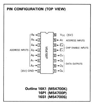
read out in parallel on data outputs  $0_1 \sim 0_4$ . All inputs are TTL-compatible. An external decoder is not necessary. All outputs are open-collector outputs, so it is possible to AND-tie them to other ROMs and TTL devices. The AND-tie fanout of each output can accommodate up to 10 standard TTL loads. The chip enables  $\overline{E_1}$  and  $\overline{E_2}$  are used to inhibit data outputs  $O_1 \sim O_4$ .
