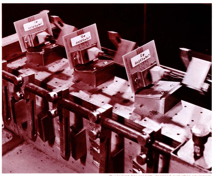
Our test lab has specially designed evaluation equipment that operates the key modules around the clock, hammering out millions of operations to simulate years of normal keyboard use.
