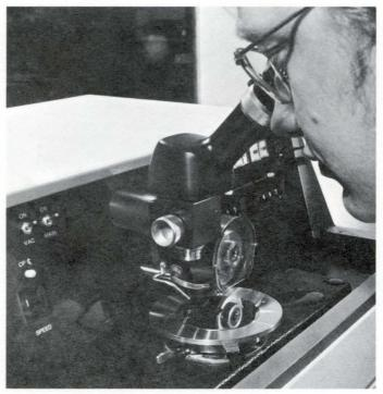
Silicon wafer separation by ultrahigh-speed saw insures the straight sides needed for the continued automated handling of the microscopic chips.
