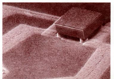
Perhaps the most significant advancement in reducing the price and increasing the reliability of the SD line is the development of an advanced mounting technique that places the chip face down on the ceramic and gives the new technology its name—"flip chip." With this process, the proven reflow solder method replaces the laborious hand operation of ultrasonically bonding the microscopic wires from the chip to the lead frame.
