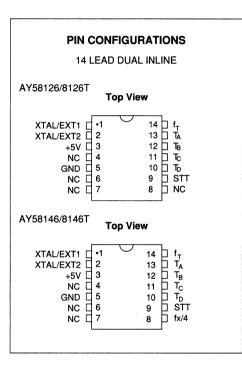
low by one clock period  $(1/f_x)$ . The clock frequency  $(f_x)$  is used by the 8146/8146T to provide a high frequency output  $(f_x/4)$ .
