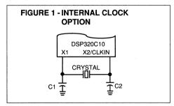
The crystal should be fundamental mode, and parallel resonant, with an effective series resistance of 30 ohms, a power dissipation of 1mW, and be specified at a load capacitance of 20pF.
