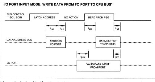
\* Assume the direction of the I/O port has already been determined via a write to the Enable register (R7A).
