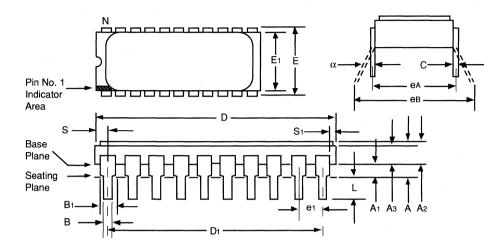
Package Type: 20-Lead Ceramic Side Brazed Dual In-line (.300 mil)
