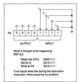
that file to be read into the CPU (MOVF, BIT SET, BIT CLEAR, and BIT TEST) is executed. Otherwise, the previous state of that pin may be read into the CPU rather than the new state. This will happen if tpd (See I/ O Timing Diagram) is greater than 1/4tcy (min). When in doubt, it's better to separate these instructions with a NOP or other instruction.
