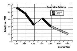
as speed, power and device leakage. Its present level has reached 200 ppm  $\underline{atter\ programming},$  with a goal of 100 ppm.
