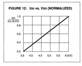
NOTE: The following graphs are based on characterization data and are for design guidance only. Most graphs are normalized to the worst case conditions to allow easy extrapolation for different operating conditions. For example, IDD max at 2.0 MHz, 5.0V can be derived from 3.3 mA  $\cdot$  0.7  $\cdot$  0.65  $\approx$  1.5 mA.
