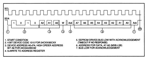
Figure 3 as shown below describes how the bit stream is set up for READ and WRITE mode in the microcomputer programming software prior to sending it on the two wire serial bus.
