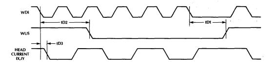
Write Mode Timing Diagram
