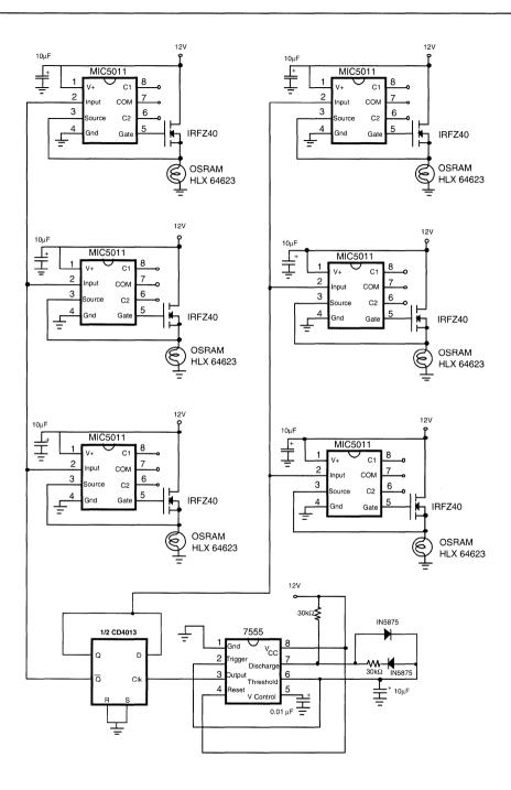
Figure 2: A 75X/Minute, 50% Duty Cycle Halogen Flasher
