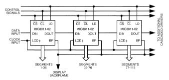
Figure 2. Cascading with External Clocking Source - Option -02
