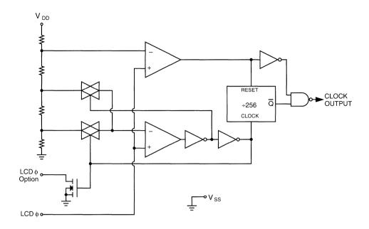
Figure 1. Internal Oscillator Circuit
