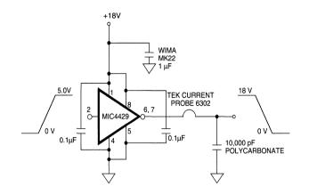
Figure 6. Peak Output Current Test Circuit
