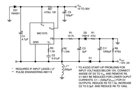
Figure 7. Positive to Negative Buck-Boost Converter
