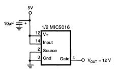
Figure 11. DC - DC Converter
