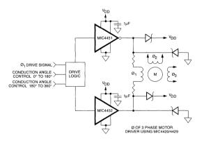
Figure 3. Direct Motor Drive
