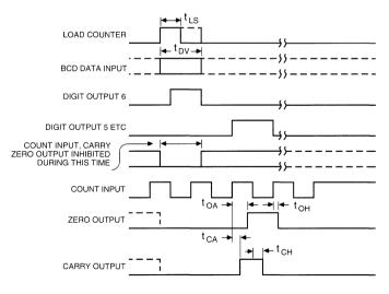
t<sub>LS</sub> 2.0 μS min NOTE: REF. TO POSITIVE TRANSITION OF DIGIT OUTPUT
