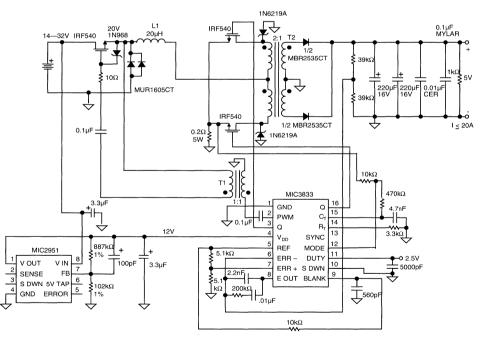
Figure 5: 100 W Current Fed Push – Pull DC to DC Converter
