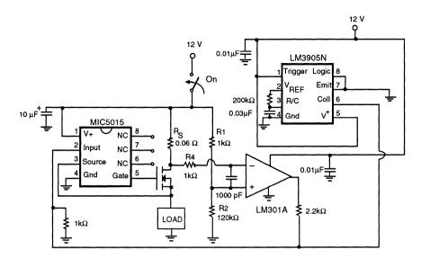
Figure 5: High Side Driver With Delayed Overcurrent Shutdown
