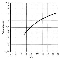
NOTE: THE VALUES ON THIS GRAPH REPRESENT THE LOSS SEEN BY BOTH DRIVERS IN A PACKAGE DURING ONE COMPLETE CYCLE. FOR A SINGLE DRIVER DIVIDE THE STATED VALUES BY 2. FOR A SINGLE TRANSITION OF A SINGLE DRIVER, DIVIDE THE STATED VALUE BY 4.
