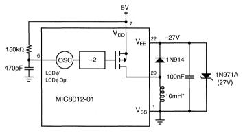
\* 129T, 30 gauge Cu, wound on Philips (Ferroxcube) core #2213P-A600-3B7
