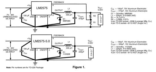
As in any switching regulator, layout is very important. Rapidly switching currents associated with wiring inductance generate voltage transients which can cause problems. For minimal stray inductance and ground loops, the length of the leads indicated by heavy lines should be kept as short as possible. Single-point grounding (as indicated) or ground plane construction should be used for best results.
