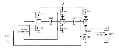
Figure 14. Gate Control Circuit Detail
