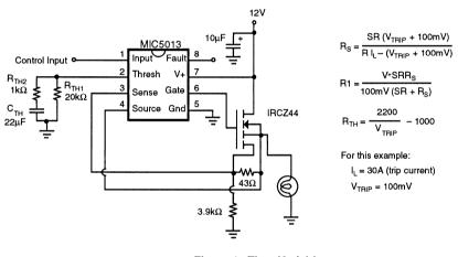
Figure 1. Time-Variable Trip Threshold
