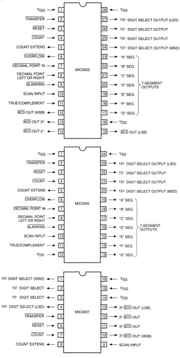
are different versions of this same chip are the MIC5005 and MIC5007. The MIC5005 is supplied in a 24-pin package and does not include the BCD outputs. The MIC5007 is supplied in a 16-pin package. (See Figure 2 for these members of the display counter/decoder family.)
