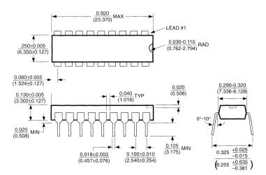
Note: Pin 1 will be denoted by one or more of the following: a notch, a printed triangle, or a mold mark.
