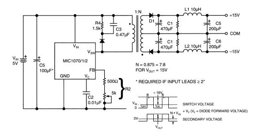
Figure 6. Totally Isolated Converter
