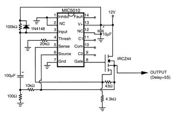
Figure 12. Time-Delay Relay with 30A Over-Current Protection
