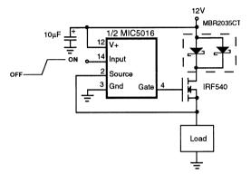
Figure 12: High Side Driver WIth Load Protection
