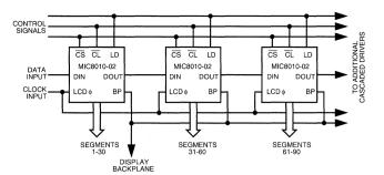
Figure 3. Cascading with External Clocking Source - 02 Configuration
