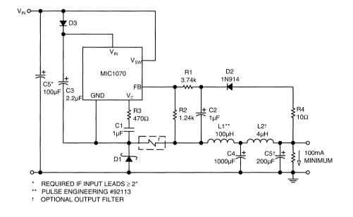
Figure 13. Positive Buck Converter
