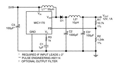
Figure 1 Boost Converter (5V to 12V)
