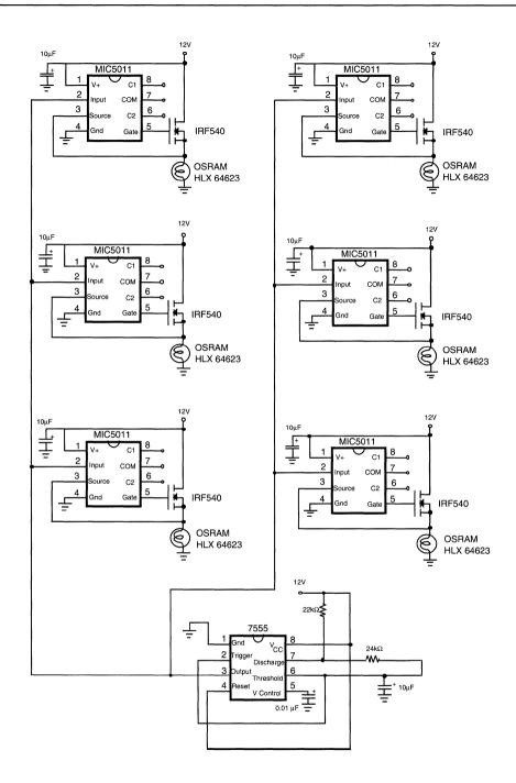
Figure 3: A 120X/Minute Halogen Flasher
