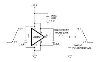
Figure 6. Peak Output Current Test Circuit
