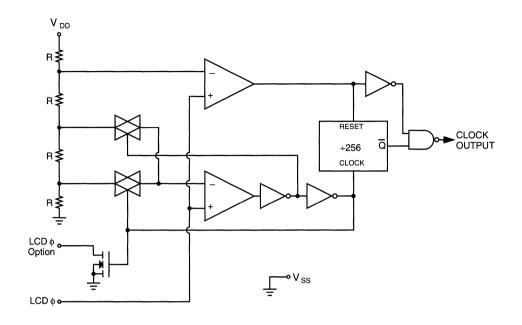
Figure 1. Internal Oscillator Circuit
