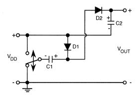
Figure 1. Charge Pump Voltage Doubler
