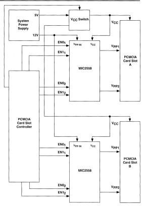
Figure 3. MIC2558 Typical two slot PCMCIA application with single 5.0V  $\rm V_{cc}.$
