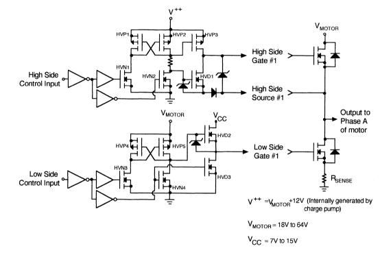
Figure 1. MPD8020-0011 Output Stage (one of three)
