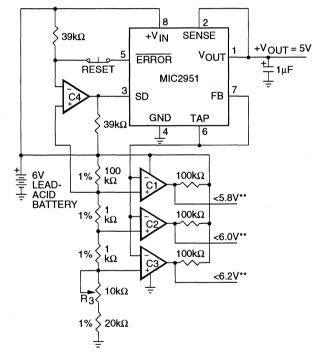
C1 TO C4 ARE COMPARATORS (LP339 OR EQUIVALENT) \*OPTIONAL LATCH OFF WHEN DROP OUT OCCURS. ADJUST R3 FOR C2 SWITCHING WHEN V<sub>IN</sub> IS 6.0V
