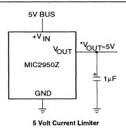
\* MINIMUM INPUT-OUTPUT VOLTAGE RANGES FROM 40mV TO 400mV, DEPENDING ON LOAD CURRENT.
