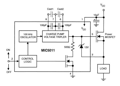
Figure 2. MIC5011 Block Diagram
