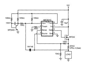
Figure 4: Automatically Resettable 10 A Circuit Breaker
