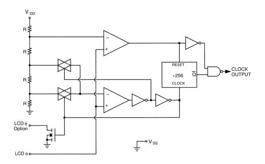
Figure 3. Internal Oscillator Circuit
