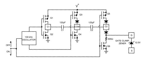
Figure 12. Gate Control Circuit Detail
