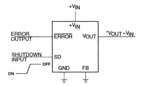
\*MINIMUM INPUT-OUTPUT VOLTAGE RANGES FROM 40mV TO 400mV, DEPENDING ON LOAD CURRENT.
