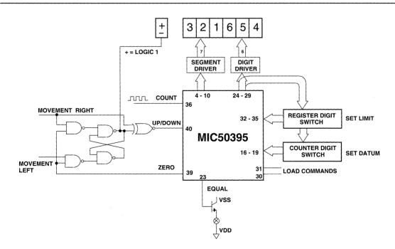
Figure 10: Positional Measurement
