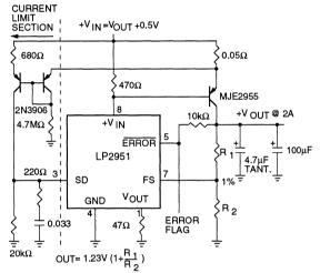
FOR 5  $V_{cutt}$  USE INTERNAL RESISTORS. WIRE PIN 6 TO 7, AND WIRE PIN 2 TO +V\_{cutt} BUS.
