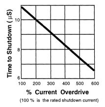
Figure 2: Shutdown Time vs. % Current Overdrive
