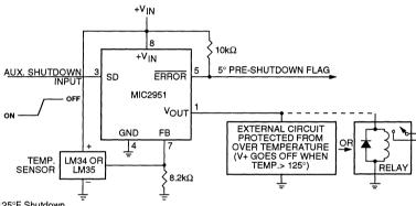
LM34 for 125°F Shutdown LM35 for 125°C Shutdown
