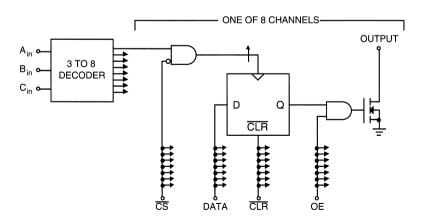
Figure 5. Block Diagram of Logic Circuitry
