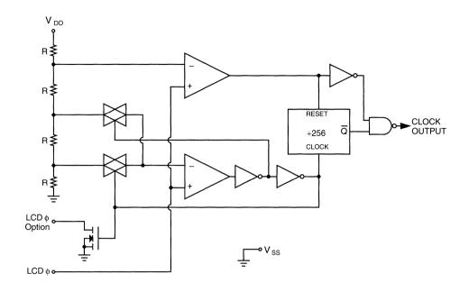
Figure 1. Internal Oscillator Circuit
