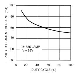
Figure 3. Pulsed Filament Current vs. Duty Cycle
