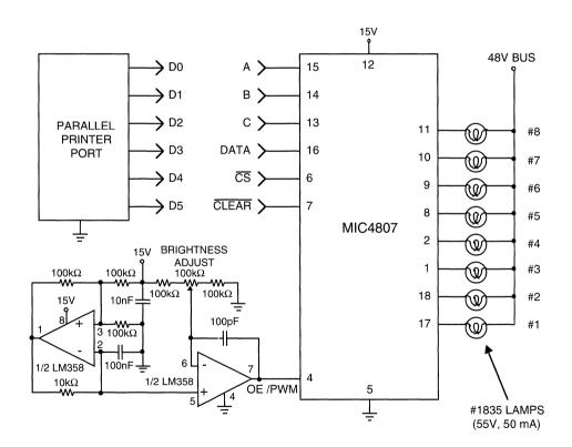
Figure 2. MIC4807 Display Controller with PWM Dimming
