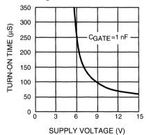
Low-side Turn-on Time for Gate = 5V 1000 300 **ΓURN-ON TIME (μS)** CGATE=10 nF 100 30 10 CGATE=1 nF 3 1 3 6 9 0 12 15 SUPPLY VOLTAGE (V) \* Time for gate to reach V<sup>+</sup> + 5V in test circuit with VS = V<sup>+</sup> - 5V.
