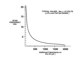
Figure 7: Scan Frequency vs. External
