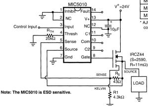
Figure 1. High-Side Driver with Current-Sensing MOSFET
