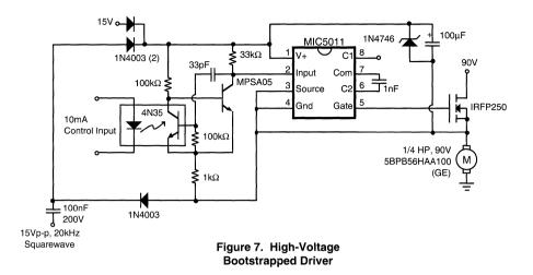
diode limits the supply to 18V. When the MIC5011 is off, power is supplied by a diode connected to a 15V supply. The circuit of Figure 5 is put to good use as a barrier between low voltage control circuitry and the 90V motor supply.
