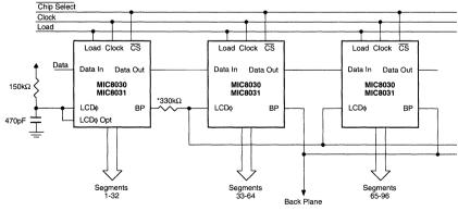
\*Required if using MIC8031 with V BB>50V.
