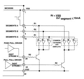
Figure 5: Driving LED Displays Directly
