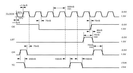
NOTE 1: To store counter information the latch strobe may go as low at any time up to 50nS before the positive going transition of counter resets.
