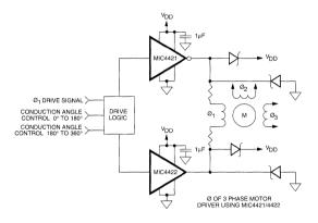
Figure 3. Direct Motor Drive
