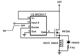
Figure 6: DC Motor Speed Control/Driver
