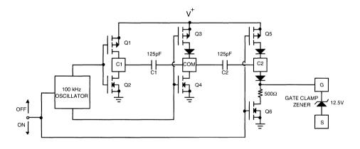
Figure 14. Gate Control Circuit Detail
