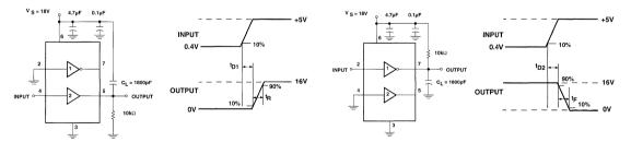
Figure 1. MIC4403 Switching time test circuit.
