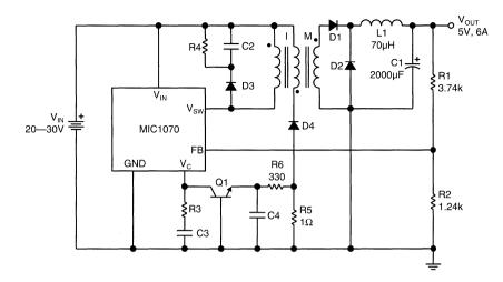
Figure 17. Forward Converter
