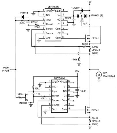
Figure 11. Half-Bridge Motor Driver
