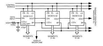
Figure 2. Cascading with Internal Clock Oscillator - 01 Configuration
