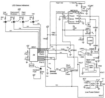
Figure 5: Z8 Based Power Controller
