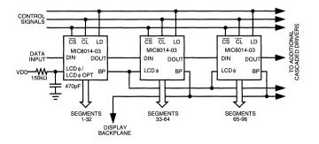
Figure 2. Cascading with Internal Clock Oscillator
