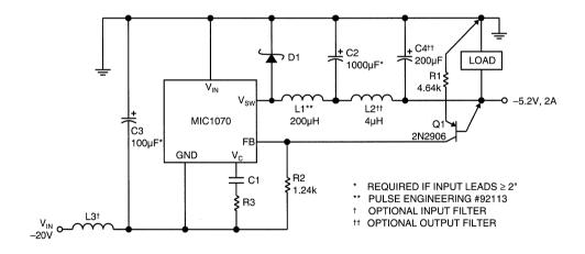
Figure 11. Negative Buck Converter
