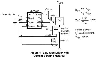
terminal from inductive switching transients. The MIC5013 supply should be limited to 15V in low-side topologies; otherwise, a large current will be forced through the gate clamp zener.
