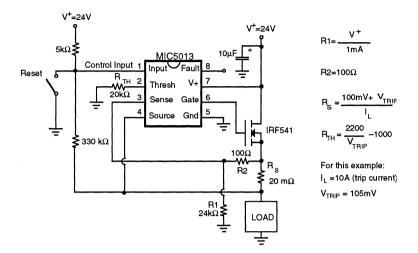
Figure 1: Basic Circuit Breaker/Switch Configuration
