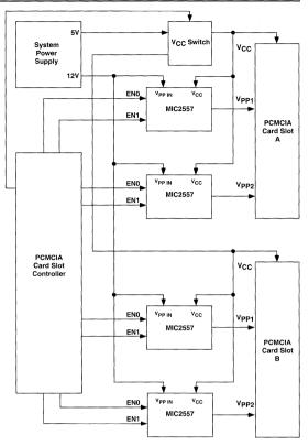
Figure 3. MIC2557 Typical two slot PCMCIA application with single 5.0V  $\rm V_{cc}.$
