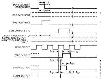
t<sub>LS</sub> 2.0 μS min NOTE: REF. TO POSITIVE TRANSITION OF DIGIT OUTPUT
