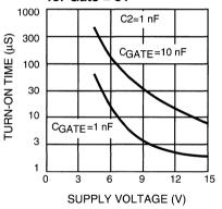
Low-side Turn-on Time for Gate = 10V3000 1000 300  $C_{GATE}=10 \text{ nF}$
