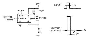
Figure 3. Inductive Spike Clamping
