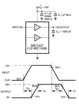
Figure 2. Non-Inverting Driver Switching Time
