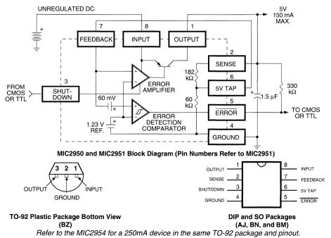
These system functions also include an error flag output that warns of a low output voltage, which is often due to failing batteries on the input. This may also be used as a power-on reset. A logic-compatible shutdown input is also available which enables the regulator to be switched on and off. This part may also be pin-strapped for a 5 V output, or programmed from 1.24 V to 29 V with the use of two external resistors.
