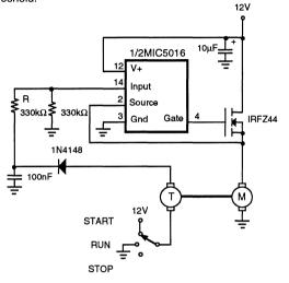
Figure 10. Motor Stall Shutdown
