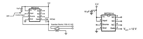
Figure 11. DC - DC Converter
