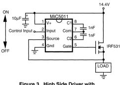
Figure 3. High Side Driver with External Charge Pump Capacitors
