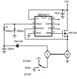
Figure 10. Motor Stall Shutdown
