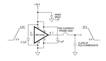
Figure 6. Peak Output Current Test Circuit
