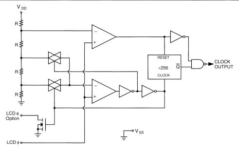
Figure 1. Internal Oscillator Circuit
