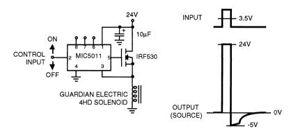
Figure 4. Clamping Inductive Transients
