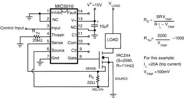
Figure 4. Low-Side Driver with Current-Sensing MOSFET
