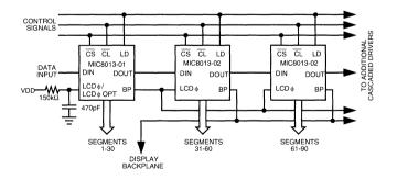
Figure 2. Cascading with Internal Clock Oscillator - 01 Option
