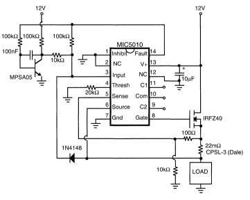
Figure 7. 10-Ampere Electronic Circuit Breaker
