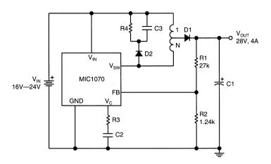
Figure 10. Current Boosted Boost Converter
