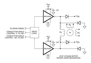
Figure 3. Direct Motor Drive
