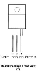
The LP2954 has a tight initial tolerance (0.5% typical), a very low output voltage temperature coefficient which allows use as a low-power voltage reference, and extremely good load and line regulation (0.05% typical). This greatly reduces the error in the overall circuit, and is the result of careful design techniques and process control.
