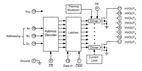
Figure 1. MIC4807 Block Diagram
