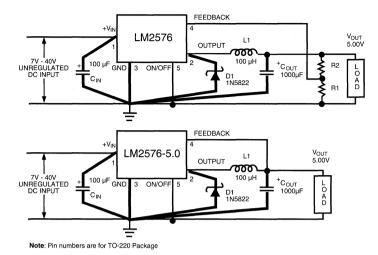
C<sub>IN</sub> --- 100µF, 75V Aluminum Electrolytic COUT - 1000µF, 15V Aluminum Electrolytic C<sub>OUT</sub> — 1000/F, 159 AduInitum Electroytec D1 — Schotky, 115822 L1 — 100µH, PE-92108 (Pulse Engineering) R1 — 1k, 0.01% R2 — 3.065k, 0.01% 5-pin TO-220 socket—2936 (Loranger Mfg. Co.) 4-pin TO-3 socket—8112-AG7 (Augat Inc.)
