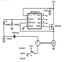
Figure 10. Motor Stall Shutdown
