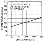
MIC1070/1/2 Feedback Pin Clamp Voltage
