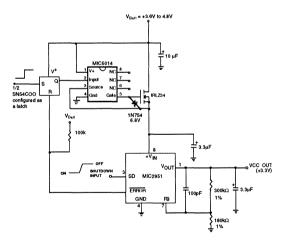
Figure 3: Low Battery Shutdown Switch
