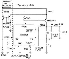
FOR 5  $V_{\text{out}}$  . USE INTERNAL RESISTORS. WIRE PIN 6 TO 7, AND WIRE PIN 2 TO +V\_{\text{out}} BUS.
