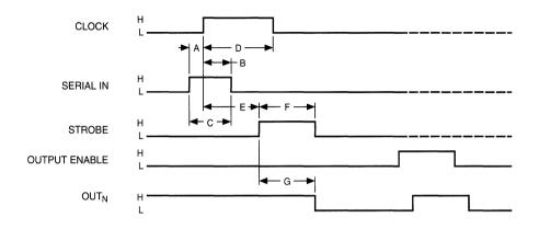
Timing Diagram—Serial Mode
