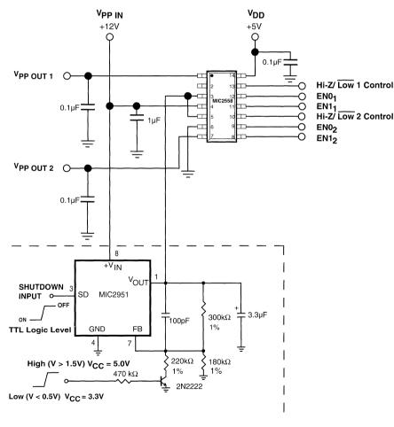
Figure 3. Full PCMCIA Implementation of V<sub>PP</sub> and V<sub>cc</sub> switching using MIC2558 and MIC2951 voltage regulator. 8-13
