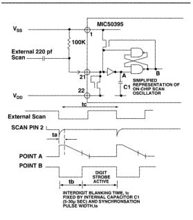
Figure 8: External Drive To Scan Input
