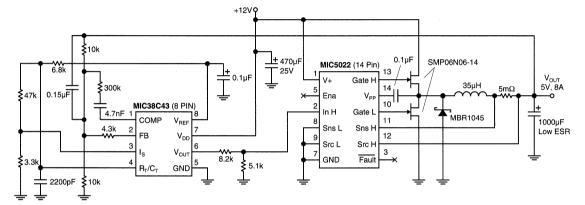
100kHz High Efficiency Synchronous Buck Rectifier
