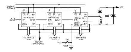
Figure 2. Cascading with MIC8010/12
