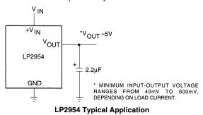
At lower values of output current, less output capacitance is required for output stability. The capacitor can be reduced to  $0.5\mu$ F for current below 10mA or  $0.15\mu$ F for currents below 1mA.
