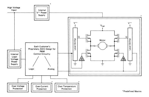
The above motor control application shows how a mixture of predefined macros and customer proprietary ASIC control circuits are used to make a circuit optimally fit an application. Each transistor in the bridge can be a single DMOS FET, or 2 to 4
