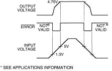
Figure 1. ERROR Output Timing
