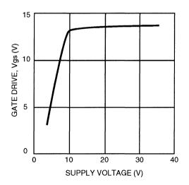
Figure 3. Gate Drive vs. Supply Voltage
