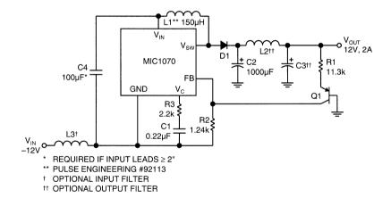
Figure 4. Negative to Positive Buck-Boost Converter
