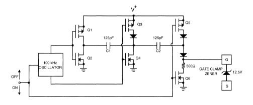
Figure 10. Gate Control Circuit Detail
