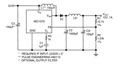
Figure 1. Boost Converter (5V to 12V)
