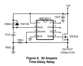
**Time-Delay Relay** (Figure 9). The MIC5011 forms the basis of a simple time-delay relay. As shown, the delay commences when power is applied, but the  $100k\Omega/1N4148$  could be independently driven from an external source such as a switch or another high-side driver to give a delay relative to some other event in the system. Hysteresis has been added to guarantee clean switching at turn-on.
