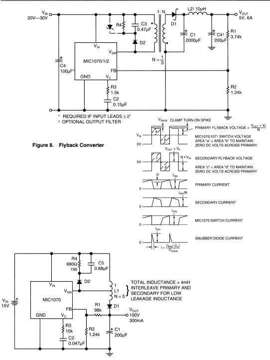
Figure 9. Voltage Boosted Boost Converter
