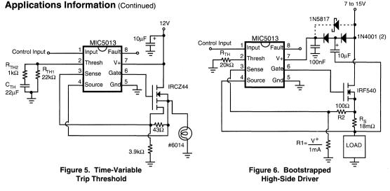
resistances.  $R_{DS(ON)}$  as specified on MOSFET data sheets includes bond resistances. A Kelvin-connected ohmmeter (using TAB and SOURCE for forcing, and SENSE and KELVIN for sensing) is the best method of evaluating "R." Alternatively, "R" can be estimated for large MOSFETs  $(R_{DS(ON)} {\leq} 100 \mathrm{m}\Omega)$  by simply halving the stated  $R_{DS(ON)}$ , or by subtracting 20 to 50m $\Omega$  from the stated  $R_{DS(ON)}$  for smaller MOSFETs.
