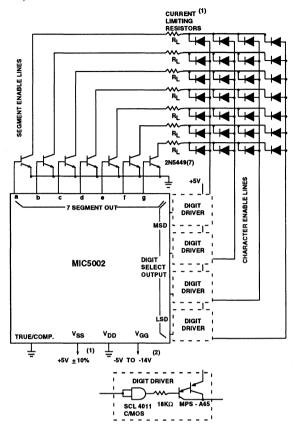
FIG. 7: INTERFACING WITH COMMON CATHODE LED'S (SUCH AS HEWLETT-PACKARD 5082-7200 SERIES, MONSANTO MAN-3)
