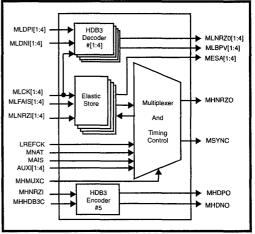
Figure 2: Multiplexer Side Block Diagram
