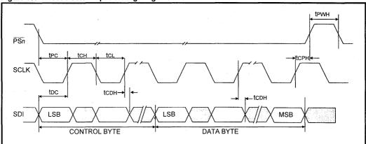
Figure 15: LXT331 Serial Input Timing Diagram
