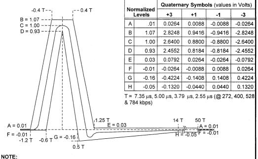
1. Pulse amplitude measured across a 135 W resistor on the line side of the transformer using the application circuit shown in Figure 13 and Table 21.
