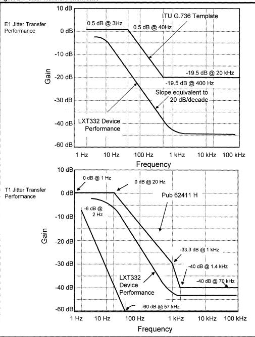
Figure 21: Jitter Transfer Performance
