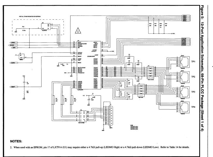
LXT914 Flexible Quad Ethernet Repeater
