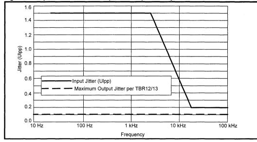
Figure 20: Input and Maximum Output Jitter Specified by TBR12/13
