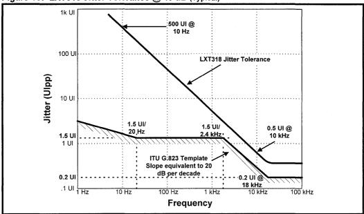
Figure 18: LXT318 Jitter Tolerance @ 43 dB (Typical)
