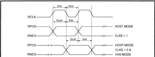
Figure 13: LXT307 Receive Clock Timing
