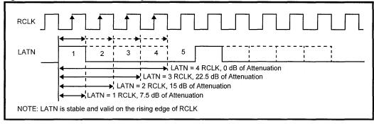
Figure 2: LATN Pulse Width Encoding
