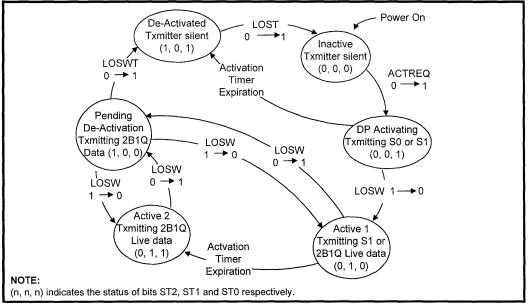
Figure 6: HTU-C Data Pump Activation State Machine
