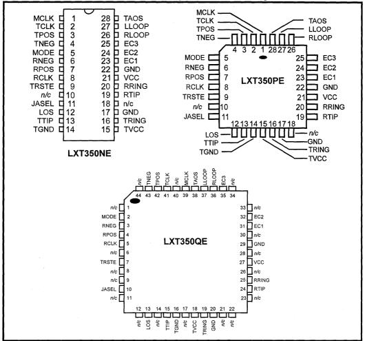
Figure 1: LXT350 Hardware Controlled Bipolar Mode Pin Assignments
