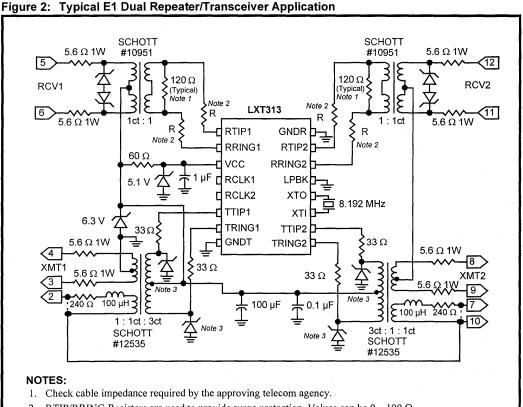
RTIP/RRING Resistors are used to provide surge protection. Values can be 0 - 100 Ω.
