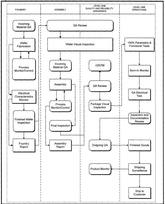
Figure 1: Level One Production Flow
