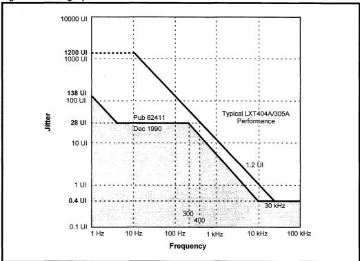
Figure 3: Charting Input Jitter Tolerance Test Results
