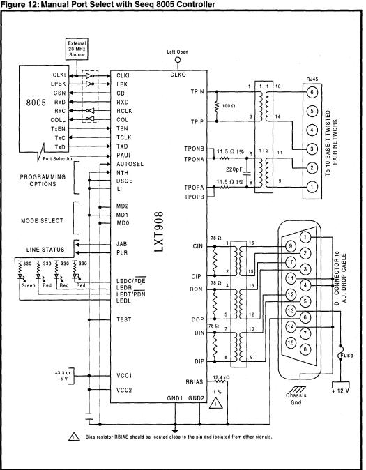
Figure 12: Manual Port Select with Seeq 8005 Controller
