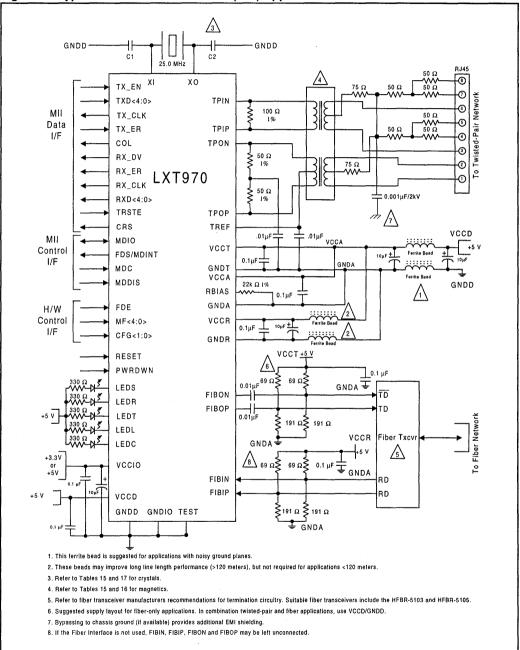
Figure 15: Typical Network Interface Card (NIC) Application
