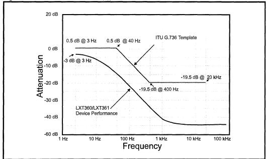
Figure 26: T1 Jitter Attenuation (Typical)
