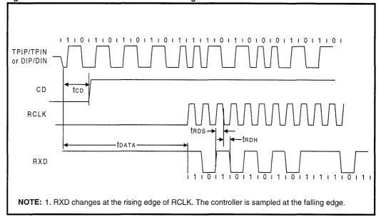
Figure 22: Mode 2 RCLK/End-of-Frame Timing
