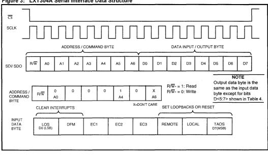
Figure 3: LXT304A Serial Interface Data Structure
