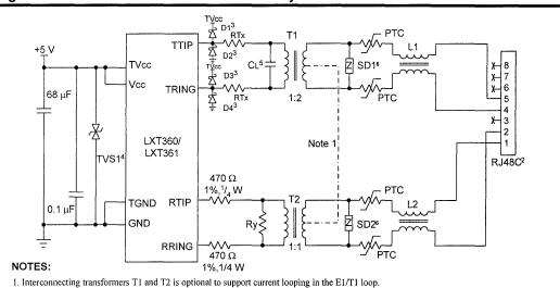
Figure 1: Enhanced Line Protection Circuitry
