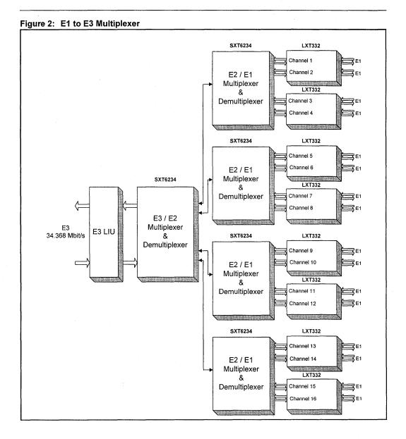
Designing an ITU G.742 Compliant PDH Multiplexer with the LXT332 Dual Transceiver
