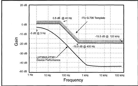
Figure 25: E1 Jitter Transfer Performance (Typical)
