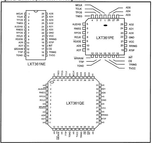
Figure 2: LXT361 Bipolar Mode Pin Assignments
