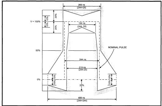
Figure 12: 2.048 Mbps Pulse Mask Template
