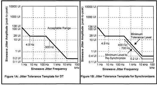
Figure 1: Input Jitter Tolerance Specified by AT&T Publication 62411
