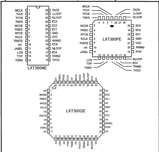
Figure 1: LXT360 Hardware Controlled Bipolar Mode Pin Assignments
