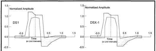
Figure 17: 1.544 MHz T1 Pulse (DS1 and DSX-1) (See Table 39)
