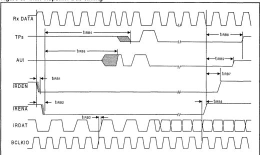
Figure 6: Inter-Repeater Bus Timing
