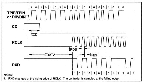
Figure 9: Mode 2 RCLK/End-of-Frame Timing
