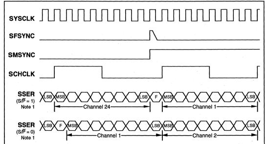
Figure 4: System Multiframe Boundary Timing (SYSCLK = 1.544 MHz)
