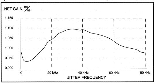
Figure 8: Nominal Jitter Transfer - 2.048 MHz CLKI to 1.544 MHz CLKO (Input Jitter = 0.25 UI)
