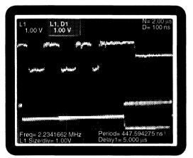
Figure 7B: DI (AUI) End of Frame with Test Load (Capacitor Coupling)
