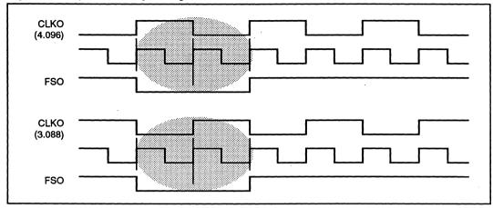
Figure 4: Output Frame Sync Alignment when HFO = 2 x CLKO
