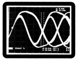
Figure 19: LXT902 Random Data Output Jitter (After Line Model - Rising Edge Trigger)
