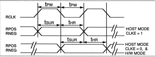
Figure 5: LXT300 Receive Clock Timing Diagram
