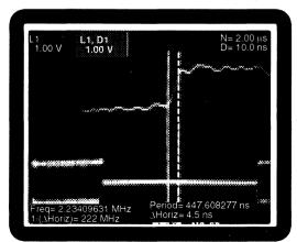
Figure 6B: DI (AUI) Rise time < 5 ns with Test Load (Capacitor Coupling)
