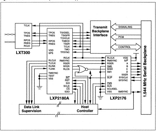
Figure 8: Serial 1.544 MHz Backplane Interface Application
