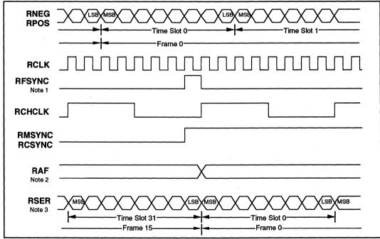
Figure 18: Receive Multiframe Boundary Timing
