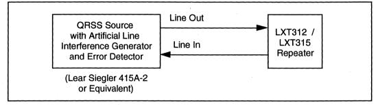
Figure 8: Receiver Gaussian Noise Immunity Test Setup
