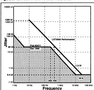
Figure 5: LXT305A Receive Jitter Tolerance
