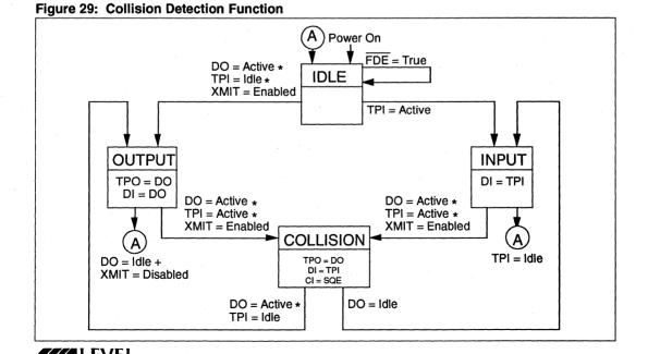
disabled when a data collision occurs, clearing the RXD circuit for the TPI data. Normal loopback is also disabled during link fail and jabber states.
