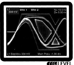
Figure 4B: Random Data after the 150  $\Omega$  Line Model (Waveform template and Jitter spec.)
