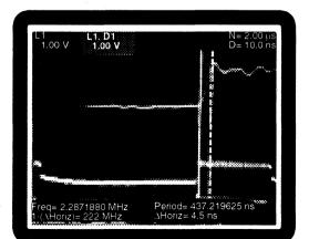
Figure 6A: DI (AUI) Rise time < 5 ns with Test Load (Transformer Coupling)
