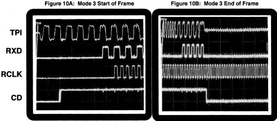
(Mode 3 : Compatible with Fujitsu MB86950 and 86960 controllers.)
