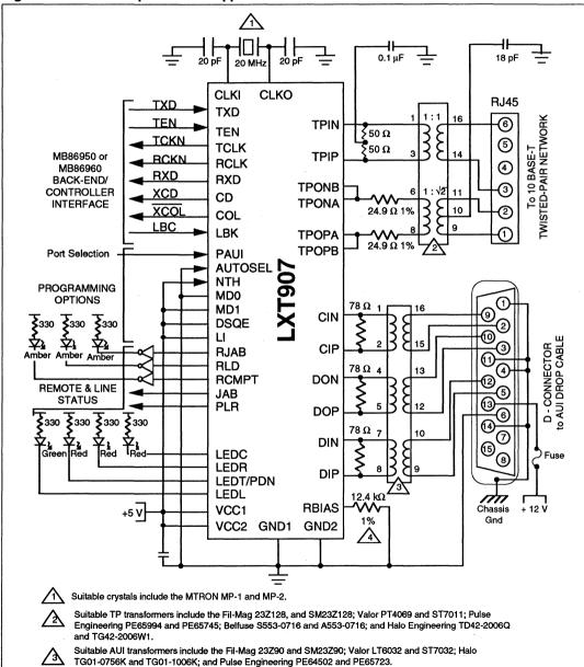
Figure 35: LAN Adapter Board Application - Manual Port Select with Link Test Function
