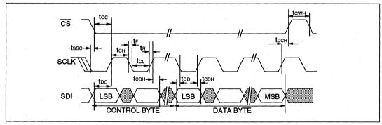
Figure 25: Serial Port Read A.C. Timing
