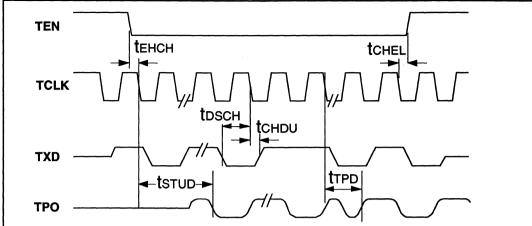
Figure 11: Mode 2 Collision Detect Timing
