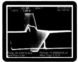
Figure 5B: Link Test Pulse after Line Model
