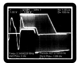
Figure 4A: TP Idle Pulse before Line Model with Test Load
