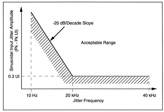
Figure 3: Receiver Jitter Tolerance Template
