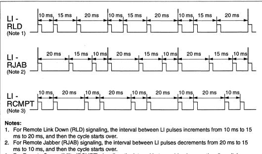
3. For Remote Compatibility (RCMPT) signaling, the interval between LI pulses continually switches between 10 ms and 20 ms.
