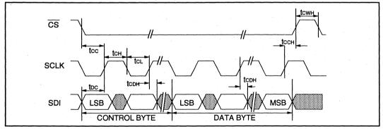
Figure 9: LXT310 Serial Data Output Timing Diagram
