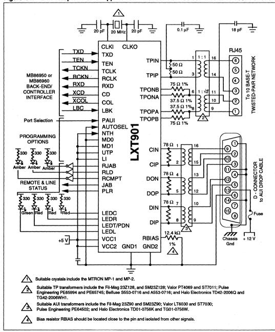
Figure 34: LAN Adapter Board Application - Manual Port Select with Link Test Function
