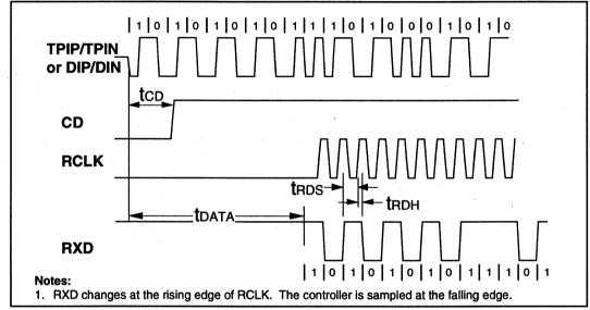
Figure 3: Mode 1 RCLK/EoF Timing
