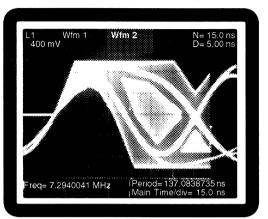
Figure 3B: Random Data after the Line Model (Waveform template and Jitter spec.)
