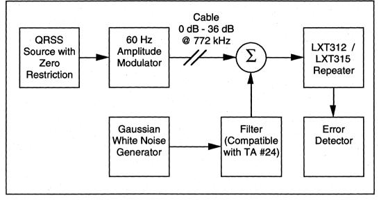
Figure 10: Receiver Timing Recovery Phase Shift Modulation Test Setup
