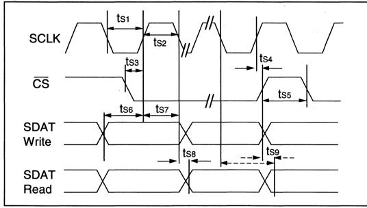
Figure 2: LXT903 Serial Interface Timing
