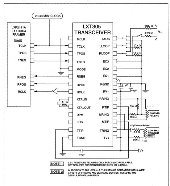
Figure 9: Typical LXT305 2.048 MHz E1 Application (Hardware Mode)
