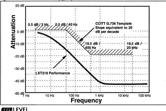
Figure 8: LXT318 Jitter Attenuation (Typical)
