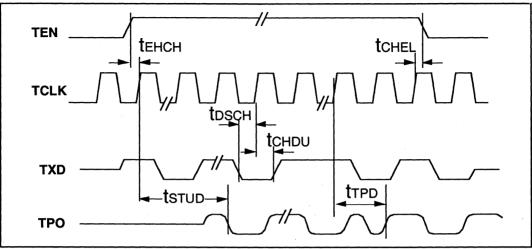
Figure 23: Mode 4 Collision Detect Timing
