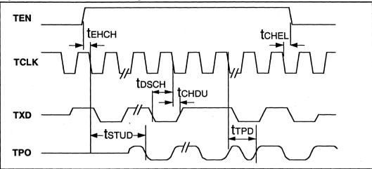
Figure 17: Mode 3 Collision Detect Timing
