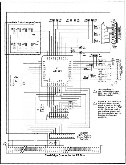
Figure 2: Schematic Diagram of the LDB901 Evaluation / Demonstration Board
