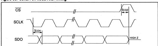
Figure 30: Serial Port Read A.C. Timing
