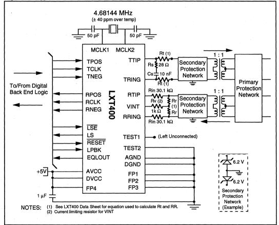
Figure 1: Typical LXT400 64 kbps Clear Channel Application
