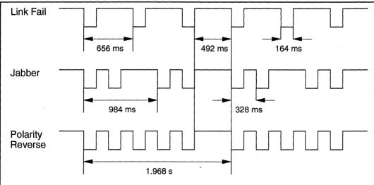
**NOTE:** LEDP/S status indications are shown in order of priority, i.e., Link Fail indication supersedes Jabber indication which supersedes Polarity Reverse (when PRC = 1). Reversed polarity conditions supersede Link Fail conditions when PRC = 0 (Polarity Correction Disabled). At the LEDL indicator, reversed polarity conditions are reported as Link Fail when PRC = 0. This allows the user to distinguish between actual link failure and apparent link failure due to polarity reversal.
