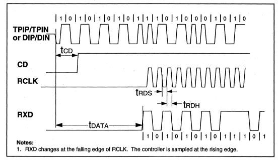
Figure 21: Mode 4 RCLK/End-of-Frame Timing
