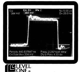
Figure 5B: TP Idle Pulse after Line Model with Test Load
