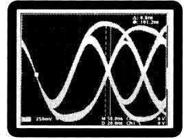
Figure 20: LXT901 Random Data Output Jitter (After Line Model - Falling Edge Trigger)
