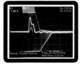
Figure 7: DI (AUI) Rise time < 5 ns with Test Load (Transformer Coupling)
