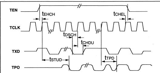
Figure 4: Mode 1 Transmit Timing
