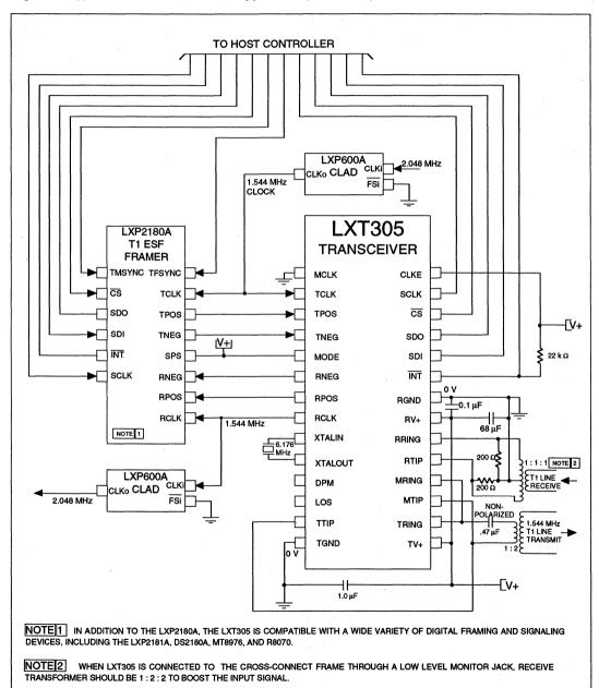
Figure 8: Typical LXT305 1.544 MHz T1 Application (Host Mode)
