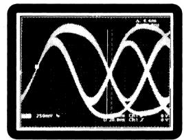
Figure 18: LXT901 Random Data Output Jitter (After Line Model - Rising Edge Trigger)
