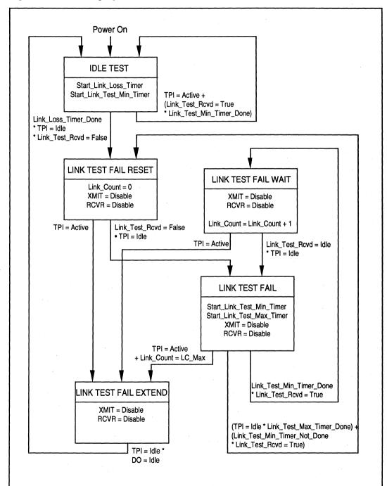
Figure 3: Link Integrity Test Function
