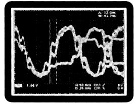
Figure 16: LXT901 Random Data Output Jitter (0 Line Length - Falling Edge Trigger)
