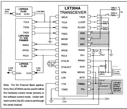
Figure 12: LXT304A 1.544 MHz D4 Channel Bank Applications (Hardware Mode)
