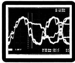
Figure 14: LXT901 Random Data Output Jitter (0 Line Length - Rising Edge Trigger)
