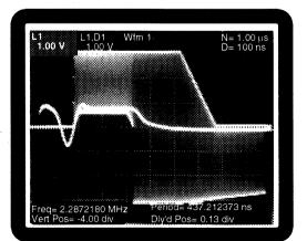
Figure 4B: TP Idle Pulse after Line Model with Test Load
