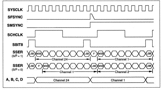
Figure 3: System Multiframe Boundary Timing (SYSCLK = 1.544 MHz)
