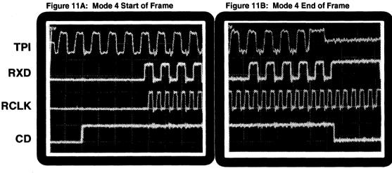
(Mode 4 : Compatible with National Semiconductor NS8390 controllers. Mode 1, compatible with Advanced Micro Devices AM7990 controllers, is similar.)
