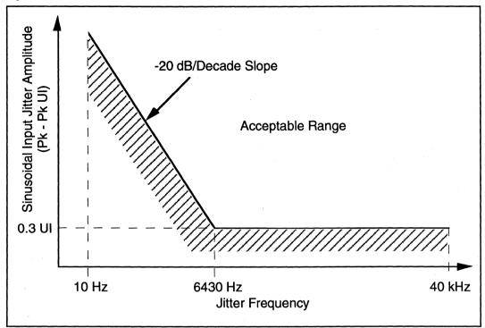
Figure 3: Receiver Jitter Tolerance Template
