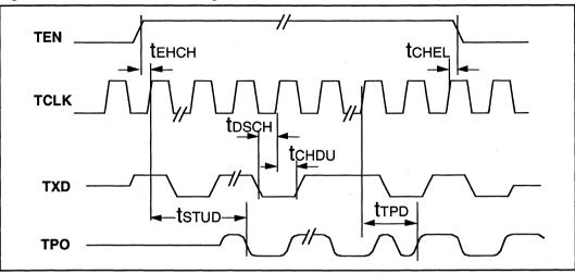
Figure 23: Mode 4 Collision Detect Timing
