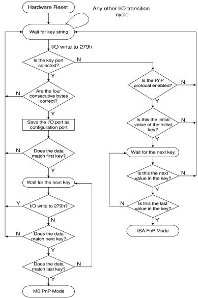
Figure 6-1. Configuration Sequence Flow Chart
