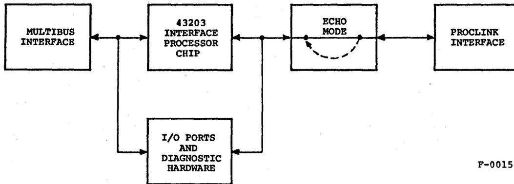
Figure 6-1. Interface Processor Board Functions
