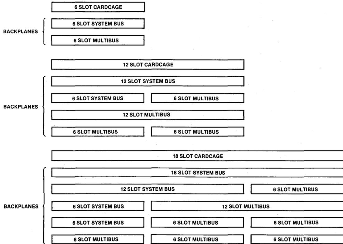
Figure 2-5. Suggested Card Cage and Backplane Combinations
