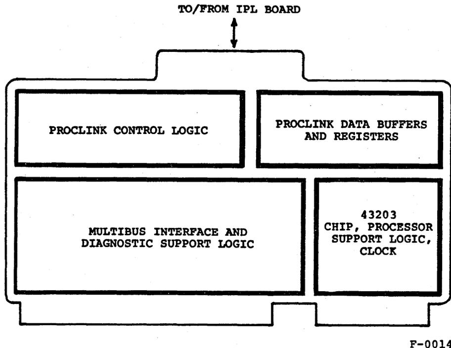
Figure 3-2. Interface Processor Board Block Diagram
