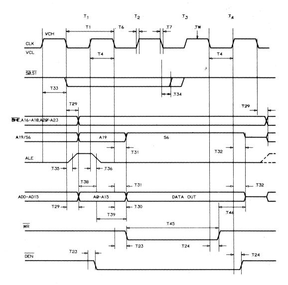
Figure 8.9 shows the Write Cycle timings:
