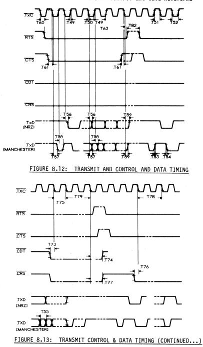
Figure 8.12 and 8.13 show the transmit control and data waveforms
