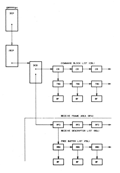
FIGURE 3.1: THE - SHARED -82856/CPU MEMORY STRUCTURE
