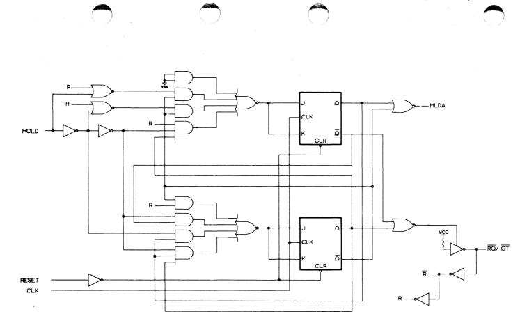
FIGURE 6.3: THE TTL HOLD/HLDA RQ/GT CONVERSION LOGIC
