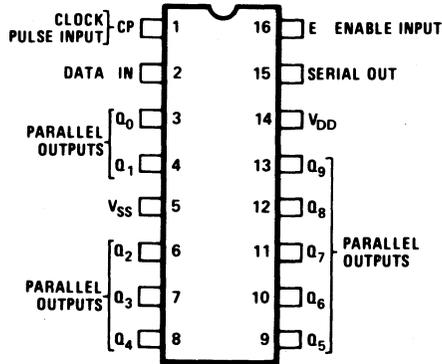
Figure 4-21. 4003 Pin Configuration.
