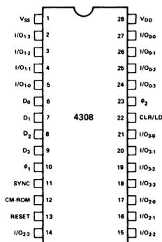
Figure 4-9. 4308 Pin Configuration.
