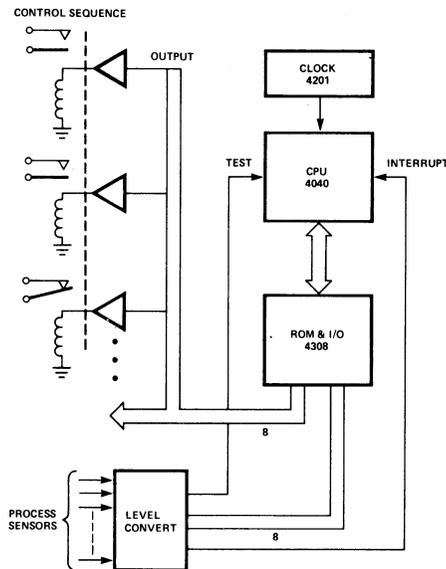
Figure 3-18. Basic Process Controller.
