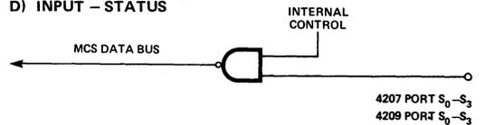
Figure 4-20. 4207, 4209, 4211 Equivalent Circuits.
