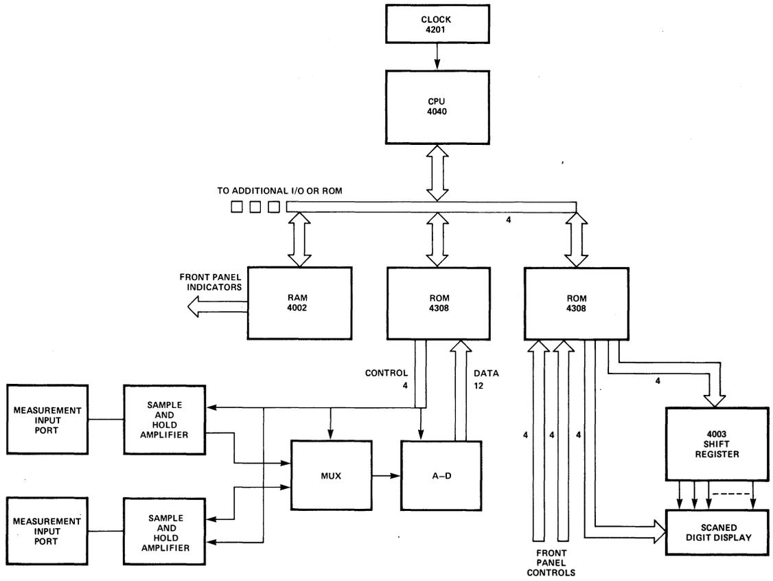
Figure 3-21. Typical A-D Instrument.
