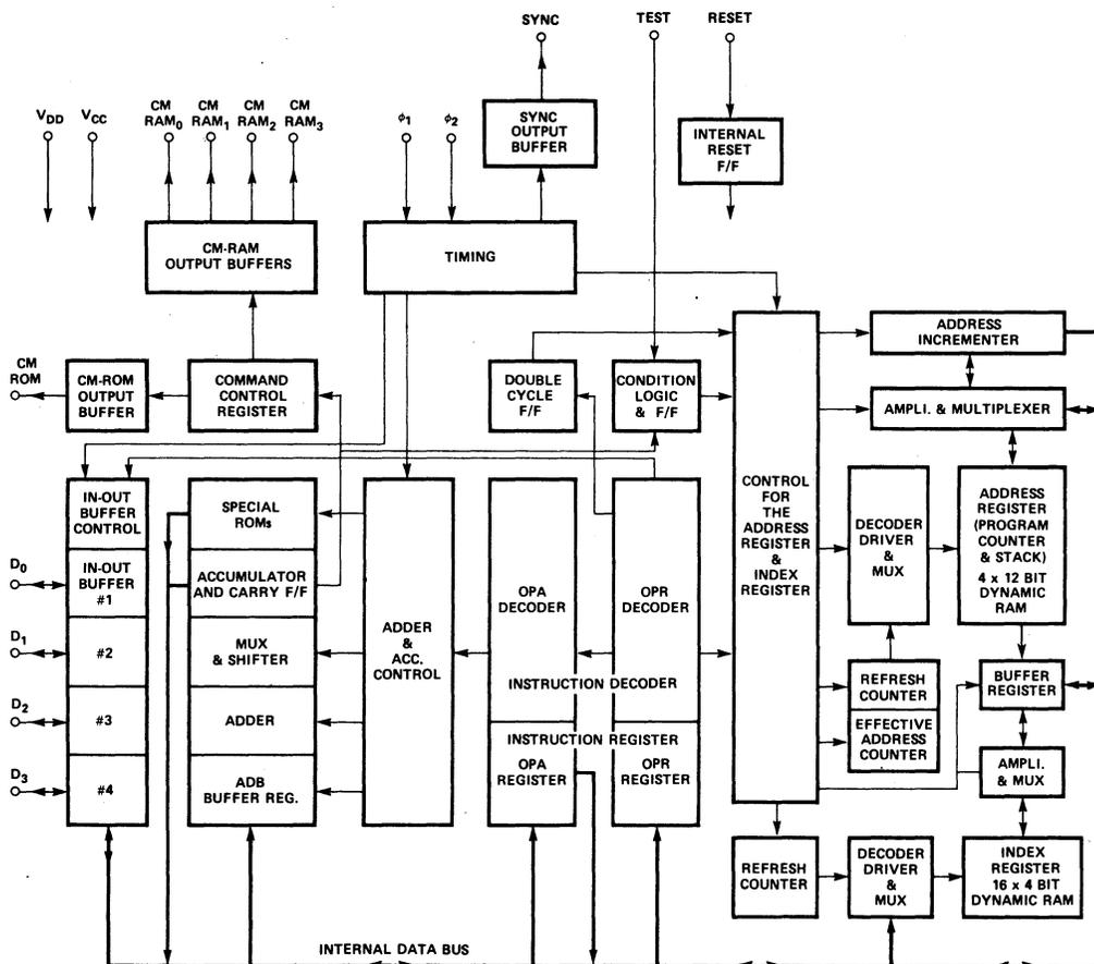
Figure 1-4. 4004 Detailed Block Diagram.
