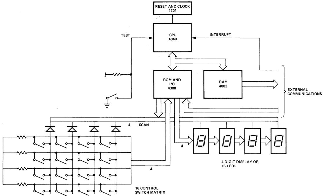
Figure 3-15. Control Panel Encoder with Display.
