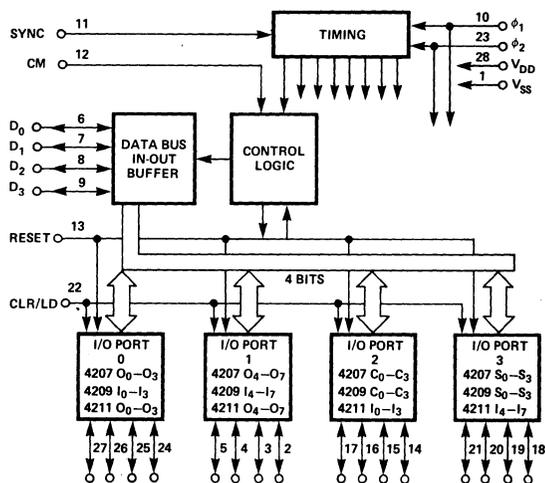
Figure 4-18. 4207, 4209, 4211 Functional Block Diagram.
