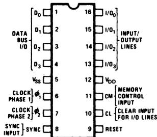
Figure 4-5. 4001 Pin Configuration.
