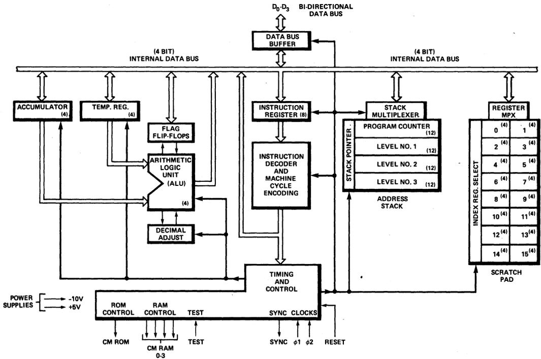
Figure 1-3. 4004 CPU Block Diagram.
