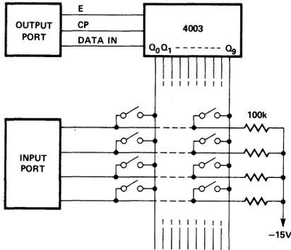
Figure 3-1. Keyboard Interface – (Scanned Array).
