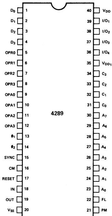
Figure 4-23. 4289 Pin Configuration.
