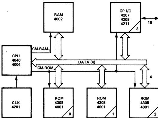
Figure 3-10. Typical System Using GP I/O.
