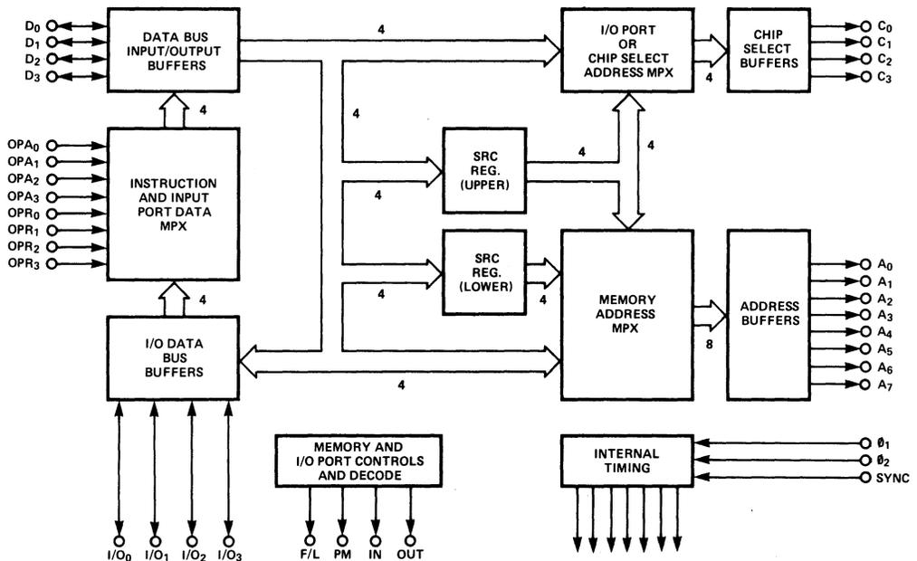
Figure 4-25. 4289 Block Diagram.
