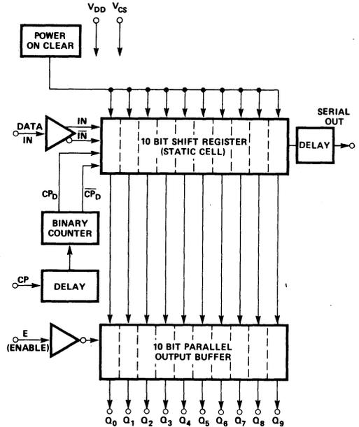
Figure 4-22. 4003 Shift Register Block Diagram.
