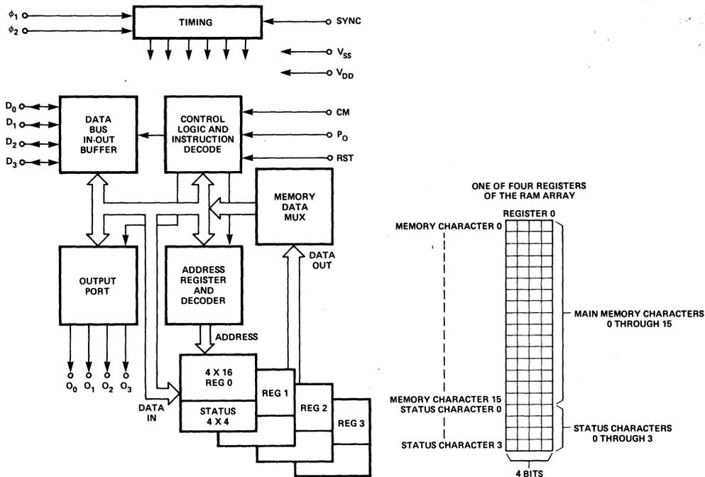
Figure 4-15. 4002 RAM Block Diagram.
