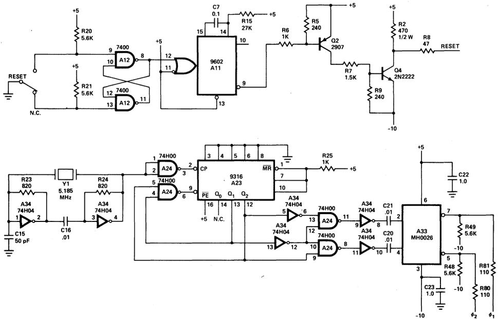
Figure 3-14. Suggested Clock and Reset Circuit.
