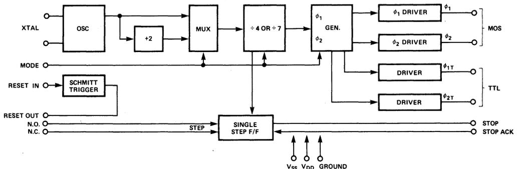
Figure 4-4. 4201 Block Diagram
