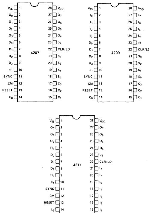
Figure 4-16. 4207, 4209, 4211 Pin Configuration.
