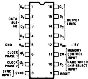
Figure 4-14. 4002 Pin Configuration.
