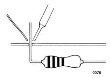
Apply solder from the side opposite the tip, as shown in the illustration. Allow the solder to melt against the lead and pad, then remove both the solder and tip. Only a small amount of solder is needed for a good bond between the lead and pad.
