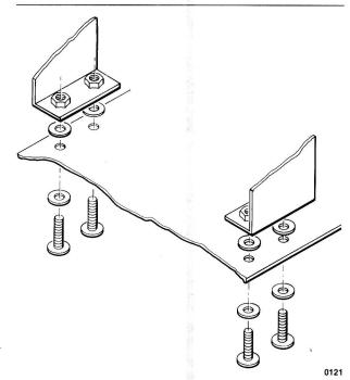
Figure 3-15. Display Board Mounting Bracket Installation
