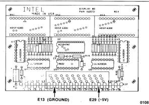
Figure 3-2. Display Board With Check Points
