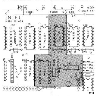
Figure 3-8. Reset Area, Detail
