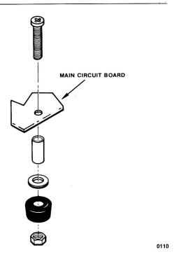
Figure 3-4. Installing Rubber Feet
