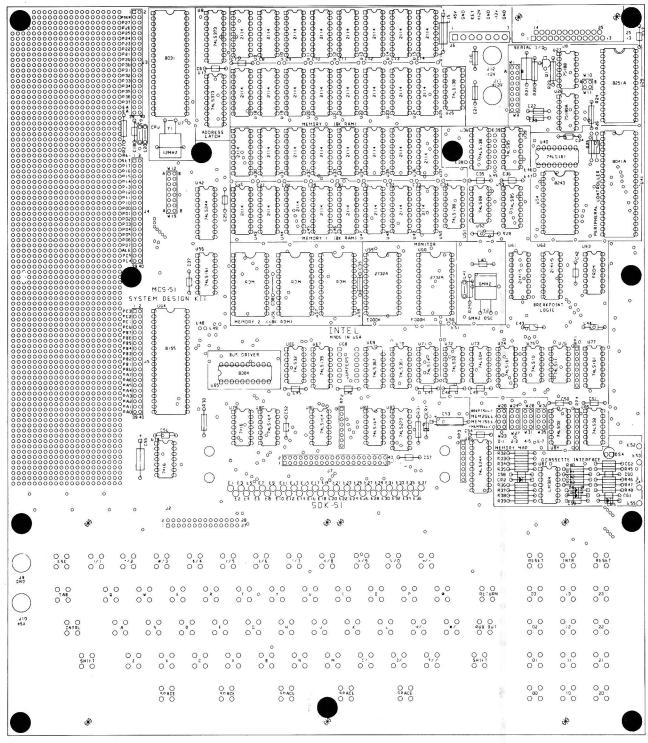
Figure 3-3. Rubber Foot Locations, CPU Board
