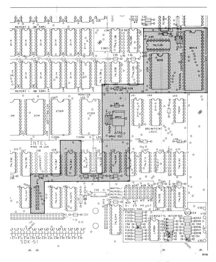
Figure 3-10. 6MHz Timing and UPI Control Areas, Detail
