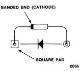
Light-emitting diodes (LEDs) have a flat edge on the cathode side. Install the LED so that the flat edge is toward the square pad.
