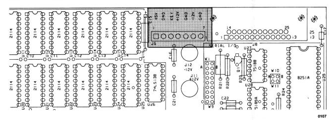
Figure 3-1. Power Connector J6, CPU Board
