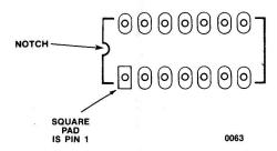
Integrated circuits are manufactured with a notch in the end nearest pin 1. Depending on the manufacturer of the integrated circuit, the notch will look like one of the following:
