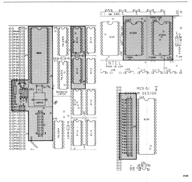
Figure 3-23. Microcontroller, Monitor and RAM Areas, Details
