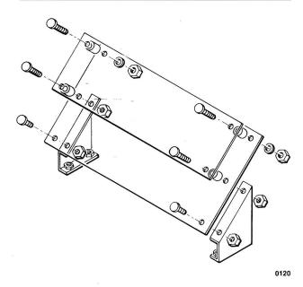
Figure 3-14. Display Board Installation
