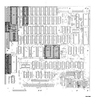
Figure 3-22. Microcontroller, Monitor and RAM Areas
