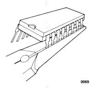
If the integrated circuit still does not fit, bend the pins inward on the other side. After inserting an integrated circuit or resistor pack, carefully check again that:
