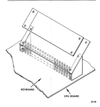
Figure 3-13. Connecting Display Board
