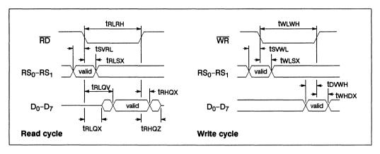
Figure 3.5 Basic read/write cycles
