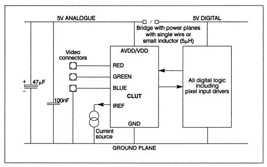
Figure 10.1 Locally decoupling the CLUT supply with an L-C circuit.
