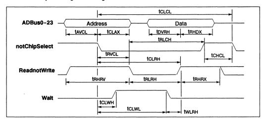
Figure 7.2 Micro port write cycle
