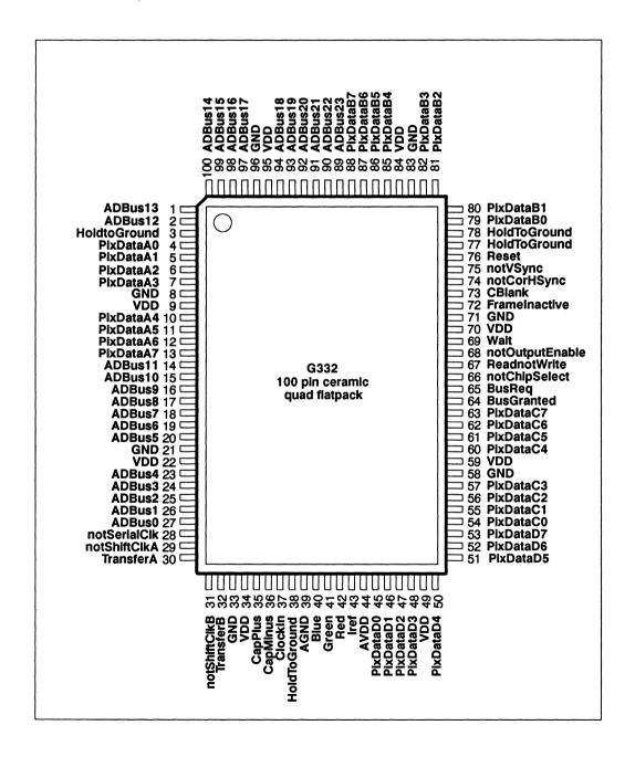
Figure 7.18 IMS G332 pin configuration
