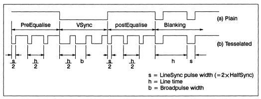
Figure 7.9 Composite Sync frame flyback waveforms
