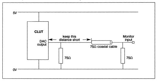
Figure 10.2 Double termination of DAC output.
