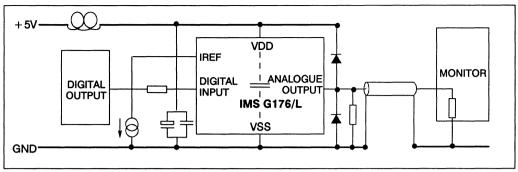
Figure 4.19 Suggested circuit using DIL package
