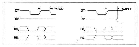
Figure 4.7 Write to pixel mask register followed by any access
