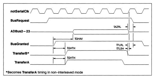
Figure 8.4 Micro port DMA and data transfer timings
