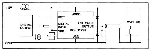
Figure 5.18 Suggested circuit using PLCC package
