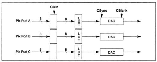
Figure 6.26 Pixel port in mode 2
