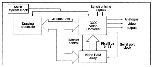
Figure 6.2 IMS G300 operating in a simple graphics system
