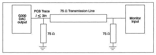
Figure 6.29 DAC output loading
