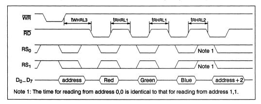
Figure 4.14 Read colour value then the address register (read mode)
