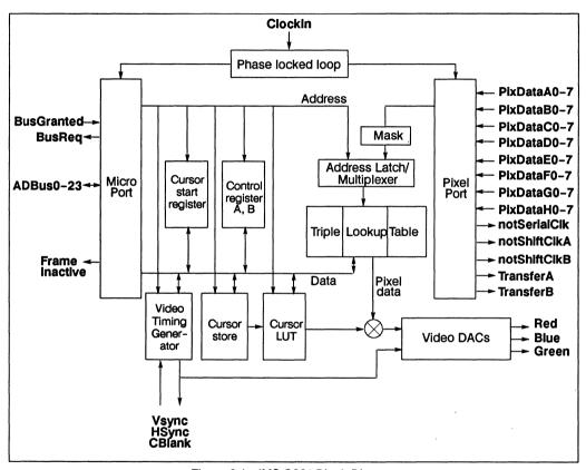
Figure 8.1 IMS G364 Block Diagram
