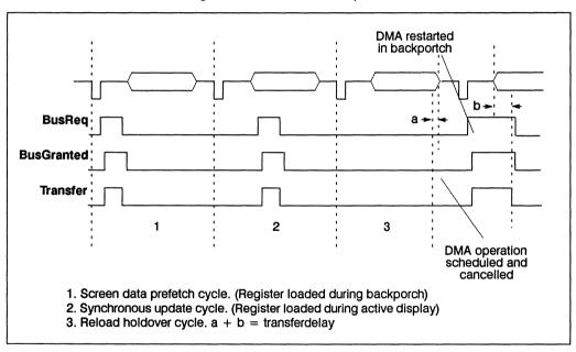
Figure 6.21 Data transfer operational behaviour
