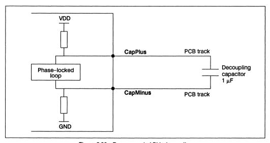
Figure 6.30 Recommended PLL decoupling
