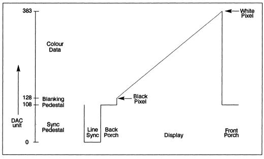
Figure 7.15 DAC output levels
