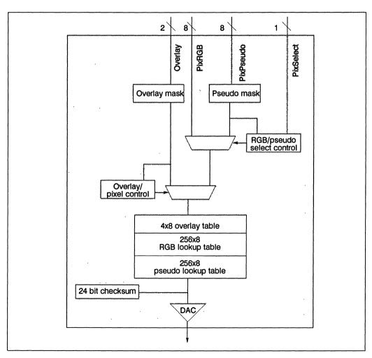
Figure 9.1 Colour Channel Architecture
