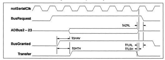
Figure 6.5 Micro port DMA and data transfer timings
