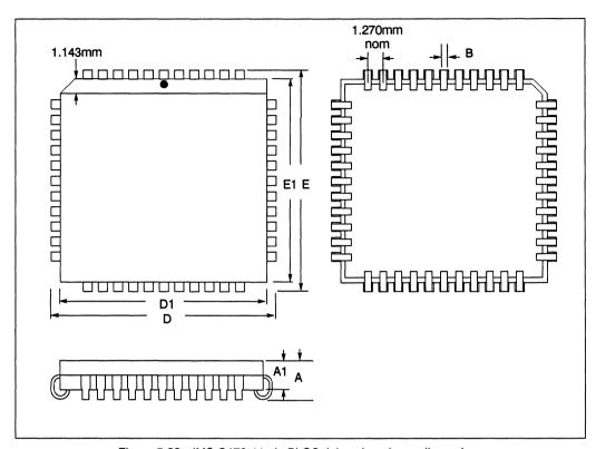
Figure 5.22 IMS G178 44 pin PLCC J-bend package dimensions
