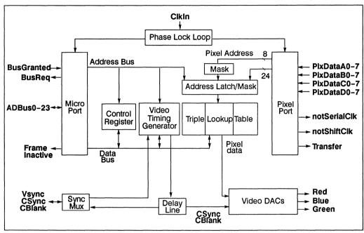
Figure 6.1 IMS G300 Block Diagram
