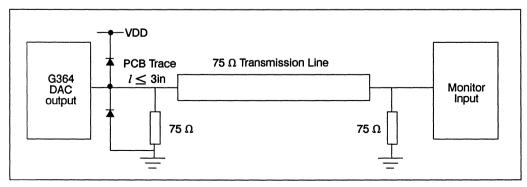
Figure 8.17 DAC output loading
