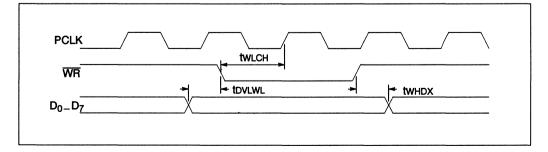
Figure 3.19 Pixel mask register synchronisation.
