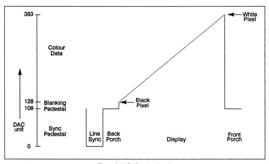
Figure 8.15 DAC output levels
