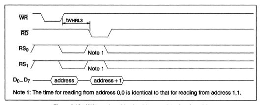
Figure 5.13 Write and read back address register (read mode)
