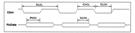
Figure 6.8 Pixel port signals in mode 2
