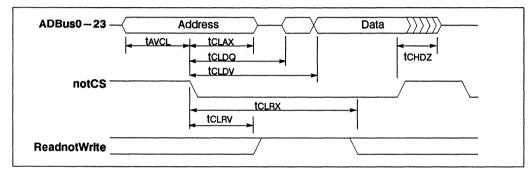
Figure 6.4 Micro port read cycle
