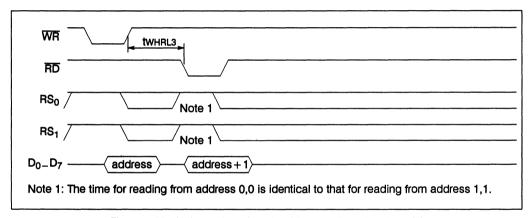
Figure 4.13 Write and read back address register (read mode)
