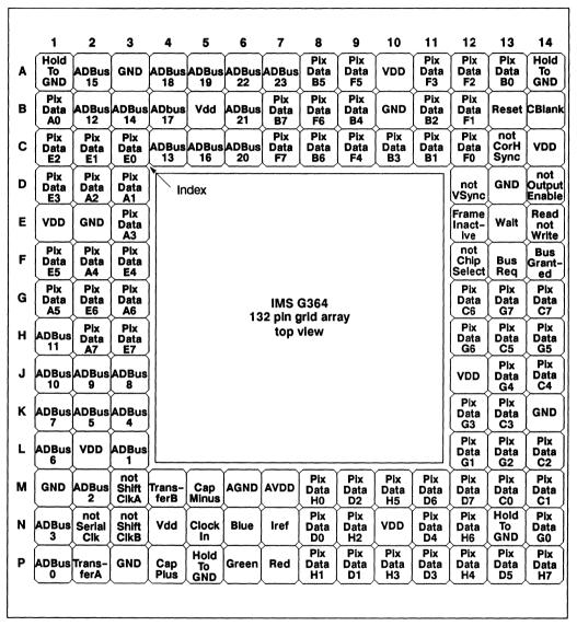
Figure 8.18 IMS G364 pin configuration
