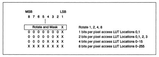
Figure 6.23 Colour palette programming information in 1, 2 and 4 bits per pixel modes
