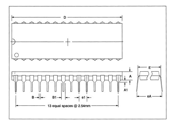
Figure 3.21 28 pin plastic dual-in-line package dimensions
