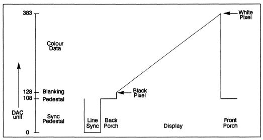
Figure 6.27 DAC output levels
