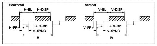
Figure 6.36 Hitachi HM-42/4119 timing
