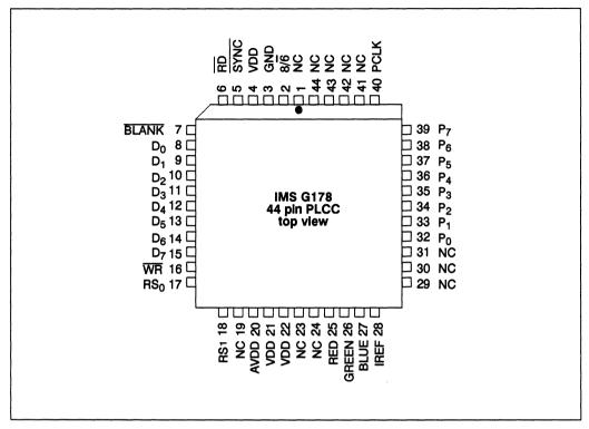
Figure 5.21 IMS G178 44 pin PLCC J-bend package pinout
