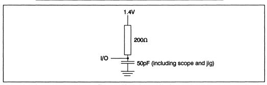
Figure 4.3Digital output load
