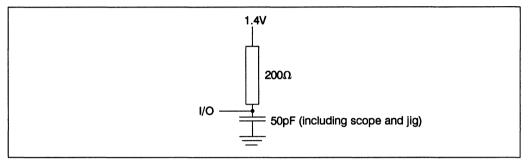
Figure 5.3 Digital output load
