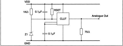
Figure 10.8 Voltage reference circuit
