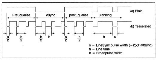
Figure 8.9 Composite Sync frame flyback waveforms
