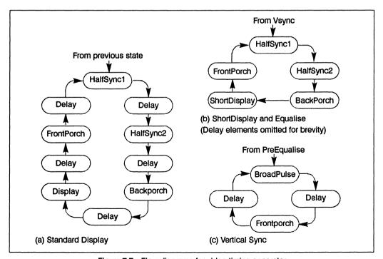
Figure 7.7 Flow diagrams for video timing generator
