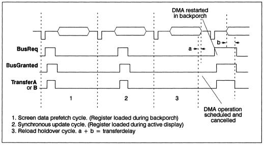
Figure 7.12 Data transfer operational behaviour
