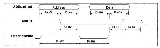
Figure 6.3 Micro port write cycle
