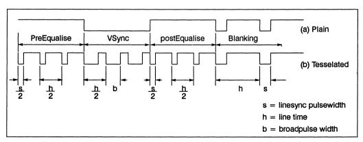
Figure 6.15 Composite Sync frame flyback waveforms
