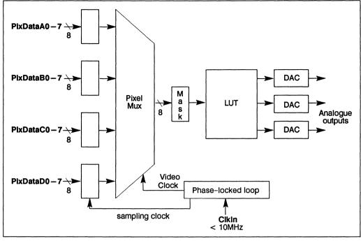
Figure 6.25 Pixel port in mode 1
