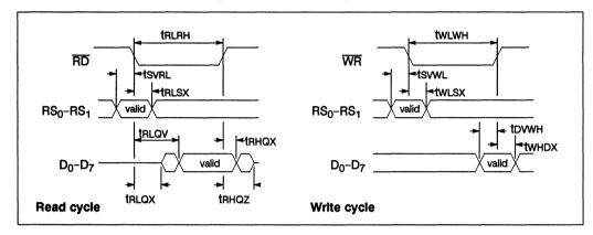
Figure 5.6 Basic read/write cycles
