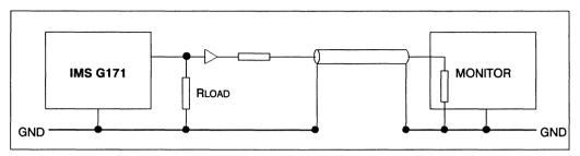
Figure 3.15 Buffered signal
