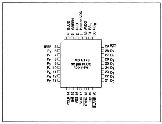
Figure 5.19 IMS G178 32 pin PLCC J-bend package pinout
