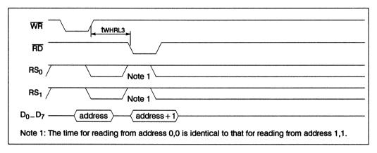
Figure 3.12 Write and read back address register (read mode)
