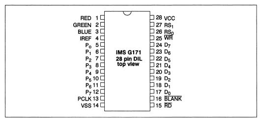
Figure 3.20 IMS G171 28 pin dual-in line package pinout
