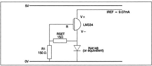
Figure 10.6 Current reference based on the LM334.
