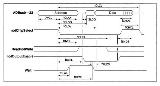
Figure 8.3 Micro port read cycle
