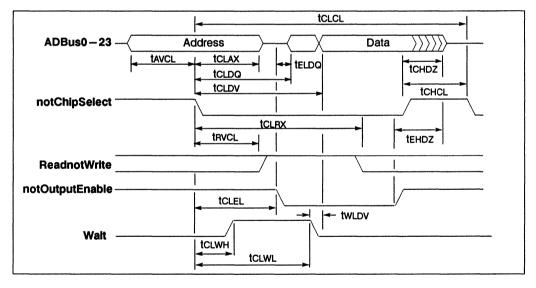
Figure 7.3 Micro port read cycle
