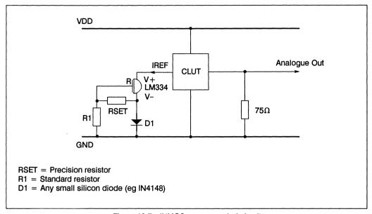
Figure 10.7 INMOS recommended circuit
