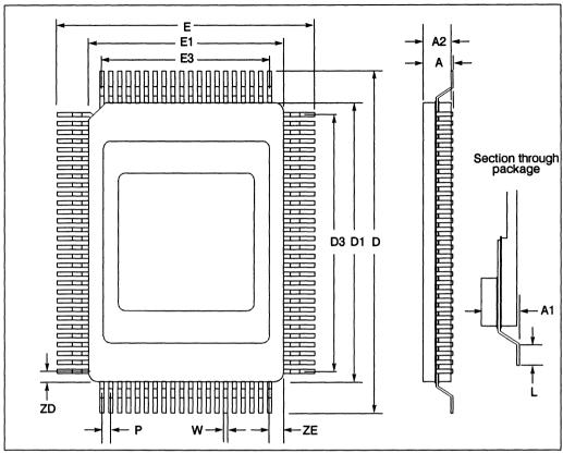
Figure 7.19 100 pin ceramic quad flatpack package dimensions
