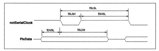
Figure 8.5 Pixel port timing diagram
