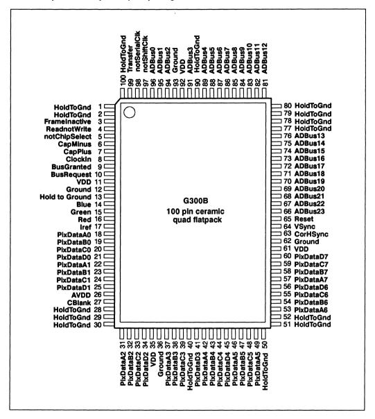
Figure 6.34 IMS G300 pin configuration
