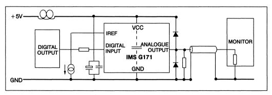
Figure 3.17 Circuit incorporating suggested design features
