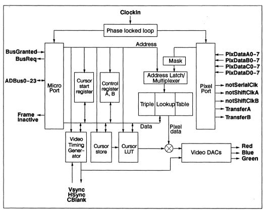
Figure 7.1 IMS G332 Block Diagram
