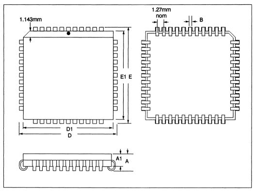
Figure 4.25 IMS G176 44 pin PLCC J-bend package dimensions
