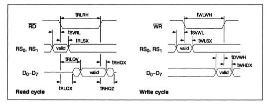
Figure 4.6 Basic read/write cycles
