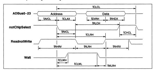
Figure 8.2 Micro port write cycle
