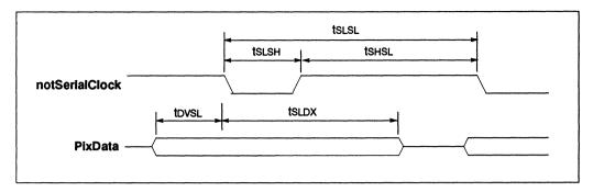
Figure 7.5 Pixel port timing diagram
