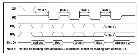
Figure 3.13 Read colour value then the address register (read mode)
