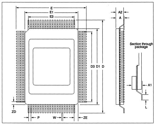
Figure 6.35 100 pin ceramic quad flatpack package dimensions
