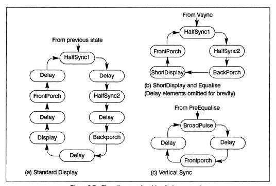
Figure 8.7 Flow diagrams for video timing generator
