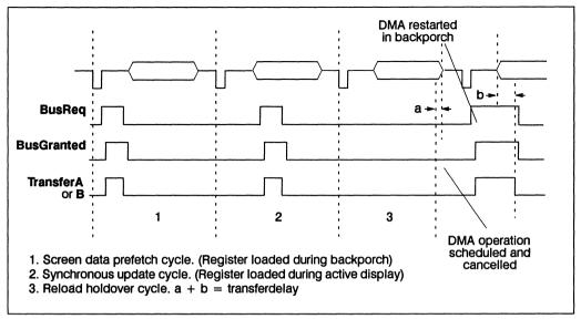
Figure 8.12 Data transfer operational behaviour
