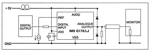
Figure 4.18 Suggested circuit using PLCC package
