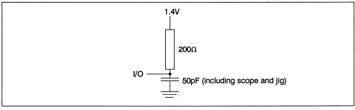
Figure 3.3 Digital output load
