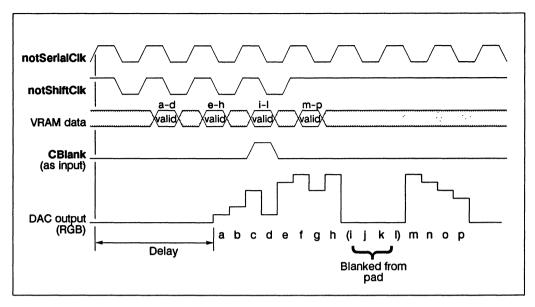
Figure 6.19 Delay between notShiftClk and DAC outputs in mode 1
