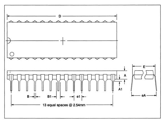
Figure 4.21 28 pin plastic dual-in-line package dimensions
