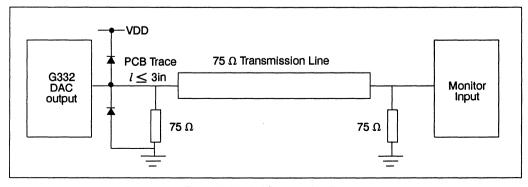
Figure 7.17 DAC output loading
