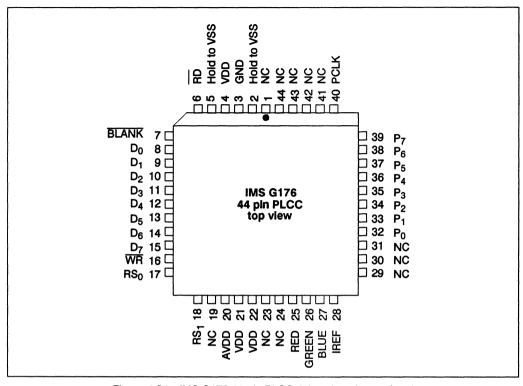
Figure 4.24 IMS G176 44 pin PLCC J-bend package pinout
