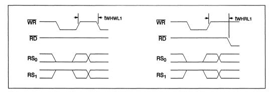
Figure 5.7 Write to pixel mask register followed by any access
