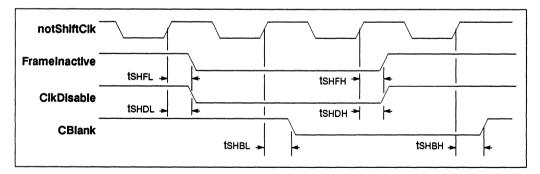
Figure 6.9 Relationship between notShiftClk, FrameInactive, ClkDisable and CBlank
