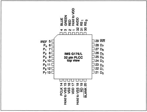
Figure 4.22 IMS G176/L 32 pin PLCC J-bend package pinout
