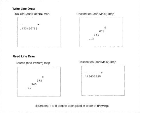
Figure 4.19 Memory to memory Line Draw address stepping.
