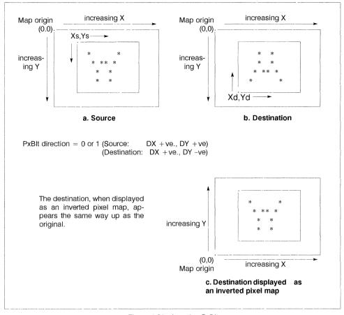
Figure 4.21 Inverting PxBlt
