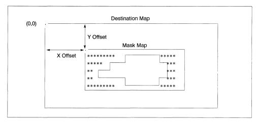
Figure 4.10 Mask Map Origin X and Y Offsets
