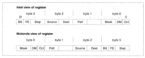
Figure 4.24 Pixel Operation Register fields
