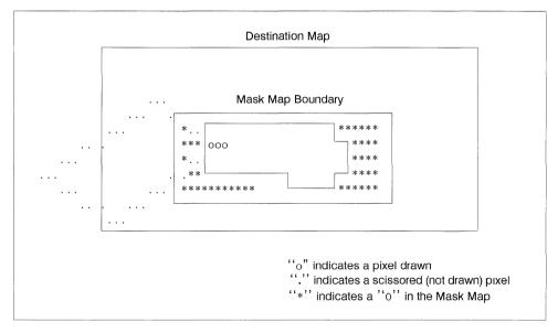
Figure 4.13 Mask Map Enabled Scissor
