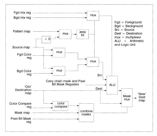
Figure 4.6 Coprocessor data flow.
