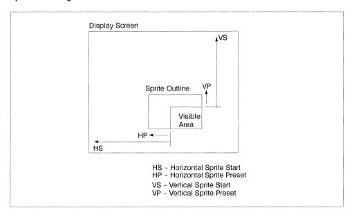
Figure 4.3 Sprite Positioning
