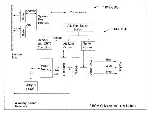
Figure 1.1 XGA Function Block Diagram
