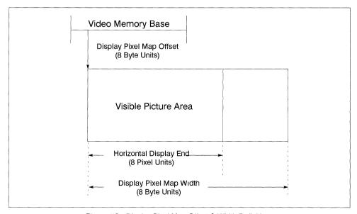
Figure 4.2 Display Pixel Map Offset & Width Definitions
