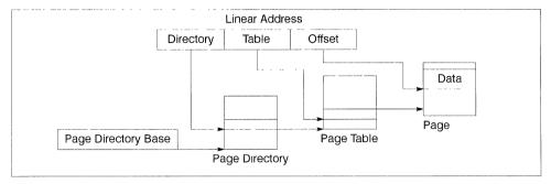
Figure 5.3 Linear to Physical Address Translation
