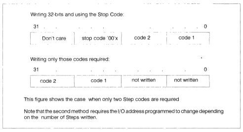
Figure 4.17 Programming less than four Step codes
