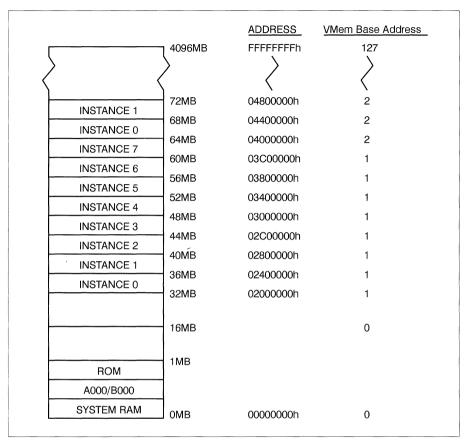
Figure 7.2 The XGA Video Memory Base Address Diagram
