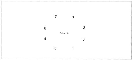
Figure 4 18 Bresenham Line Draw Octant encoding
