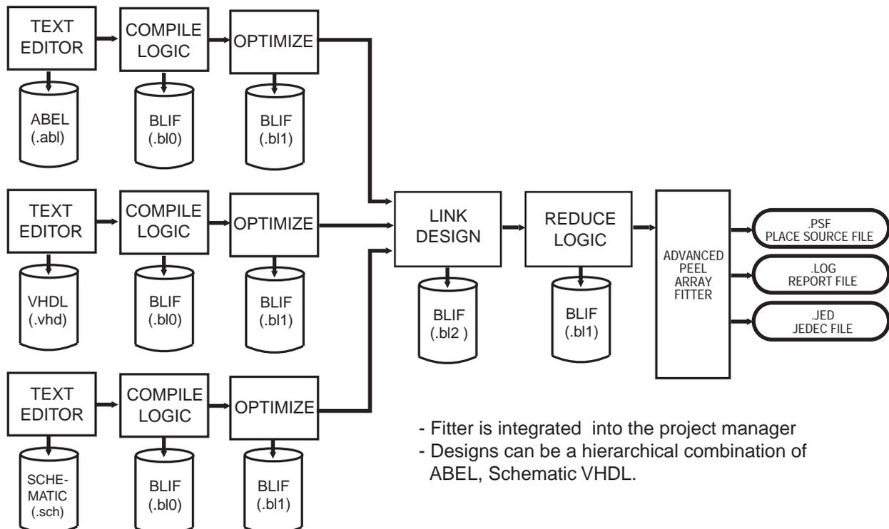
Figure 1. Flow diagram for Synario
