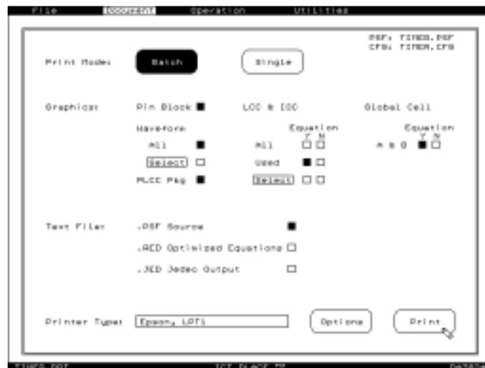
Figure 6. PLACE designs can be documented through batch or single printing of architectural configurations, waveform displays and logic descriptions including equations, state-diagrams, and truth-tables.
