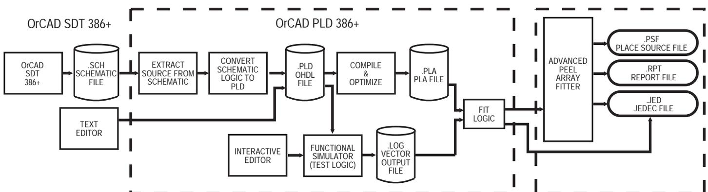
Figure 1. OrCAD design process for PEEL Arrays
