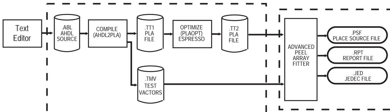
Figure 1. Design flow with the ABEL-to-PEEL Advanced Fitter
