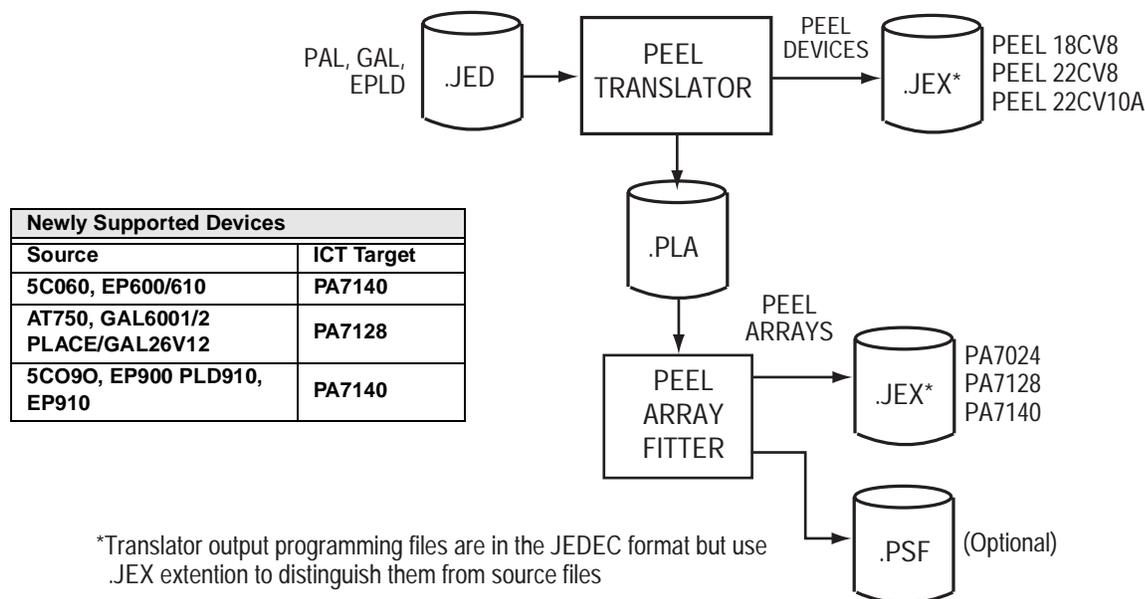
Figure 1. PEEL Translator Design Flow
