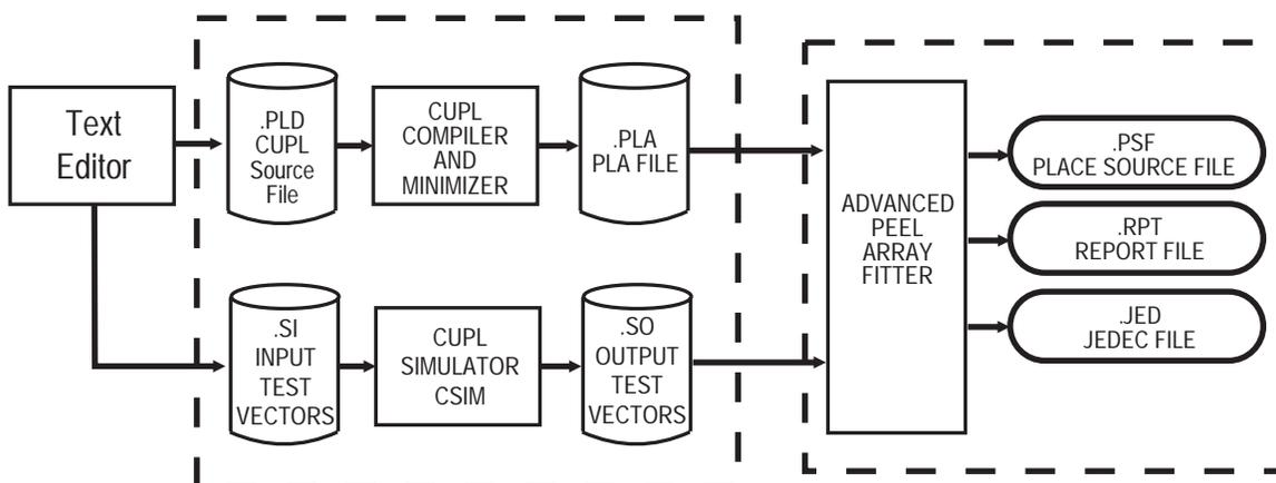
Figure 1. Design Flow for the CUPL-to-PEEL Advanced Fitter
