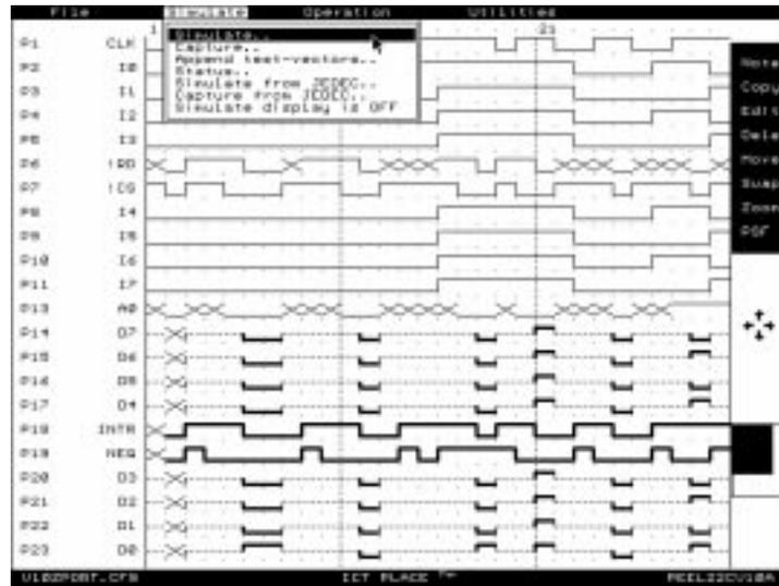
Figure 5. The PLACE logic simulator lets external and internal signals be fully simulated, analyzed and edited via a special waveform display. Output signals can be “captured” or simulated. Simulation errors are marked on the display for quick analysis.
