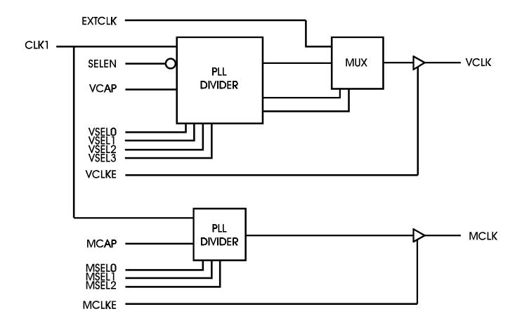
Figure 2-2 ICS90C64A Functional Block Diagram
