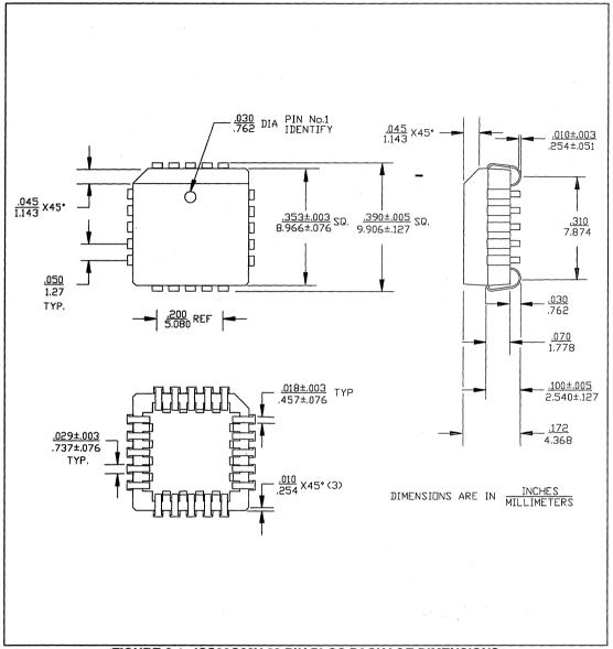
FIGURE 6-1. ICS90C63V 20-PIN PLCC PACKAGE DIMENSIONS
