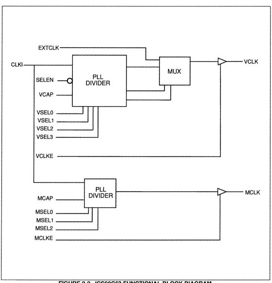
FIGURE 2-2. ICS90C63 FUNCTIONAL BLOCK DIAGRAM
