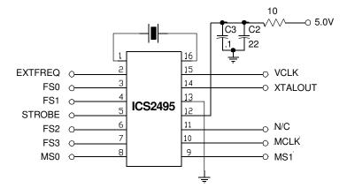
**NOTES:** FS3-FS0, MS1-MS0, EXTFREQ, and STROBE inputs are all equipped with pull-ups and need not be tied high. Mount decoupling capacitors as close as possible to the device and connect device ground to the ground plane where available. Mount crystal and its circuit traces away from switching digital lines and the VCLK, MCLK and XTALOUT lines.
