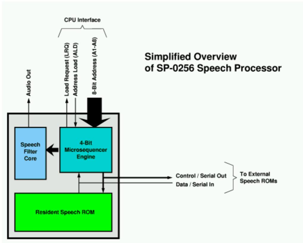
The digital filter contains all of the pieces necessary to generate the actual speech sounds. The impulse generator and IIR filter model the vocal tract by shaping the periodic impulses in a similar manner to how the human vocal tract shapes sound. This core operates largely independently of the microsequencer, except that it relies on the microsequencer to receive parameter updates, and it notifies the microsequencer when it completes an utterance.
