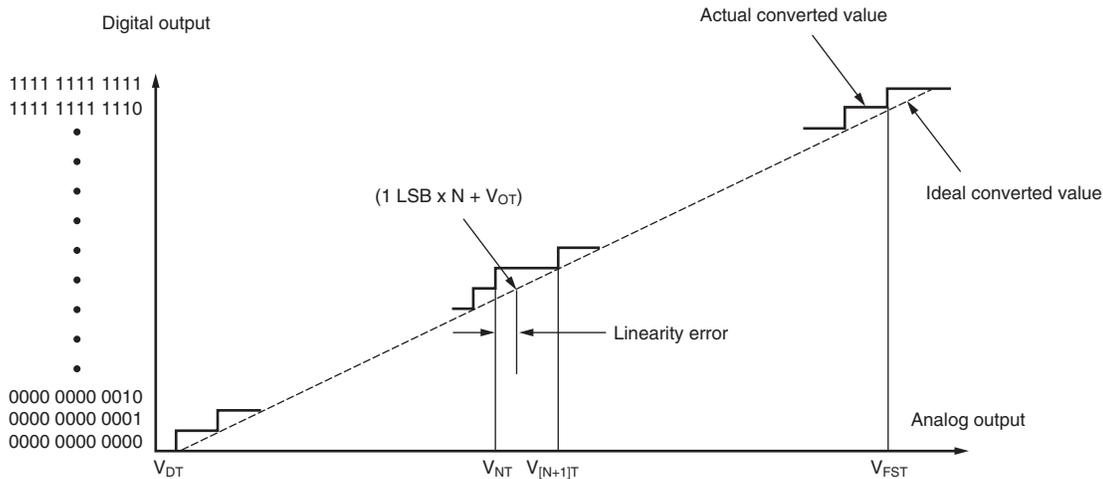
**Differential linearity Error:** The deviation of input voltage needed to change the output code by one LSB from the theoretical value.
