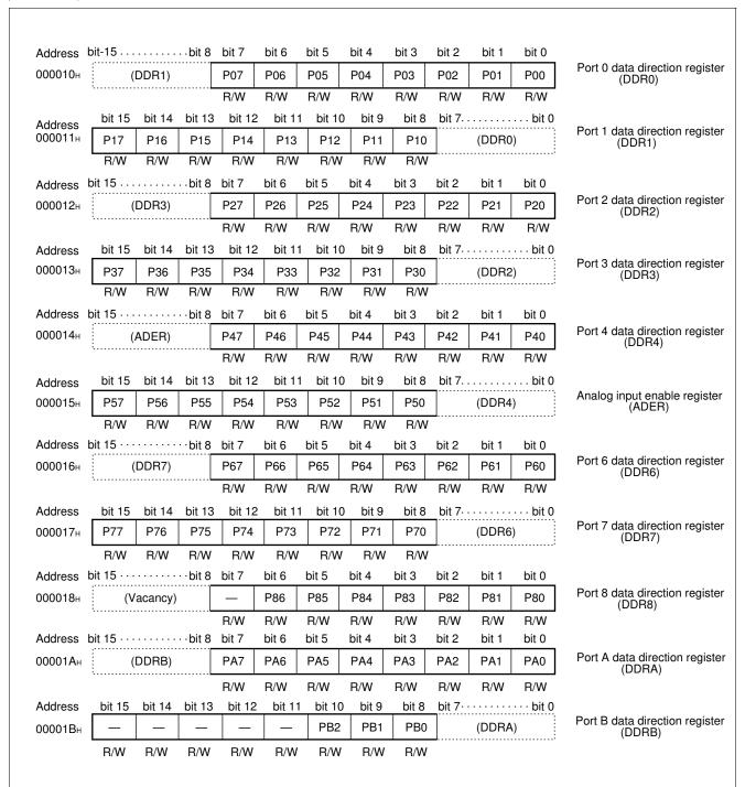
Note: Only MB90675 series has P81 through P86, P90, PA0 through PA7, and PB0 through PB2, and MB90670 series does not have such pins.
