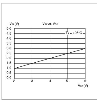
(3) "H" Level Input Voltage/"L" Level Input Voltage (4) "H" Level Input Voltage/"L" Level Input Voltage (Hysteresis Input)
