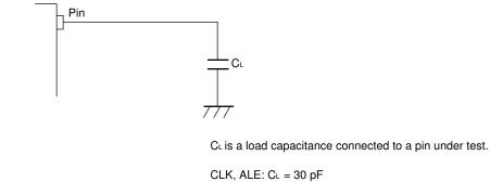
Address data bus (AD15 to AD00),  $\overline{RD}$ ,  $\overline{WR}$ :  $C_L = 80 \text{ pF}$
